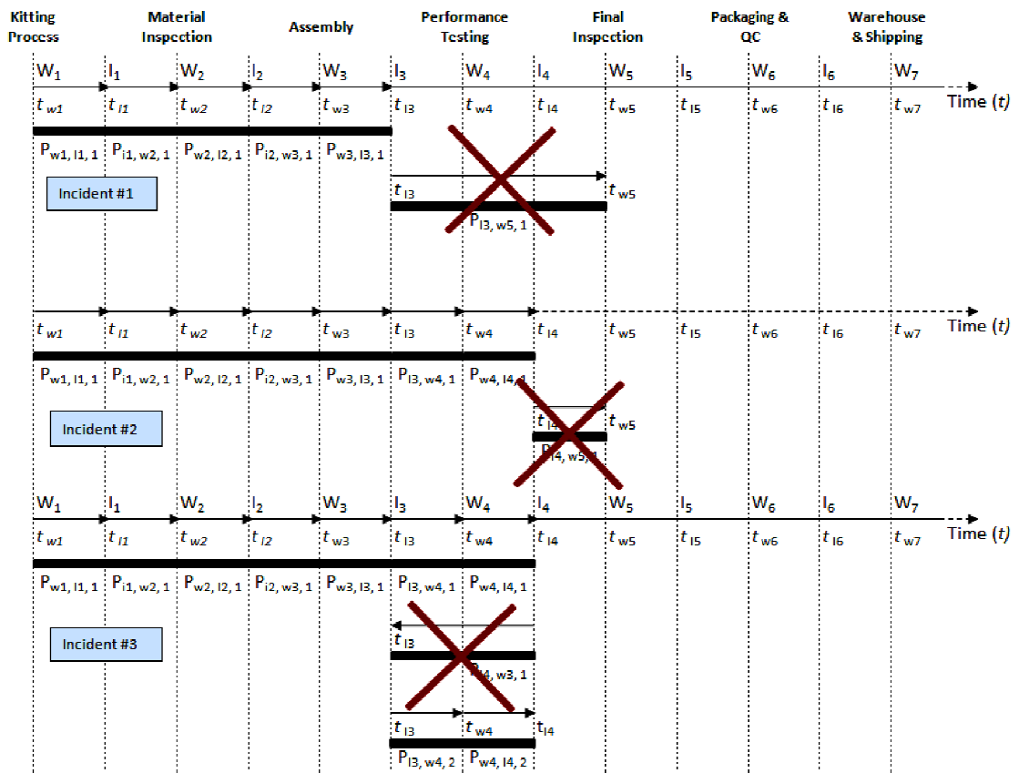
Figure 15: Unexpected Incidents and RFID-based Traceability System
