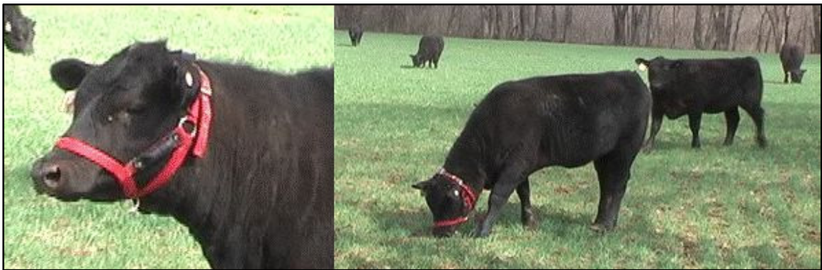
Figure 1. Heifer fitted with instrumented test halter grazing in an open range wheat pasture. Halter style is standard nylon turn-out, and is equipped with micro-GPS and grazing activity wireless sensor (915 MHz carrier frequency).
