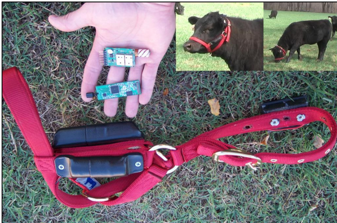
Figure 12. Standard nylon turnout halter equipped with custom enclosures. Custom wireless sensor and miniature GPS module are shown.
