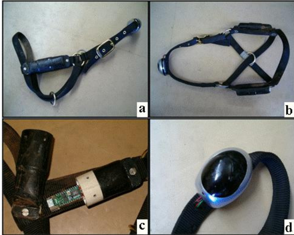
Figure 17. Instrumented proof-of-concept halter. a) Side view of test halter, b) top view, c) accelerometer data logging device, and d) GPS logging device
