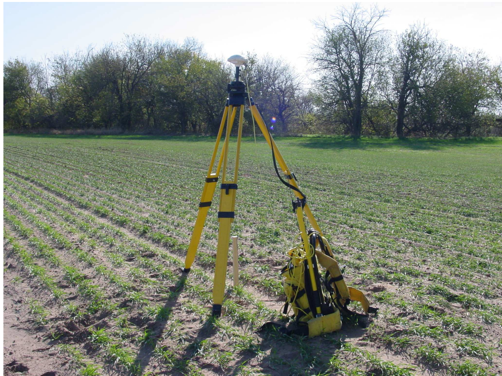
Figure 2-2 Control points set-up
