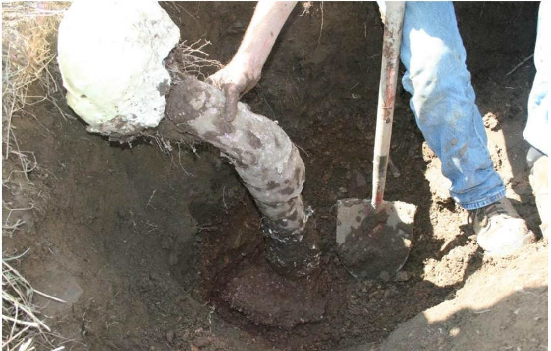
Figure 7.12. Large macropore at the Barren Fork Creek site observed during plot scale infiltration experiment (a) and subsequently filled with expandable foam and excavated (b).
