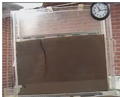
Figure 1.3 Examples of undercutting by seepage particle mobilization, tension crack formation, and bank collapse observed during the lysimeter experiments.
