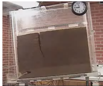
Figure 1.3 Examples of undercutting by seepage particle mobilization, tension crack formation, and bank collapse observed during the lysimeter experiments.
