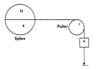
Diagram shows the mass connected by a string to both sphere and pulley. The mass will descend a distance h.
