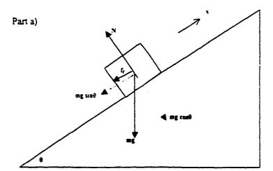
Diagram shows initial conditions Dotted lines show resolution of the weight, mg, into components mg sin0 and mg cos 0. The force of friction acts against upward motion.. Force due to frictian,  $f_f$ is parallel to the incline and its direction is opposed to motion. The normal force is shown by N. The x-direction is parallel to the incline.
