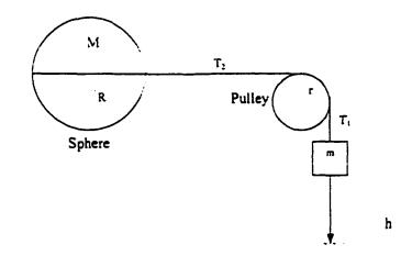
Diagram shows the mass connected by a string to both sphere and pulley. The mass will descend a distance h.
