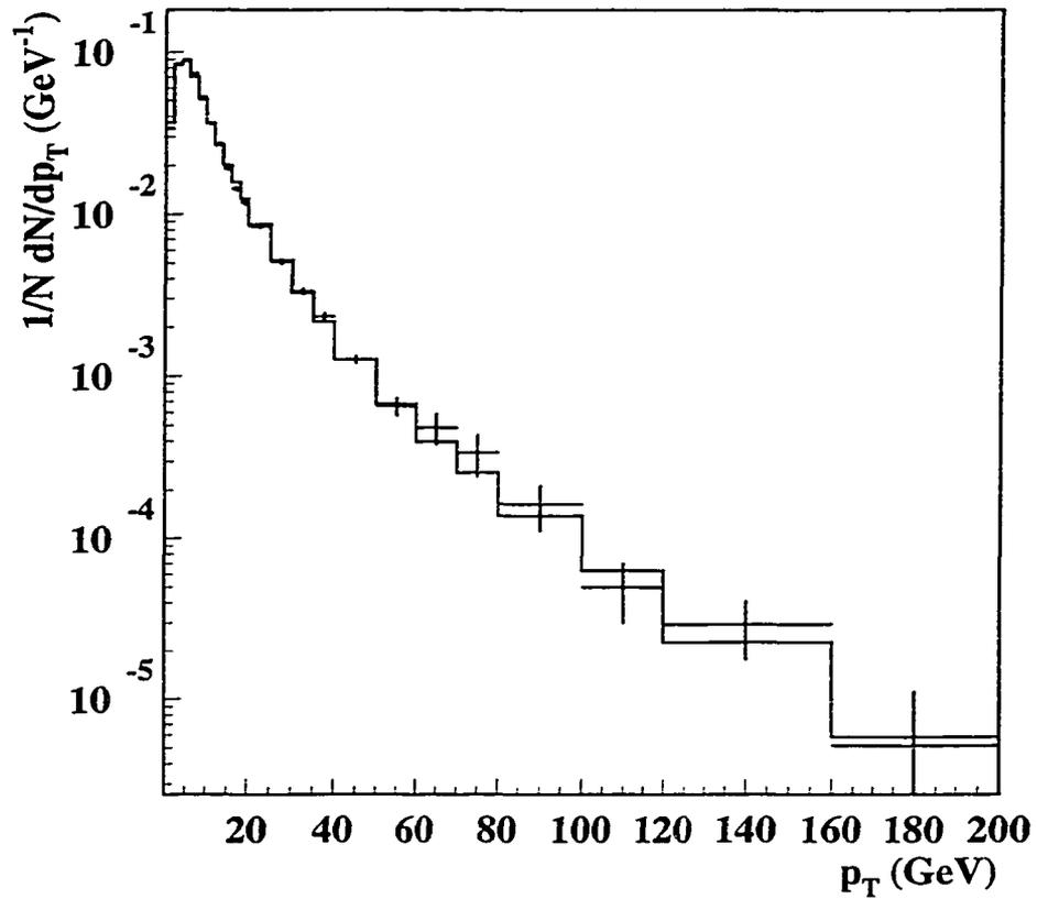
Figure 5.36: Background subtracted transverse momentum distribution for  $W \rightarrow e\nu$  events (points with statistical errors) and smeared theory (solid histogram).
