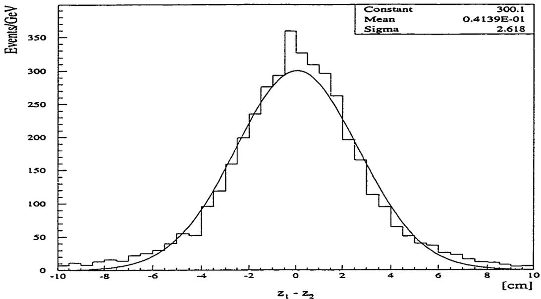
Figure 4.10: Distribution of  $(z_1 - z_2)$  for  $Z \rightarrow ee$  events.
