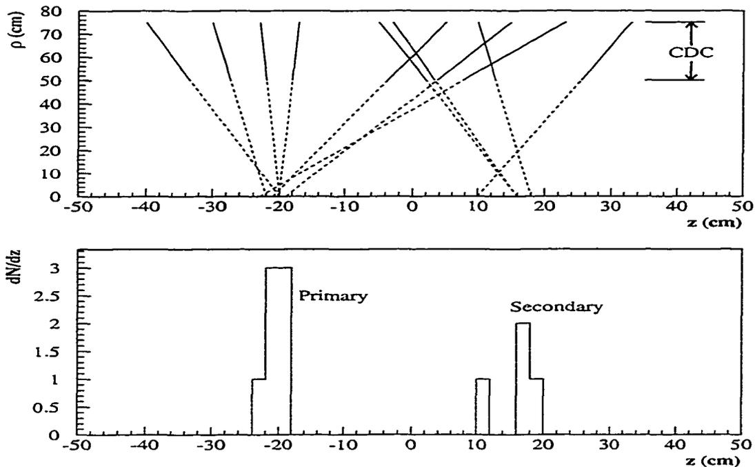
Figure 4.1: Vertex  $z$  coordinate finding by the histogram method as used by DØRECO. The upper plot shows CDC tracks projected onto the beamline (for all  $\phi$ ). The lower plot shows the corresponding  $z$ -intercept distribution.
