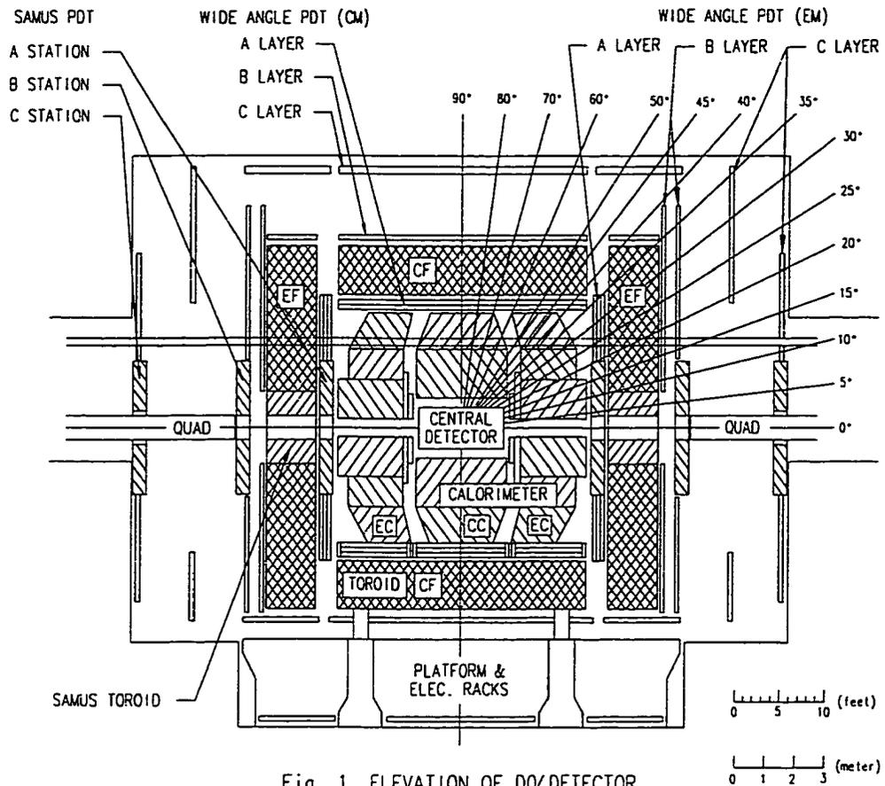
Fig. 1 ELEVATION OF DØ/DETECTOR
