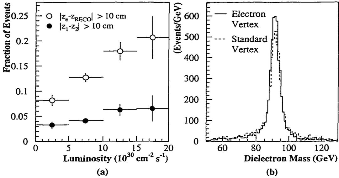
Figure 4.11: (a) Frequency at which the RECO vertex is mismeasured as a function of instantaneous luminosity. To be compared to the frequency at which the vertices obtained by projecting the two electrons into the beamline are more than 10 cm apart. (b) Invariant mass distributions for  $Z \rightarrow ee$  events for the two vertex methods.
