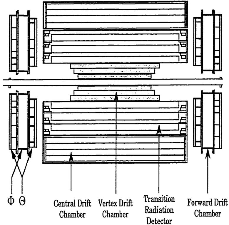
Figure 3.3: Side view of the central tracking system.
