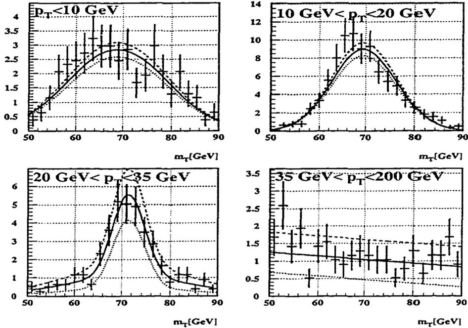
Figure 5.31:  $Z$  background as a function of transverse mass in four  $p_T$  bins. The curves shown are the fits and overall  $Z$  background errors.
