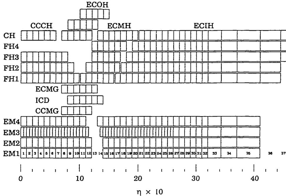
Figure 3.10: Segmentation of the  $D\emptyset$  calorimeter towers.
