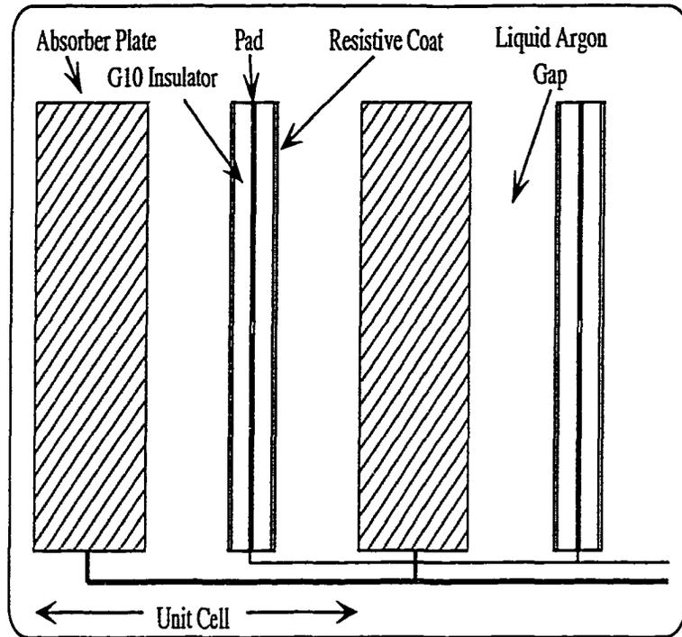
Figure 3.9: Two unit cells of the DØ calorimeter.
