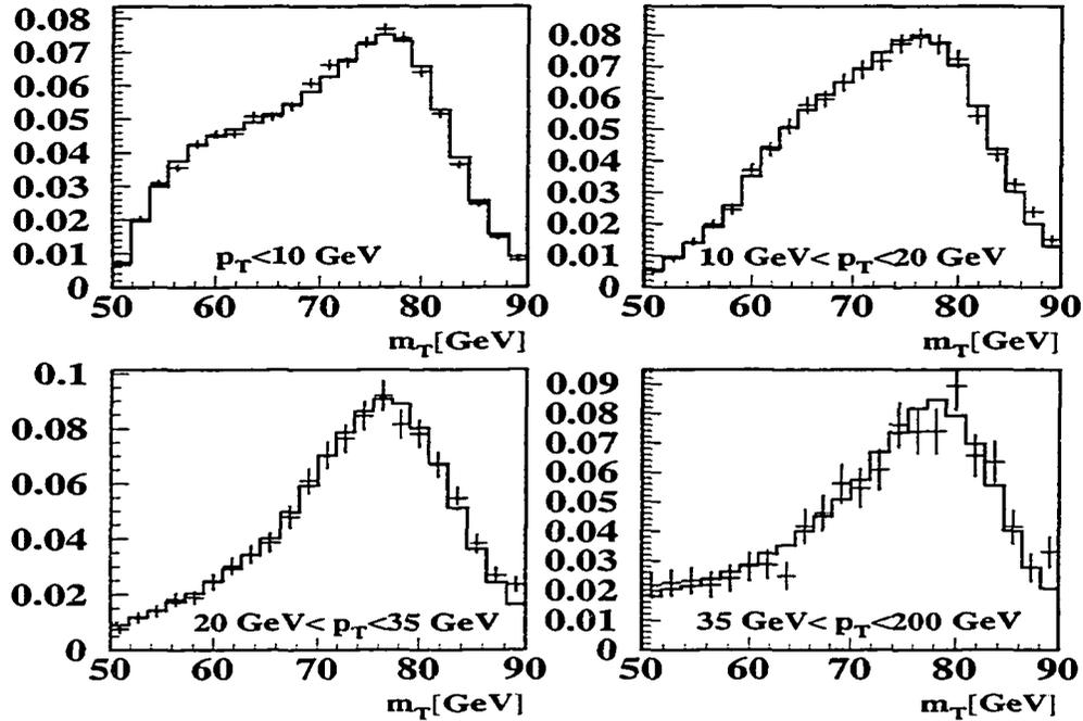
Figure 5.39: Background subtracted transverse mass distribution in four  $p_T$  bins compared to CMS.
