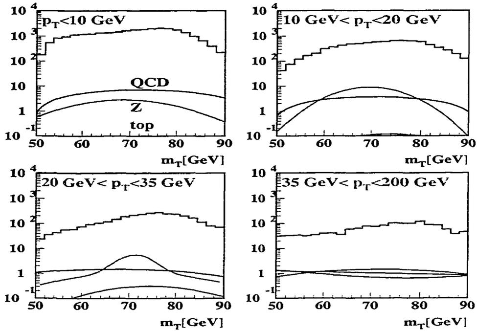
Figure 5.35: Transverse mass spectrum for  $W \rightarrow e\nu$  candidate events and QCD (black), Z (light grey), and  $t\bar{t}$  backgrounds (darker grey) in four  $p_T$  bins.
