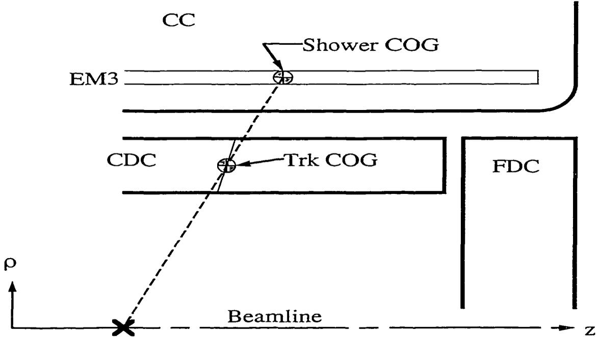
Figure 4.9: Vertex position finding by cluster-track projection method.
