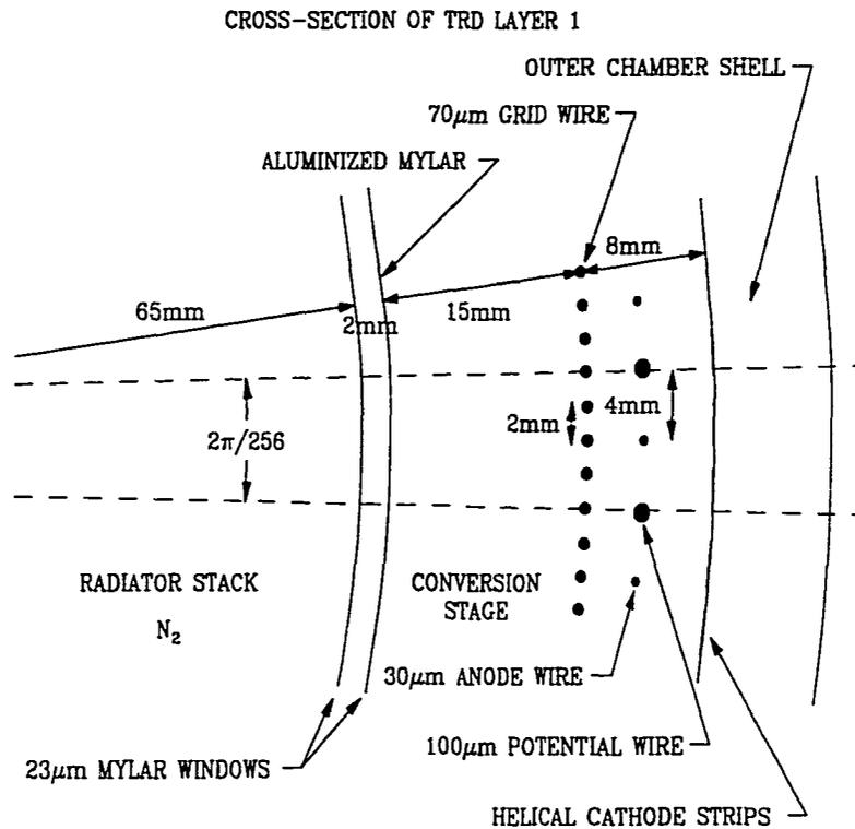
Figure 3.4: The Transition Radiation Detector.
