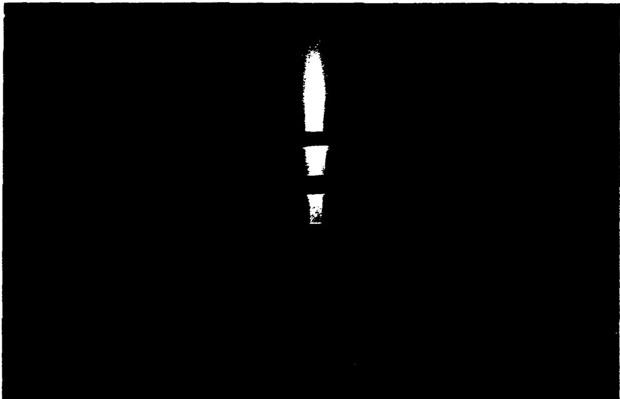
**Fig. 4.1b: Photograph of the cascaded gas jet flame at  $Re=5100$ .**
