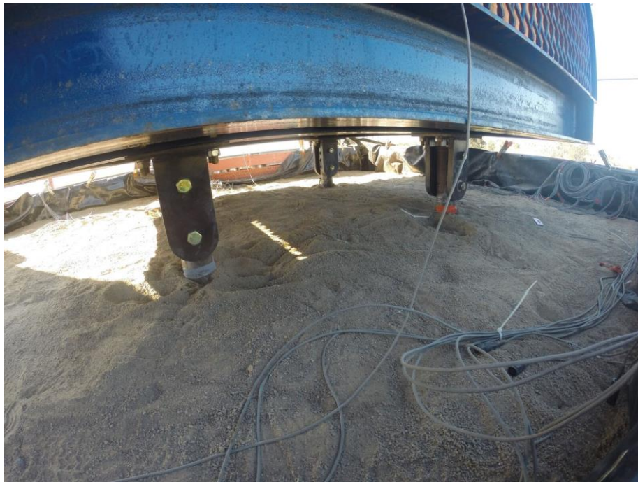
Figure 20: Illustration of Fixed Connection (Double Bolt)
