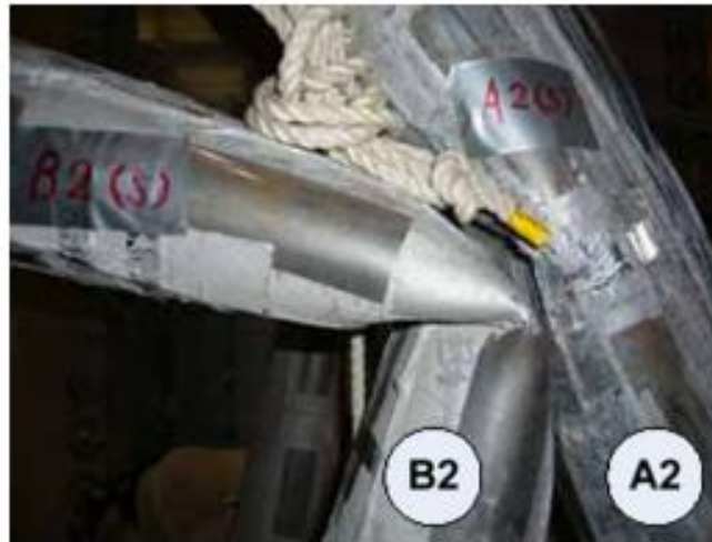
Figure 3: Plastic Hinge Formation in Test Piles (Motamed et al. 2013)
