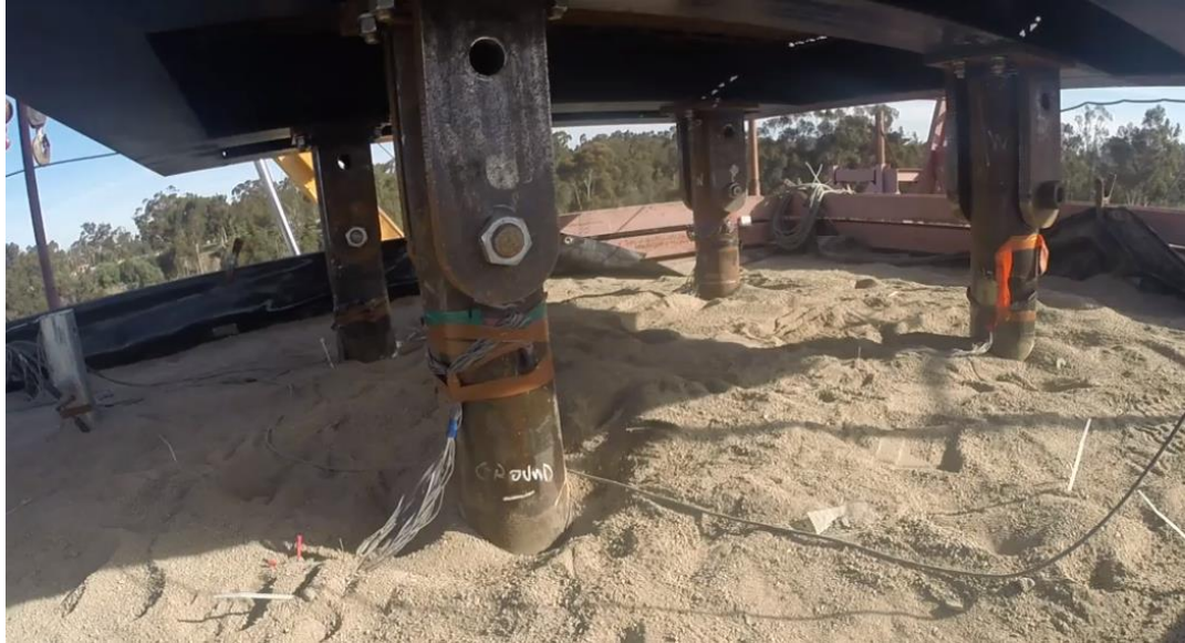
Figure 21: Illustration of Pinned Connection (Single Bolt)
