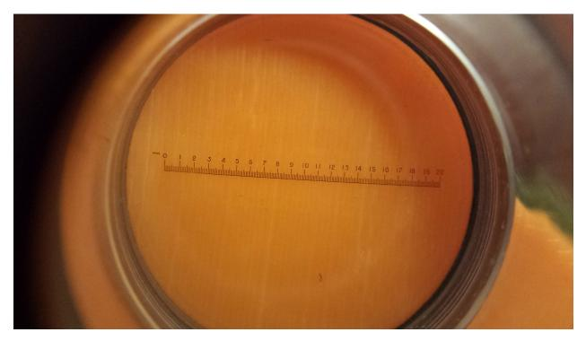
Figure 5.38: Flat mounting surface of part printed on MakerBot 2 on 3D printed part surfaces under 10x magnification loupe. Primary tick marks on ruler denote 1 mm increments, and the secondary tick marks denote 100  $\mu$ m increments.
