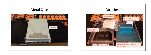
Figure E.1: Instructions for sensor node assembly, slides 1-6.
