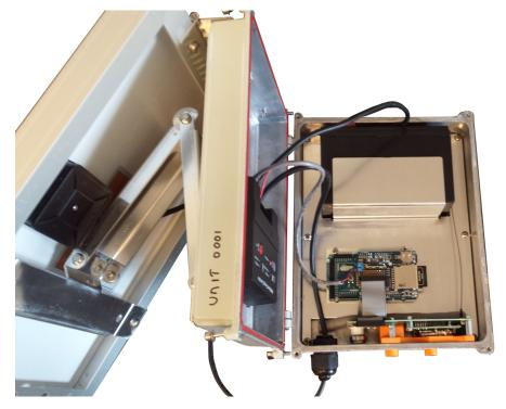
Figure 5.47: Arduino Mega development board with an real-time clock and SD card installed in an enclosures for testing.
