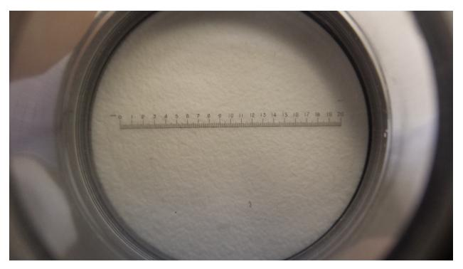
Figure 5.40: Flat mounting surface of part printed on EOSINT P 700 on 3D printed part surfaces under 10x magnification loupe. Primary tick marks on ruler denote 1 mm increments, and the secondary tick marks denote 100  $\mu$ m increments.
