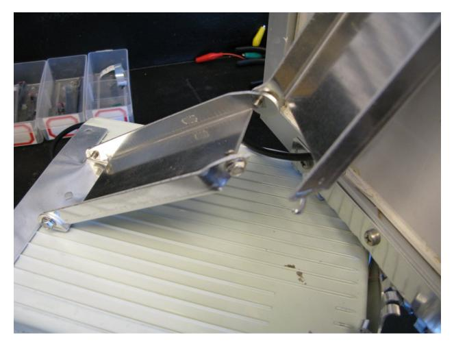
Figure 6.6: Damage to UNIT 0003: This image shows the bracket which supports the solar panel on the Tycon enclosure has been ripped by damage incurred during the impact.
