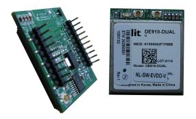
Figure 5.16: This is an example of the cellular modem utilized in the communication nodes. The two U.FL connectors allow attachment of antennas for both cellular communication as well as GPS synchronization.
