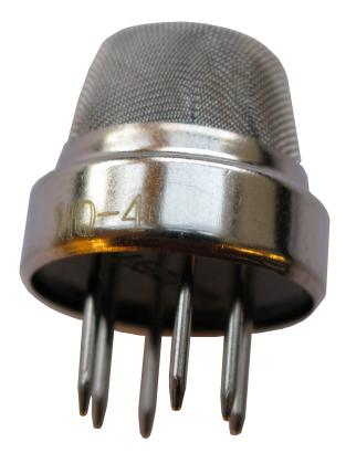
Figure 5.23: The MQ-4  $CH_4$  sensor is a pluggable unit. The wire mesh prevents damage to the delicate sensing parts, and, according to manufacturers, prevents explosions when applied to dangerous gas mixtures.
