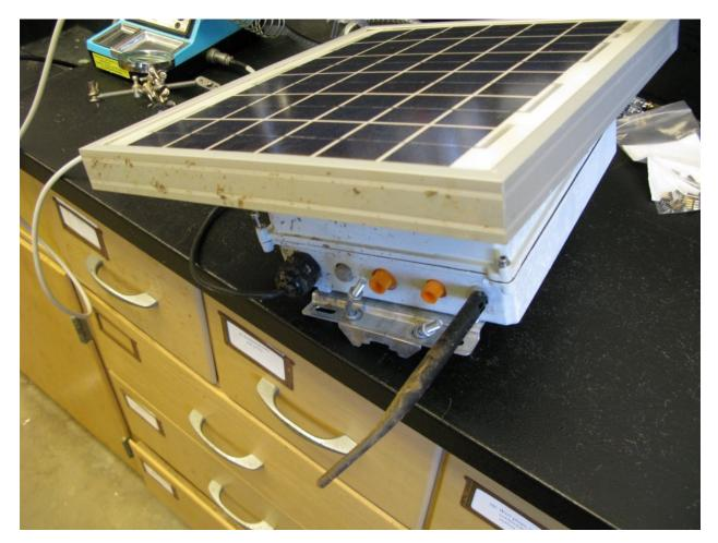
Figure 6.7: Damage to UNIT 0004: This image shows the antenna which snapped after the impact. The mud flecks on the downward facing side of the sensor confirms that this sensor was dropped straight to the ground.
