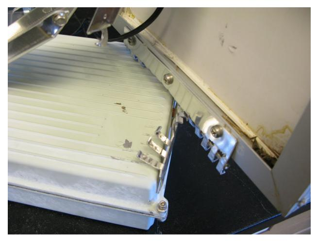
Figure 6.5: Damage to UNIT 0003: This image shows the steel hinge holding the solar panel on the Tycon enclosure has been sheared away by stress during the impact.
