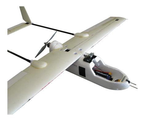
**Figure 7.1**: This image depicts one of the Unmanned Aerial Vehicles being researched at the UAS site. This unit includes a carbon dioxide and methane flow sensor mounted in the fuselage. Collaborative efforts are underway to compare the data detected by these aerial units to the units deployed in the sensor array.
