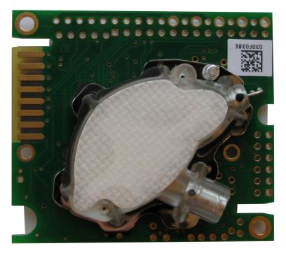
Figure 5.20: The K series  $CO_2$  sensor is an optical sensor which detects gas passing through a membrane. This is mounted on a discrete board which is mounted with standoffs on the sensor breakout board.
