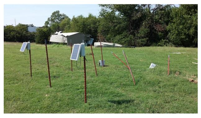
Figure 6.4: Severe damage to prototype sensors at test site after debris strike (seen in background) during gusty weather.
