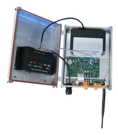
Figure 5.48: The completed sensor node was made by replacing the prototyping Arduino Mega with the custom circuit board designed for this project. This shot of the internals shows the detail of the wiring between the components in the case.
