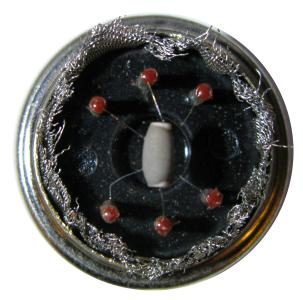
Figure 5.24: This image of the MQ-4 sensor with the metal mesh removed shows the actual sensor. A gas sensing layer on an  $Al_2O_3$  substrate is connected with Au and Pt electrodes. A nichrome filament housed within the ceramic tube heats the area during detection to improve response.
