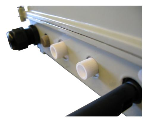
Figure 5.45: The custom part joins the sensor board and enclosure perfectly.
