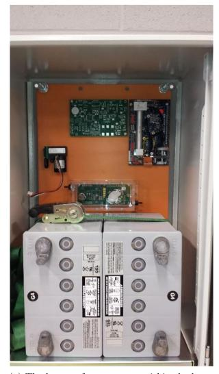
(a) The layout of components within the large communication nodes. The batteries take up most of the space inside the enclosure, so components were arranged to be bolted to the top of the back plate.
