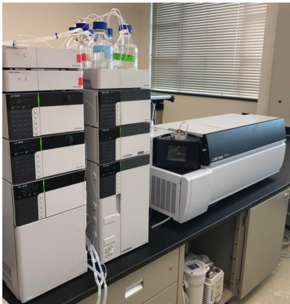
Figure 35. LC-MS/MS Instrument Setup at OSU-F TTL. Shimadzu UFLC pumps on the left and Shimadzu 80-40 MS/MS on the right.
