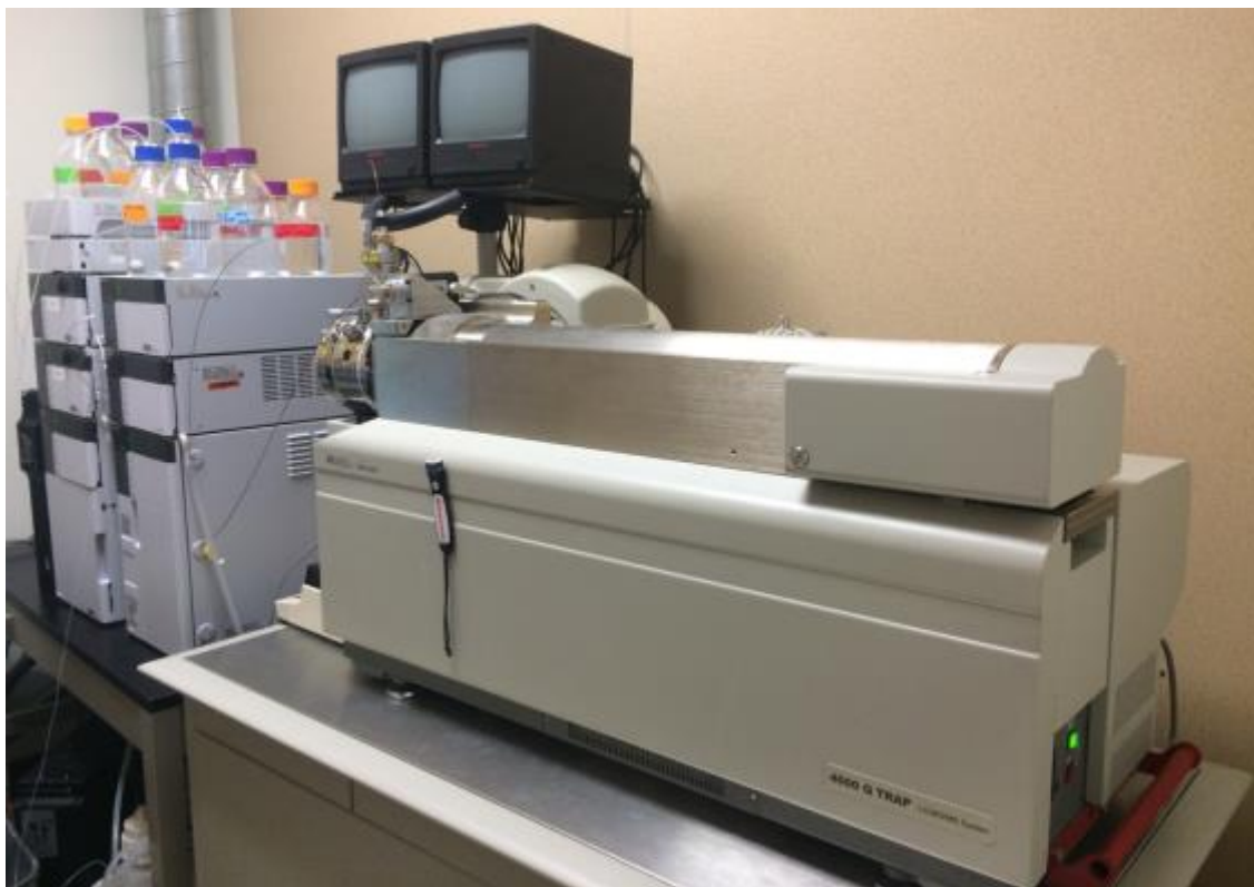
Figure 8. LC-MS/MS Instrumentation Setup at OSU-FTTL. Shimadzu UFLC pumps on the left, and Applied Biosystems 4000 Q Trap MS/MS on the right.
