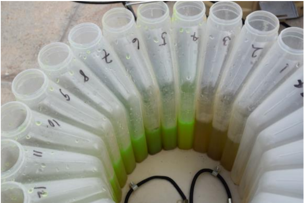
Figure 14. Collected Waste Water Samples Within Autosampler Rack. Green dye test initiated at the collection of Bottle 2, followed by 15-minute interval collections. Green dye present in Bottle 4 indicates a manhole to lift station travel time of 15-30 minutes.
