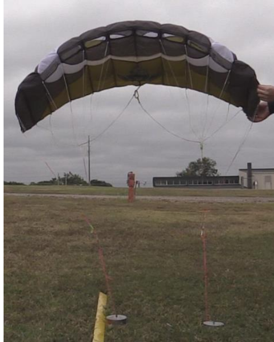
Figure 36: Ozone Quattro Parafoil with Reduced Arc Anhedral
