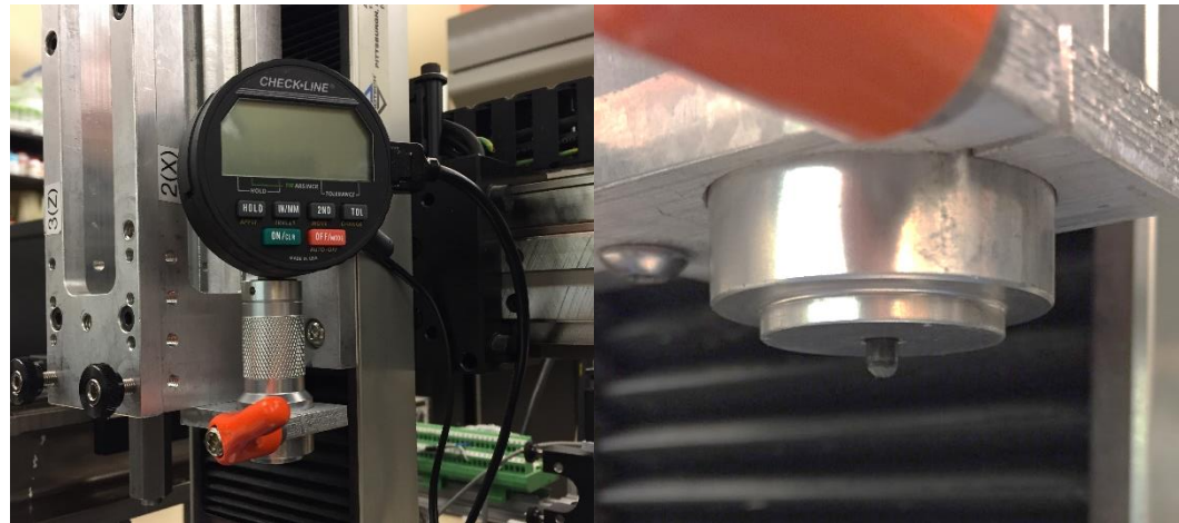
Figure 3.10: Digital image of (a) the durometer mounted to the Z-axis gantry and (b) a close-up of the durometer presser foot (indenter)
