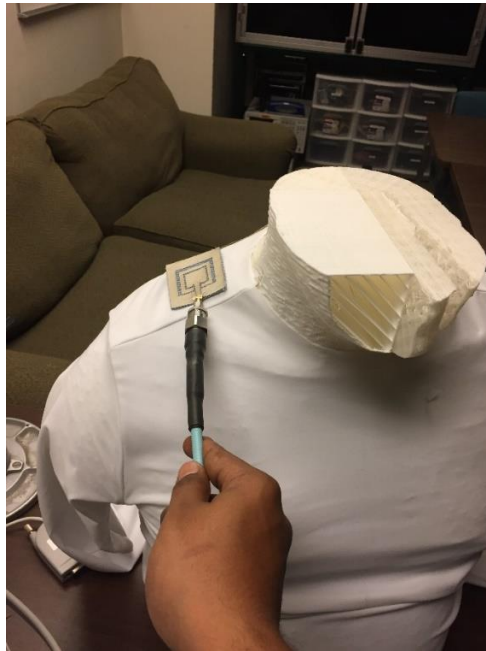
Fig. 6.15. Prototype IV on Body Phantom
