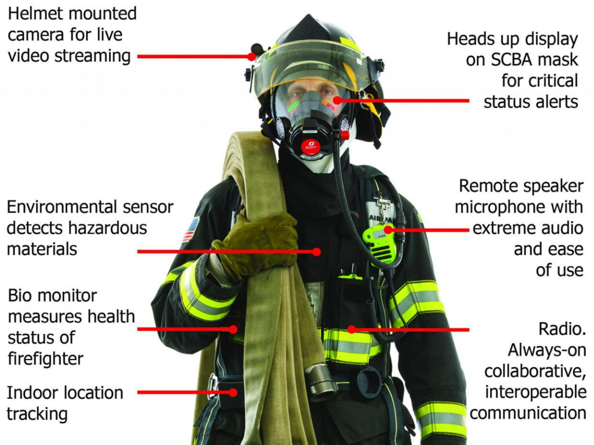
Fig. 2.5 Smart Protective Suit for Firefighters [23]
