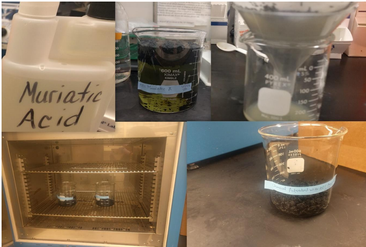
Figure 12. Chemical Treatment of carbon using muriatic acid
