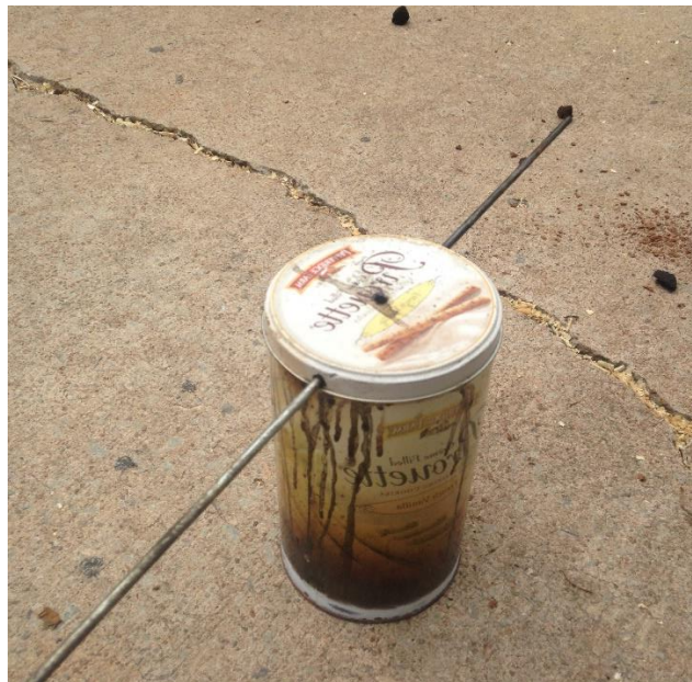
Figure 6. Charcoal oven made using a tin can with a tight fitting lid and a metal dowel
