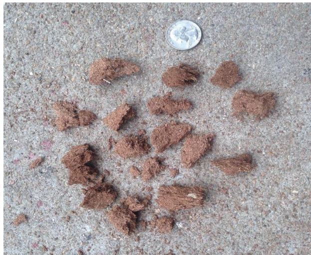
Figure 5. Coconut husk pieces no bigger than a US quarter
