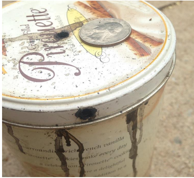
Figure 7. Small hole punctured in the center of the lid to allow gases to escape
