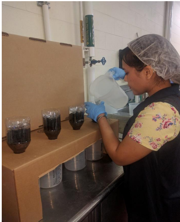
Figure 16. Pouring water through the filter bodies
