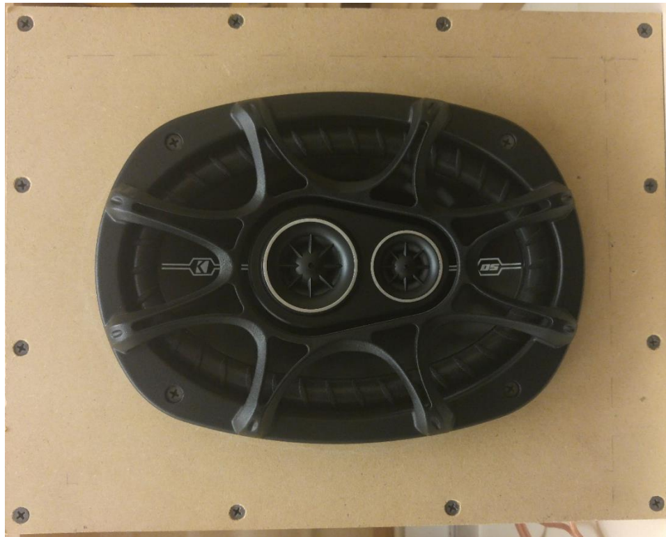
Figure 23. Kicker DSC693 6-inch by 9-inch 4Ω woofer used as acoustic source driver mounted in top of wind tunnel test section to provide normal incidence sound waves for transmission loss testing.
