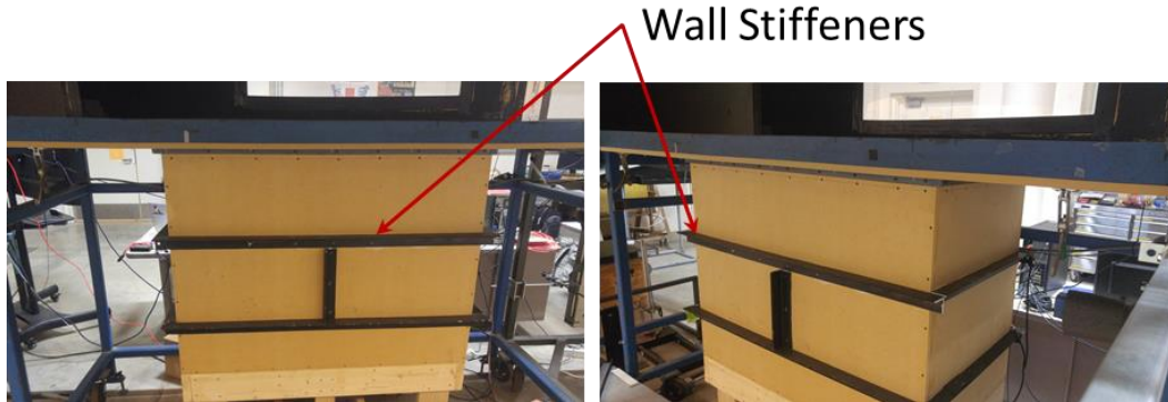
Figure 20. Photographs of quiet box after addition of aluminum angle stiffeners on outer wall panels shift natural frequency for better attenuation
