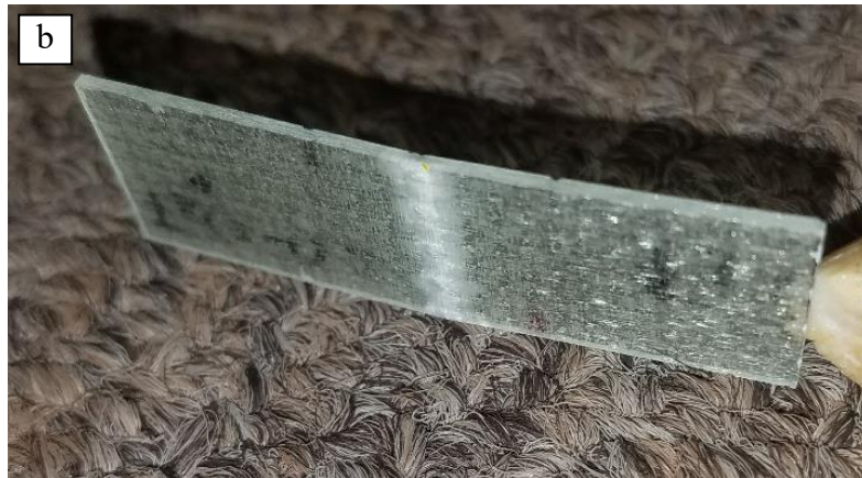
Figure 34: Fracture due to tension at the bottom surface of the laminate for both (a) random mat and (b) plain weave laminates
