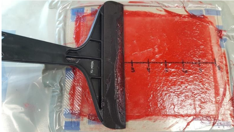
Figure 11: Foam edged scrapper used to redistribute grease during magnet application
