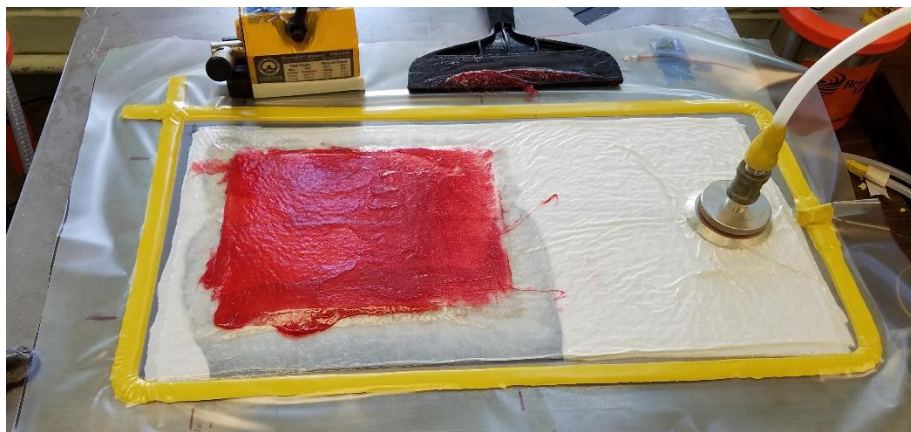
Figure 6: Completed wet layup/vacuum bag procedure with vacuum pressure applied. The magnet is applied on the greased (red) area
