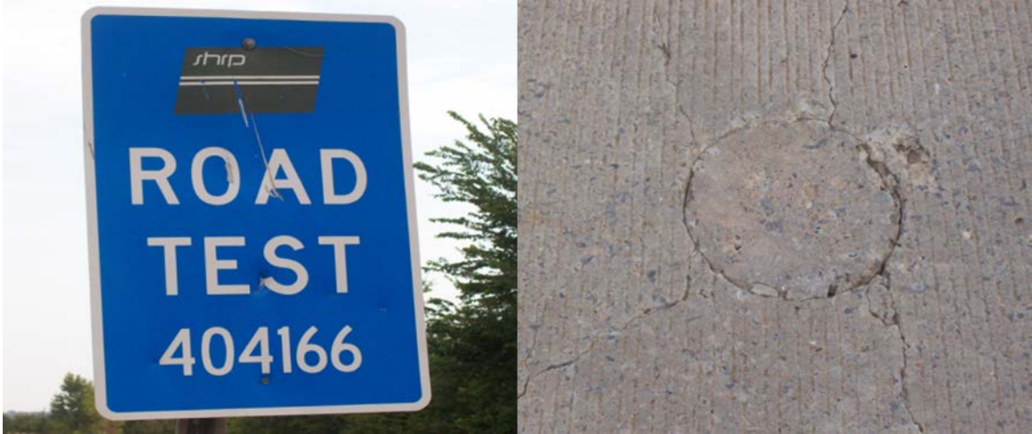
Figure A.57 (right) road test sign found beside roadway, (left) one of several large cores taken
