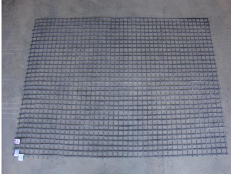
Figure 156. WGG2 geogrid specimen after exhumation
