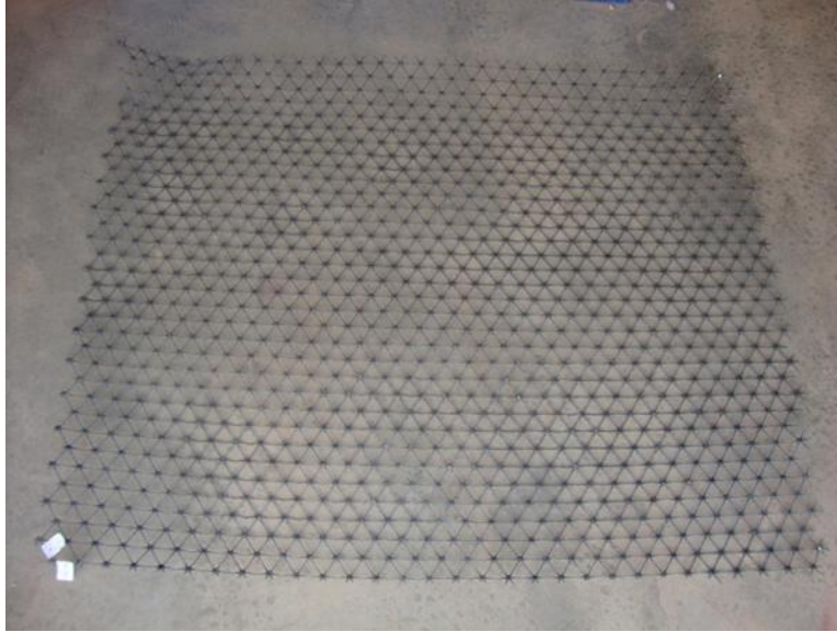
Figure 160. EGG3 geogrid specimen after exhumation
