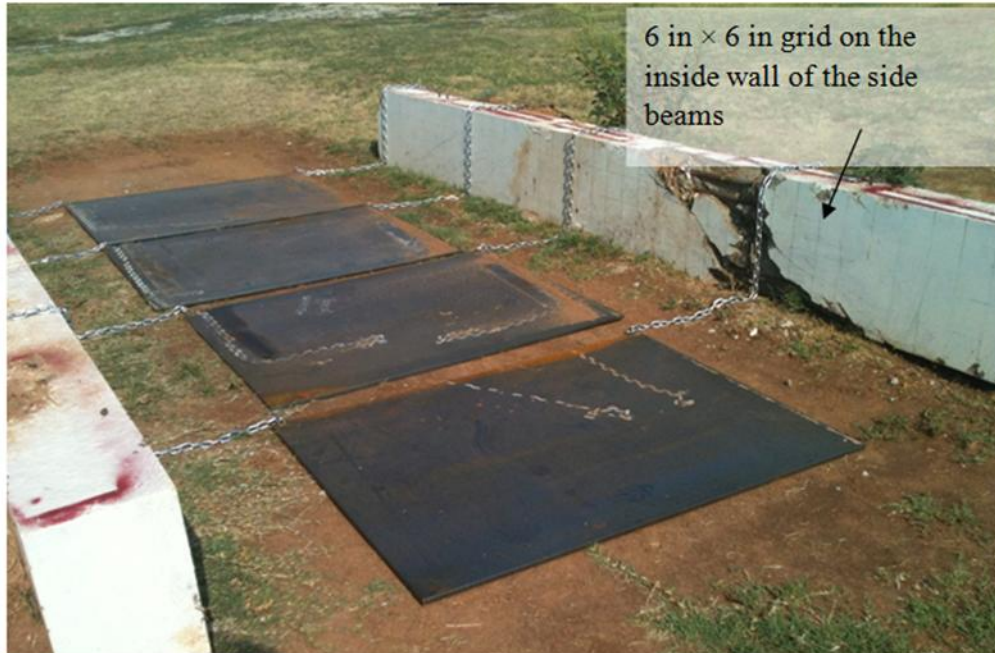
Figure 141. Four steel plates were placed in the test bed to facilitate the exhumation process of the geogrids after they were covered by compacted aggregate
