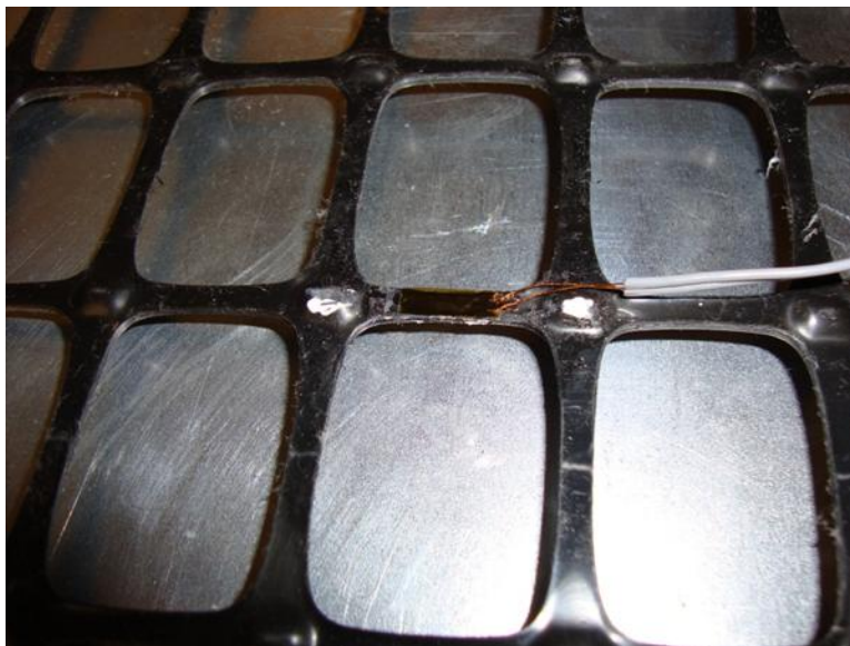
Figure 191. The tape is peeled off carefully from the strain gauge
