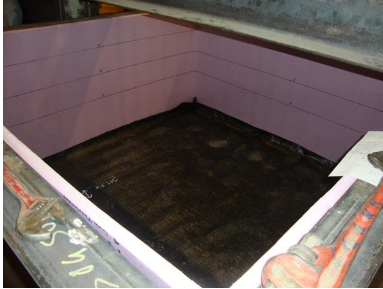
Figure 208. Cyclic plate load test box after placing the geotextile separator on Styrofoam panels on the bottom of the test box
