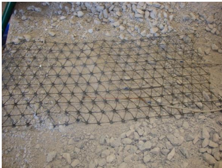
Figure 79. EGG3 geogrid after pullout test
