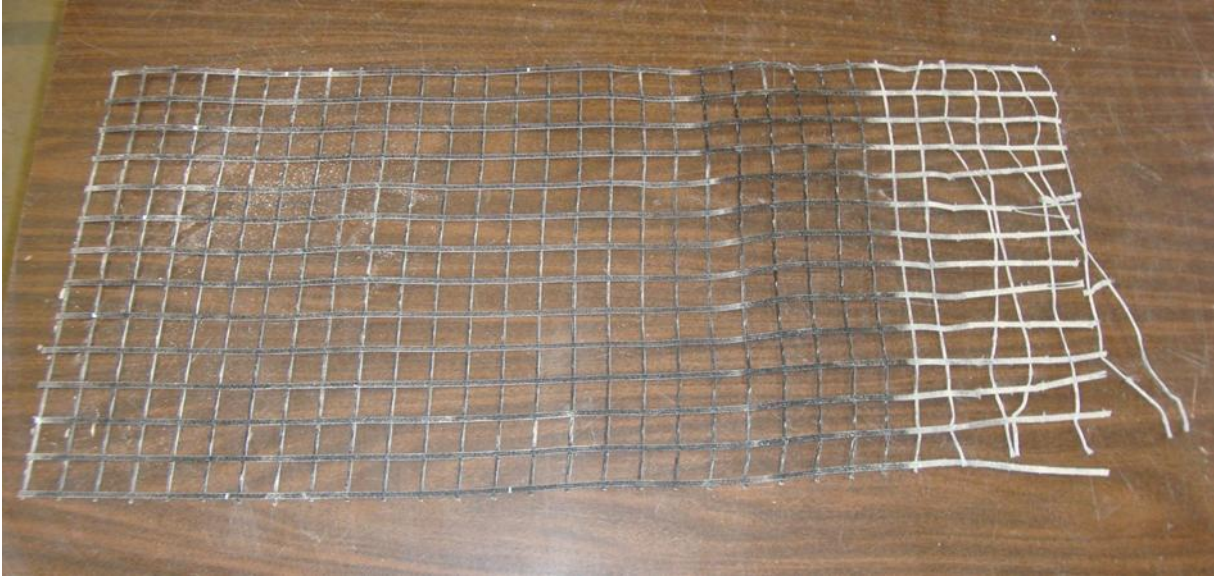
Figure 76. KGG1 geogrid after pullout test
