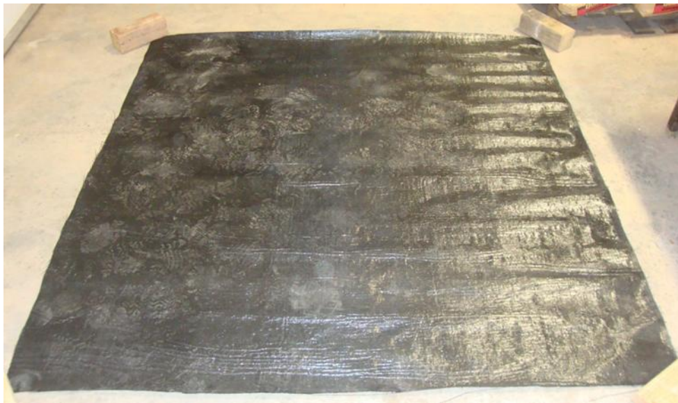
Figure 201. Geotextile for use underneath the subgrade layer in the test box
