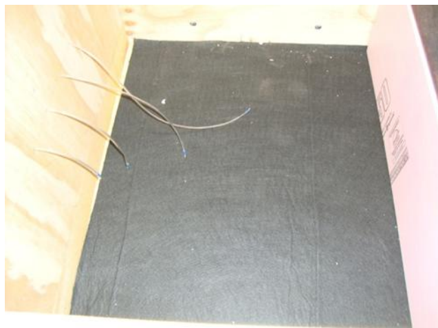
Figure 60. Pullout test box before placing the aggregate
