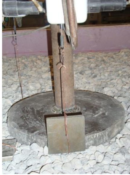
Figure 218. Vertical plate telltale to measure the aggregate deformation near the circular loading plate
