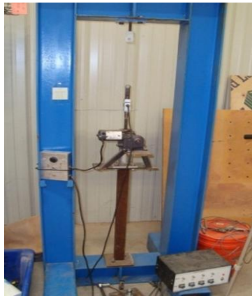
Figure 6. Tensile testing frame for testing rib and junction strength of geogrid specimens
