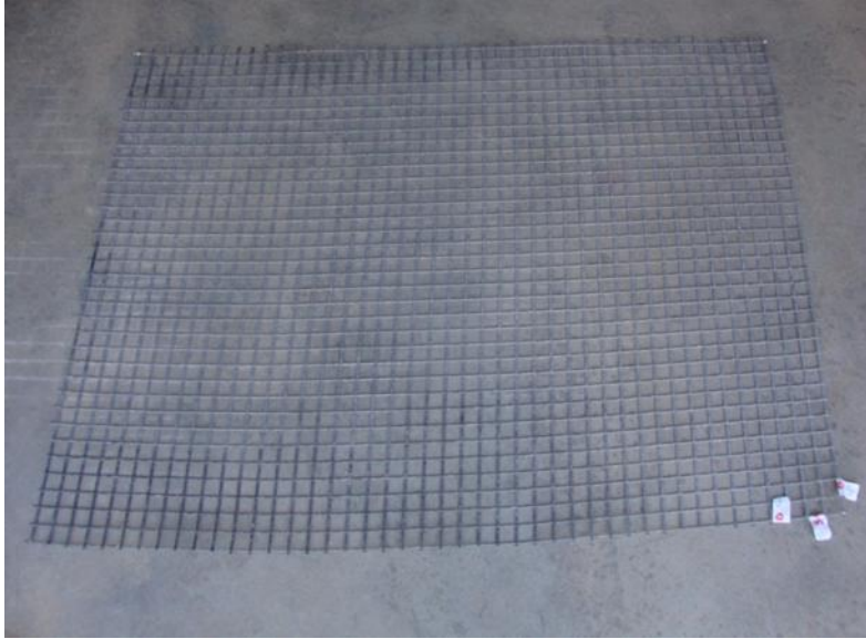
Figure 158. KGG1 geogrid specimen after exhumation
