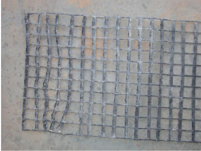
Figure 72. WGG2 geogrid after pullout test
