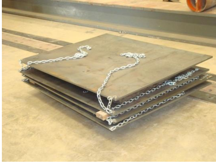
Figure 135. Steel plates with lifting chains
