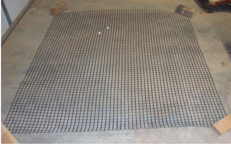
Figure 200. KGG1 geogrid specimen to be used in a cyclic plate load test (before instrumentation)
