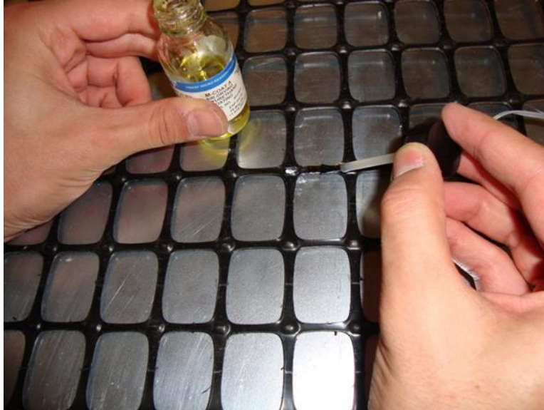
Figure 192. The gauge surface is covered with coating material
