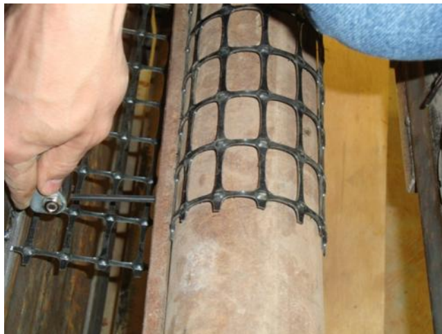
Figure 69. The geogrid is connected to the roller clamp
