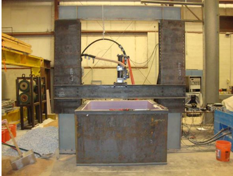
Figure 206. The redesigned and retrofitted steel loading frame with the actuator, which is connected to the hydraulic pump and the controller system
