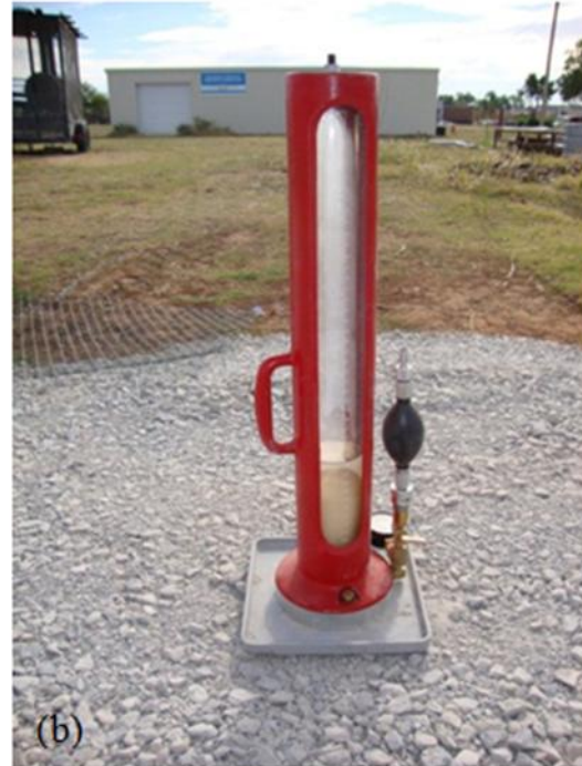
Figure 146. Measuring the in-situ density of aggregates according to ASTM D2167-08: (a) Model HM-310 Volumetric Rubber Balloon densometer, (b) The densometer in use on the test bed
