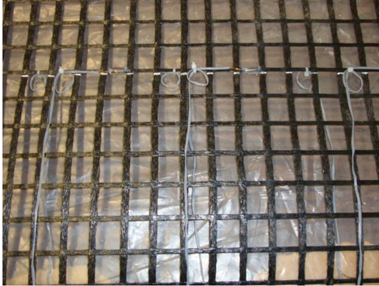
Figure 205. WGG3 geogrid specimen instrumented with strain gauges
