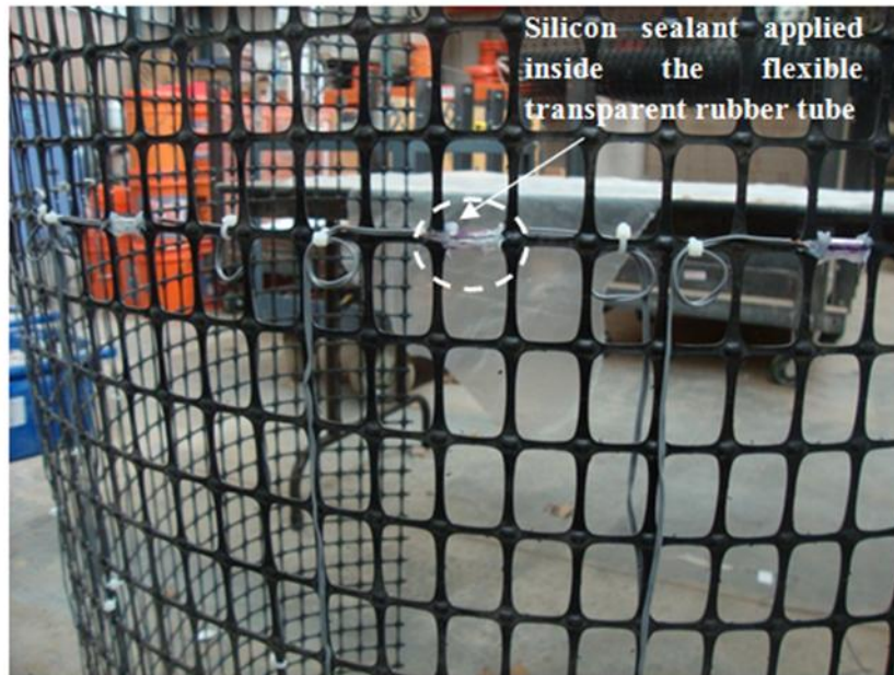
Figure 204. EGG1 (ODOT Type-2) geogrid specimen instrumented with strain gauges
