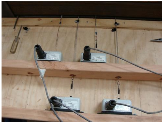
Figure 64. Tell-tale wires connected to wire potentiometers
