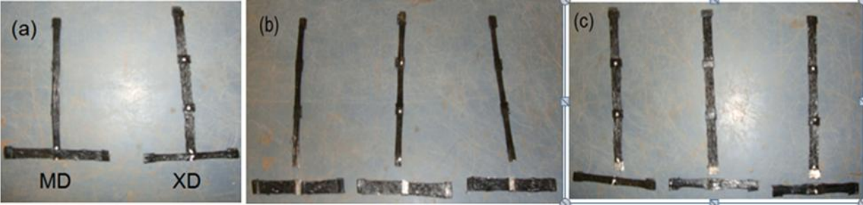
Figure 12. WGG3 geogrid junction strength specimens (a) before the test, (b) after failure (MD), (c) after failure (XD)
