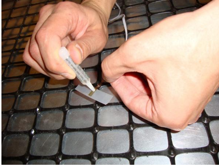
Figure 188. Application of adhesive material to the back of the strain gauge base
