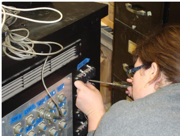
Figure 219. Connecting strain gauges to the DAS (Data Acquisition System)
