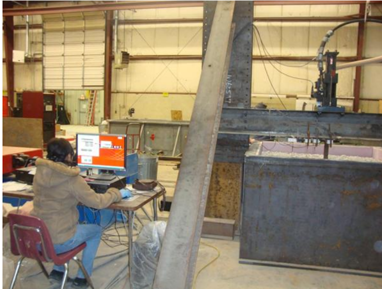
Figure 182. Cyclic loading tests on reinforced base-substrate models using a new controller system
