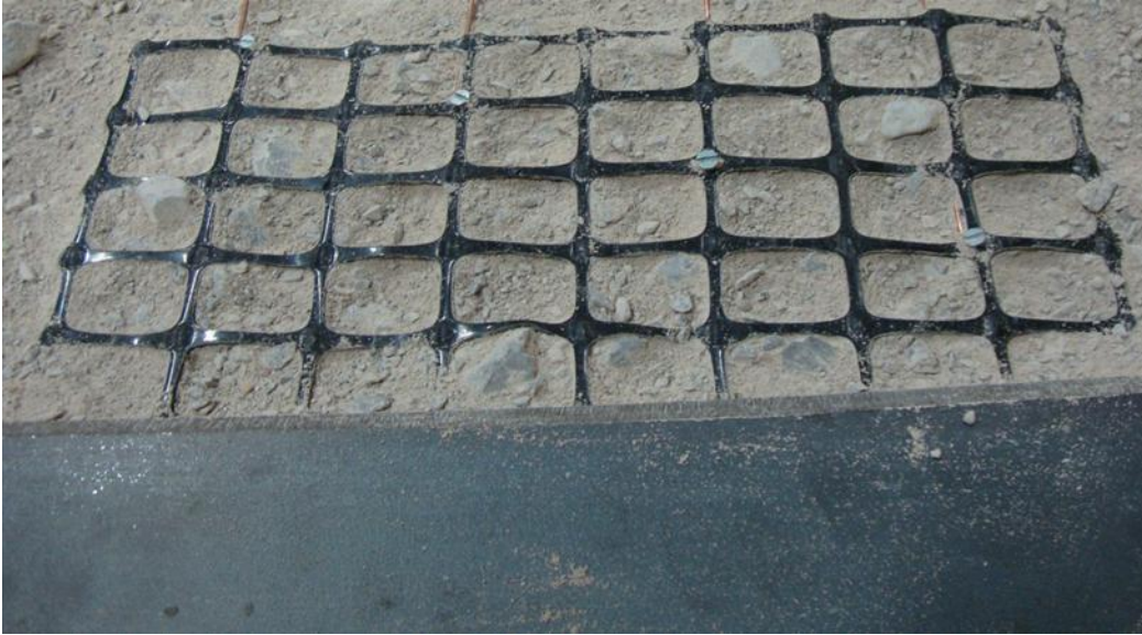
Figure 70. EGG1 geogrid after pullout test
