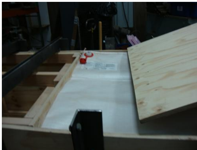
Figure 67. Air bag is used (if necessary) to generate additional overburden pressure on the geogrid-aggregate interface
