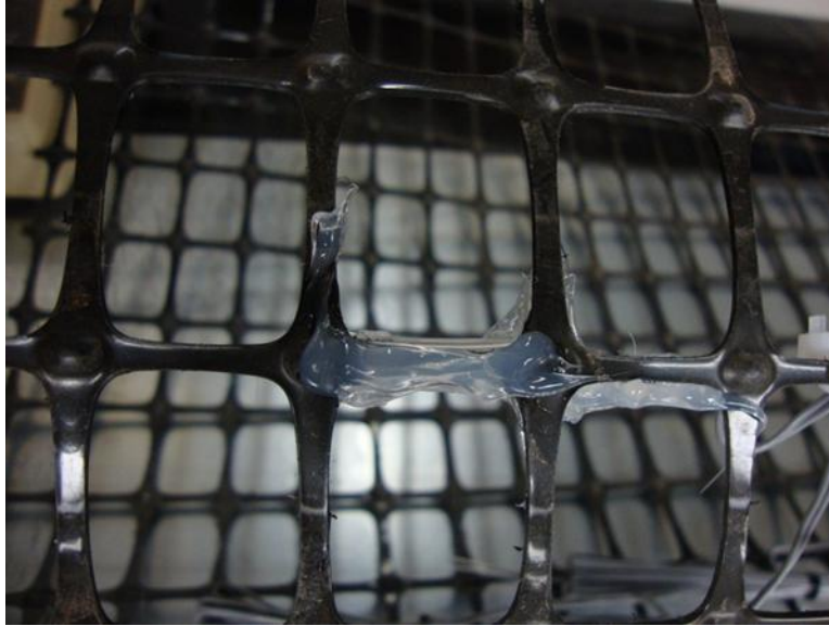
Figure 196. Siliocon rubber sealant is applied on the strain gauge
