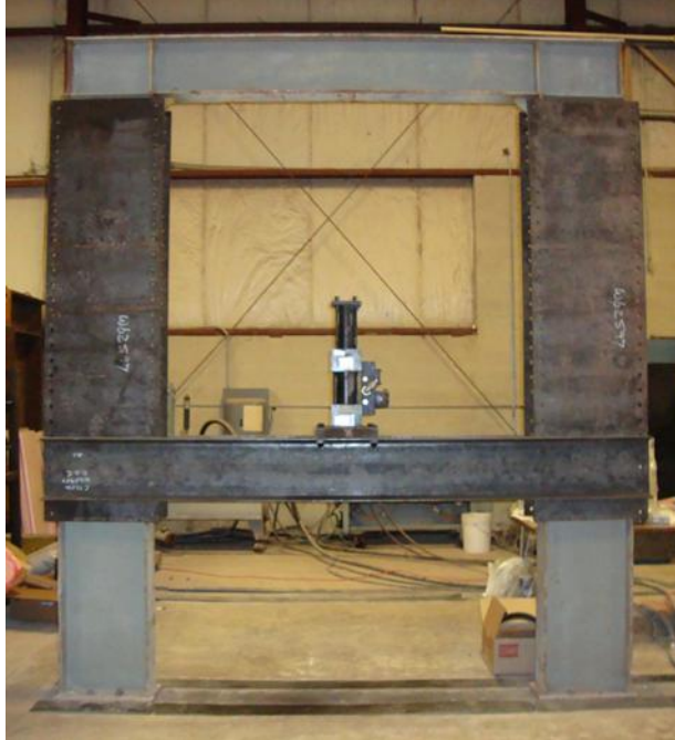
Figure 180. Redesigned and retrofitted steel loading frame at the Fears laboratory
