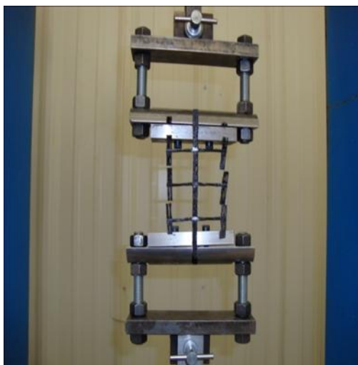
Figure 42. Rib strength testing of non-extruded geogrid in progress
