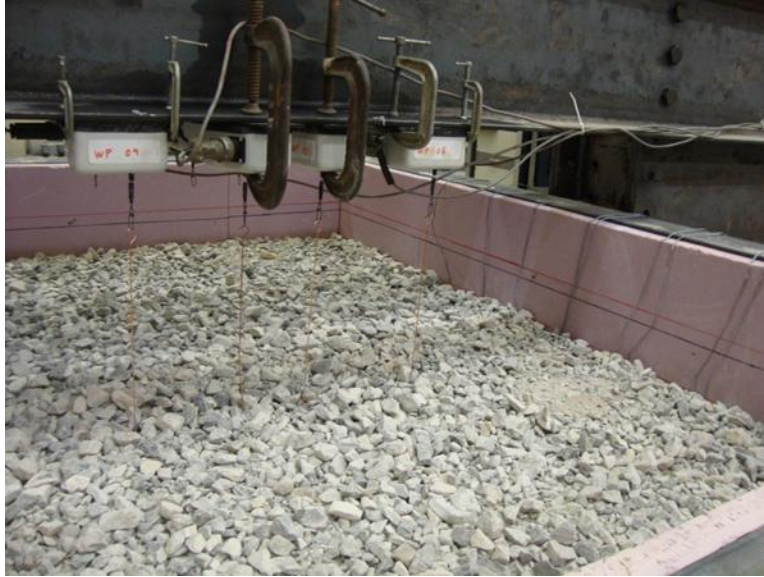
Figure 214. First 3 inches of compacted aggregate layer placed on the geogrid reinforcement
