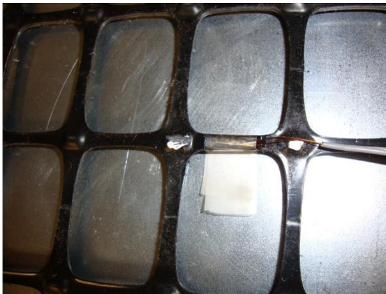
Figure 189. Gauges are held in place with the Scotch tape while the adhesive is cured
