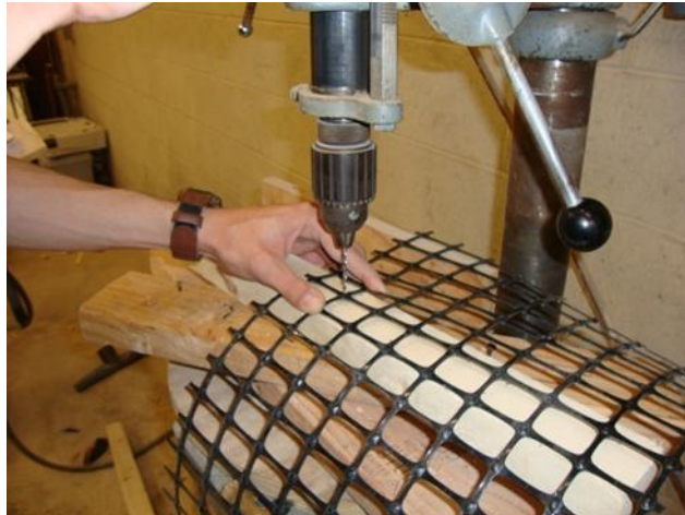
Figure 62. Drilling the geogrid junctions to connect the extensometers
