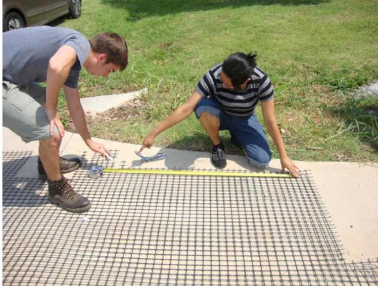
Figure 122. Geogrid sample preparation
