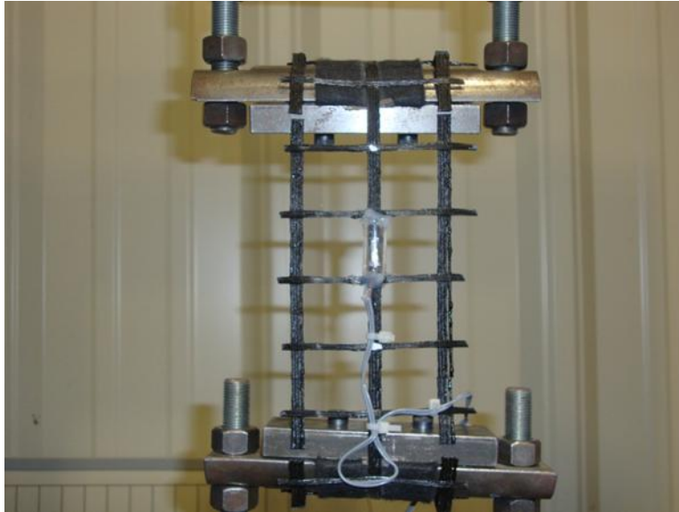
Figure 202. Determination of calibration factor of strain gauges attached to NEGG geogrid products (test setup following the ASTM D 6637 test standard)
