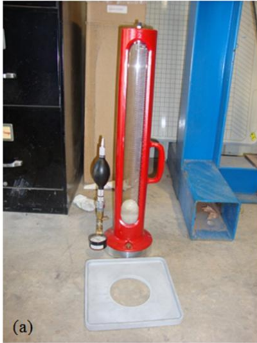
Figure 146. Measuring the in-situ density of aggregates according to ASTM D2167-08: (a) Model HM-310 Volumetric Rubber Balloon densometer, (b) The densometer in use on the test bed
