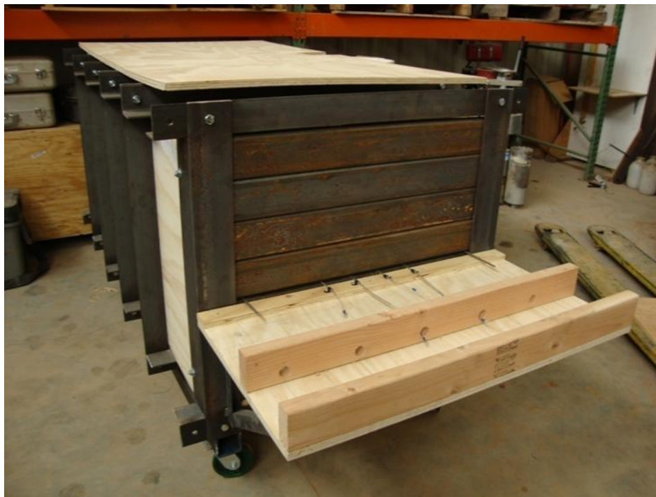
Figure 59. One of the two pullout test boxes at the OU Fears laboratory
