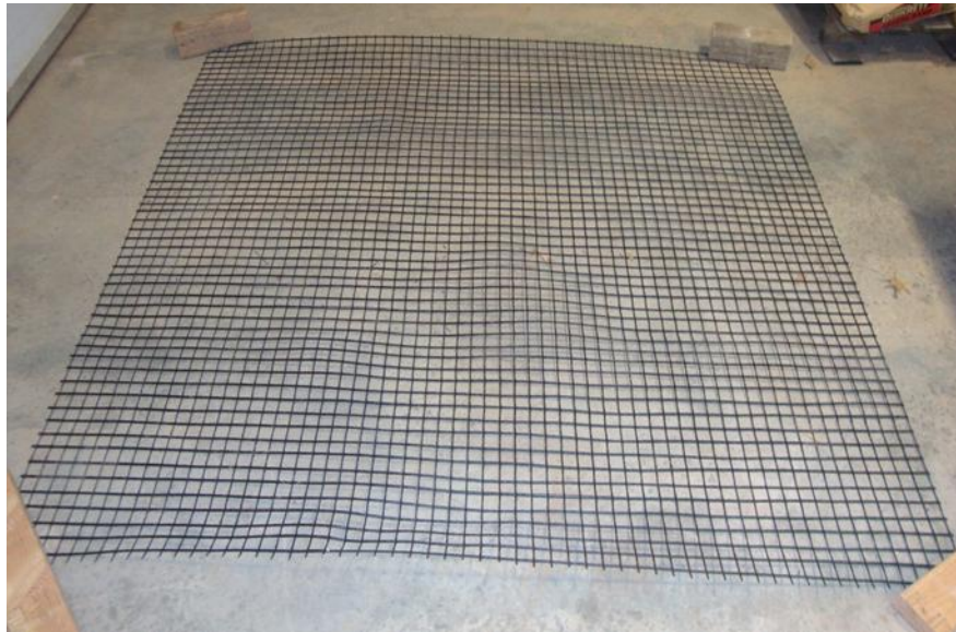
Figure 199. WGG1 geogrid specimen to be used in a cyclic plate load test (before instrumentation)
