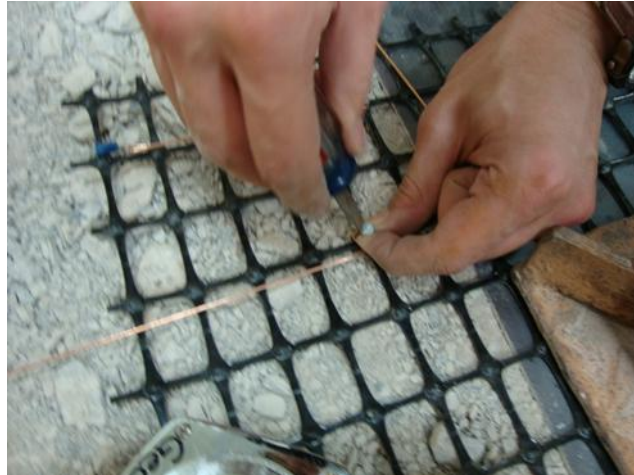
Figure 63. Connecting wires to geogrid specimen
