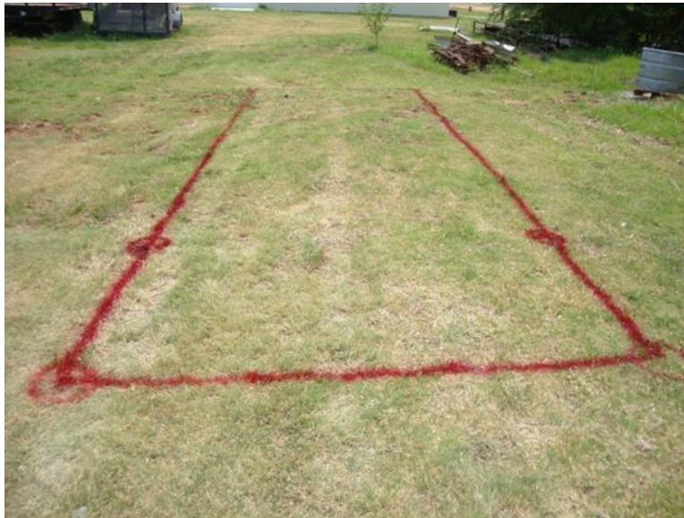
Figure 137. Test site for the installation damage tests of geogrids outside the Fears Laboratory
