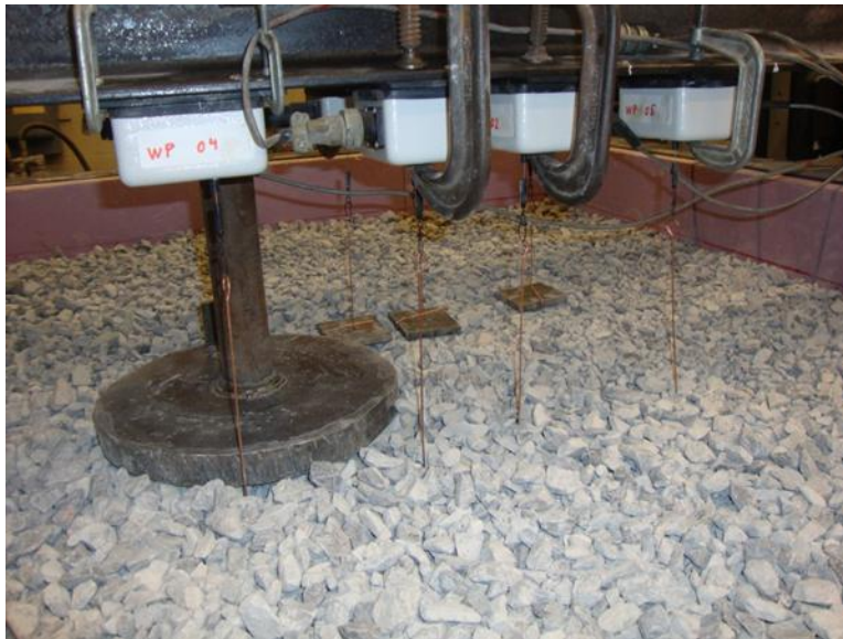
Figure 215. Brass wires connected to the wire potentiometers to measure the base layer deformation
