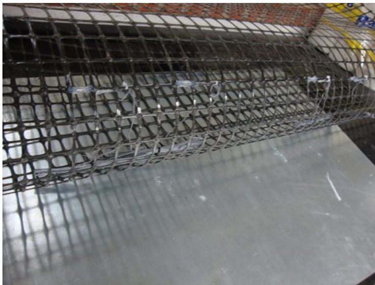
Figure 197. Geogrid sample after the installation of strain gauges
