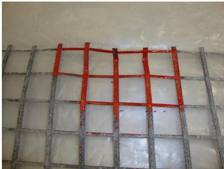
Figure 163. KGG1 geogrid sample with marked damaged area
