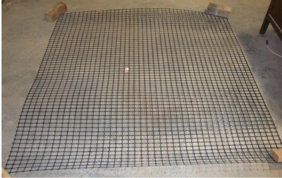
Figure 198. EGG1 (ODOT Type-2) geogrid specimen to be used in a cyclic plate load test (before instrumentation)
