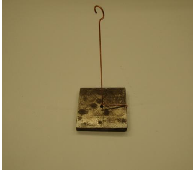
Figure 216. Telltale plates for the wire potentiometers to measure the surface deflection of the aggregate layer
