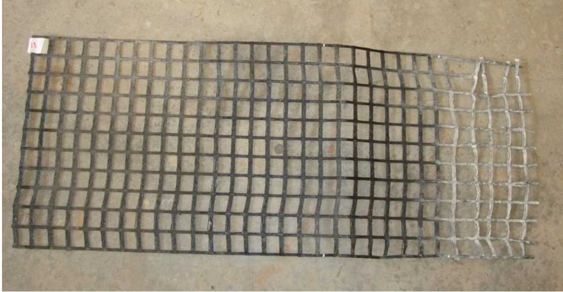
Figure 74. WGG3 geogrid after pullout test
