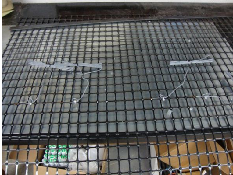
Figure 194. Geogrid with strain gauges attached
