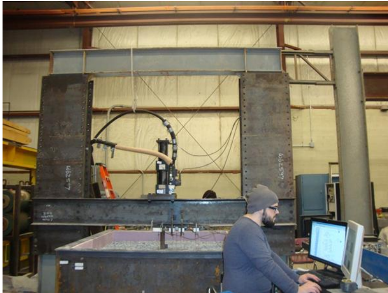
Figure 221. Monitoring data in the Data Acquisition System while the cyclic plate load test is in progress
