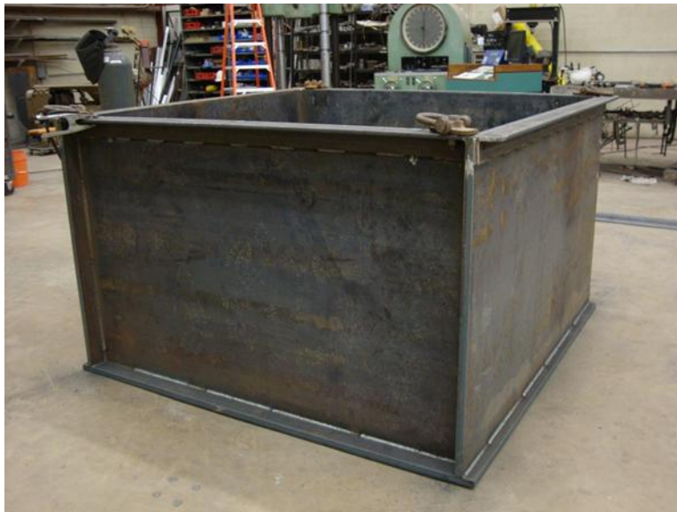
Figure 181. The newly fabricated large steel test box [6 ft (L) \times 6 ft (W) \times 3.5 ft (H)] for cyclic plate load tests
