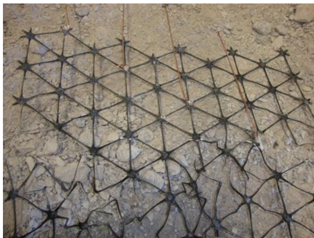
Figure 82. EGG4 geogrid after pullout test subjected to 138 psf overburden pressure
