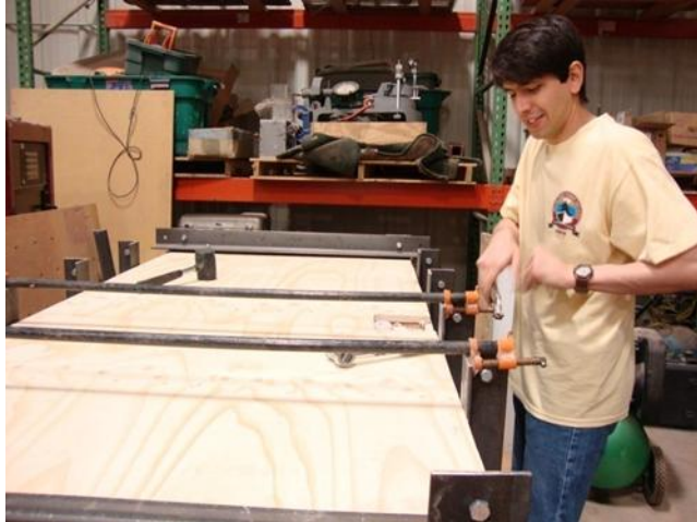
Figure 68. The pullout test box is closed before the test
