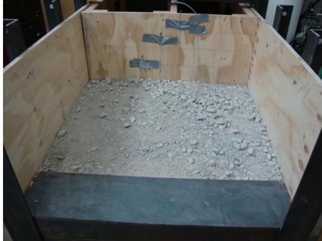
Figure 61. Compacted aggregate in the pullout box (the 8 inch-wide lower steel sleeve can be seen in the foreground)
