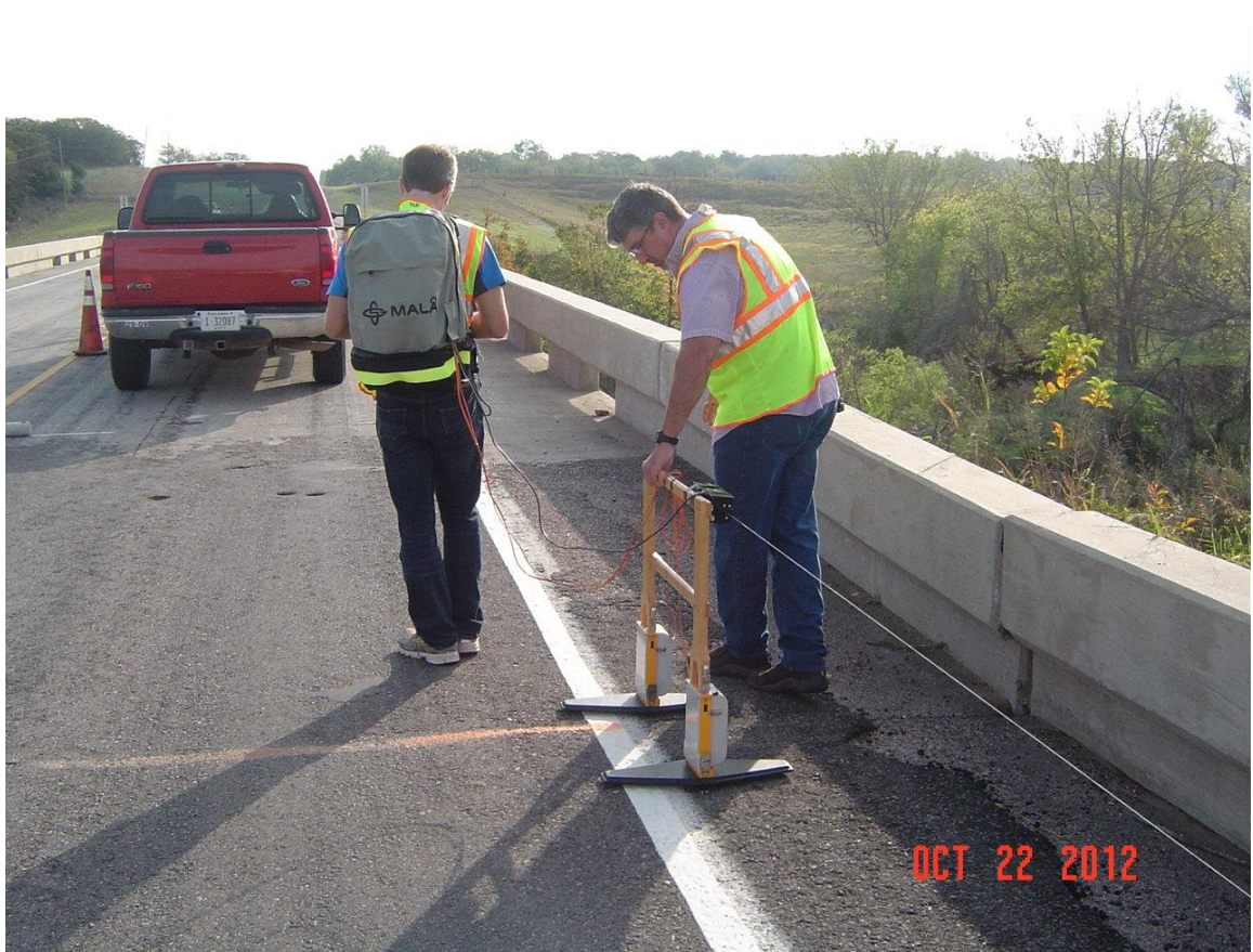
Figure 5.9 Photograph Showing Use of Portable GPR at SH-59A over Big Creek
