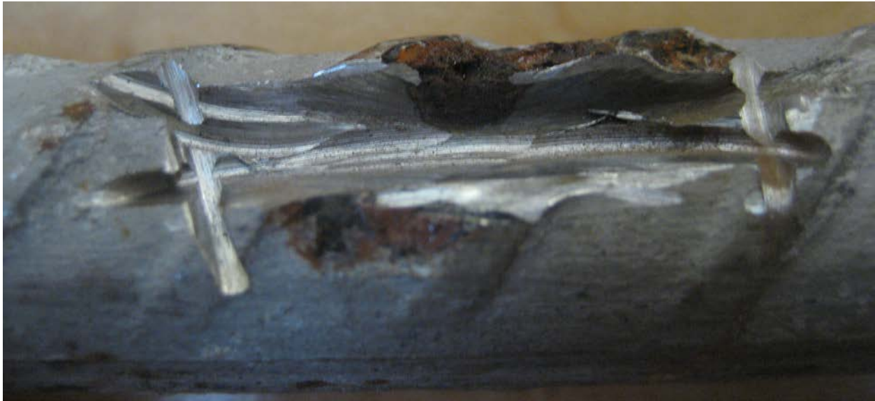
Figure 97e: Bars from Southern Exposure specimen 5 containing stainless steel clad reinforcement with four holes through the cladding after autopsy, showing extent of corrosion underneath the hole
