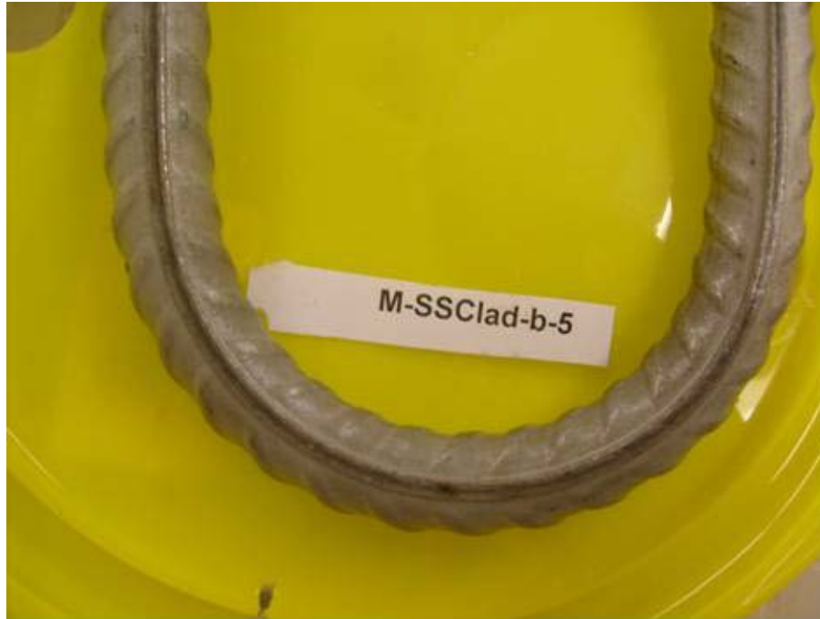
Figure 50: Rapid macrocell specimen upon completion of test, bent stainless steel clad reinforcement (anode)
