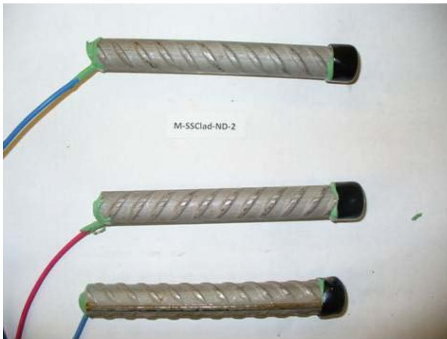
Figure 45: Rapid macrocell specimen upon completion of test, undamaged stainless steel clad reinforcement (anode on top, cathode on bottom)
