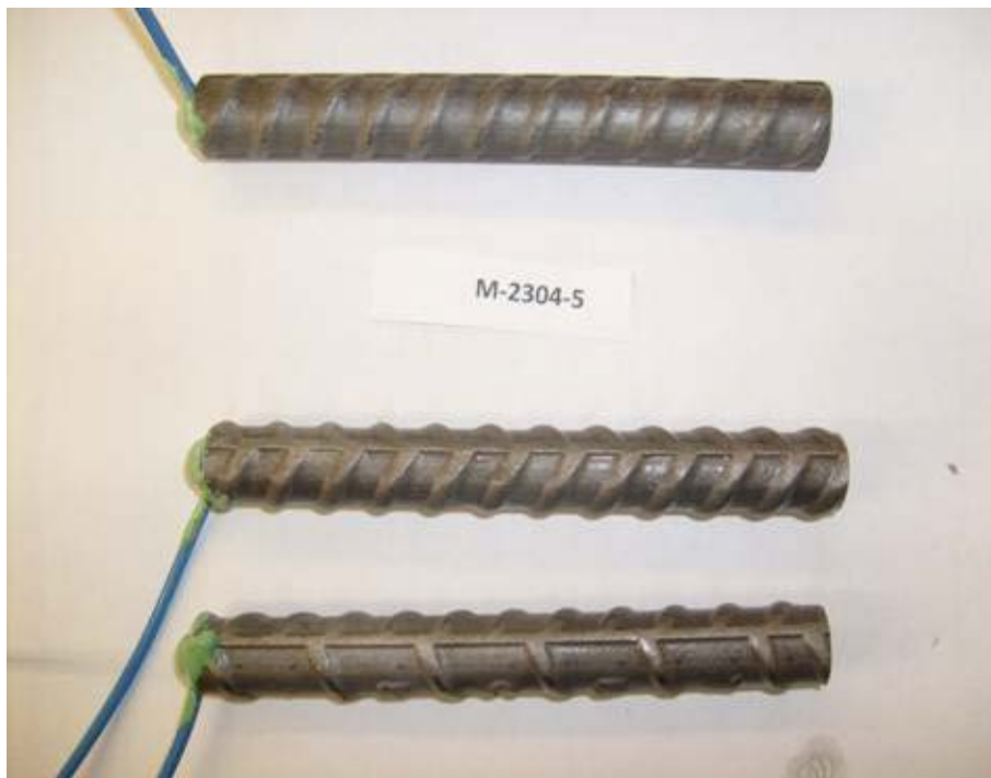
Figure 41: Rapid macrocell specimen upon completion of test, 2304 stainless steel (anode on top, cathode on bottom)
