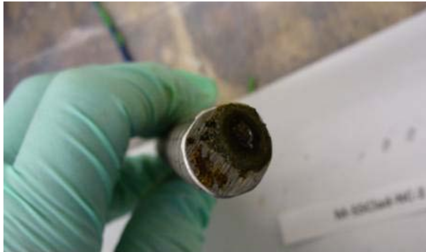
Figure 30: Uncapped bar end upon autopsy, NX-SCR™ stainless steel clad bar
