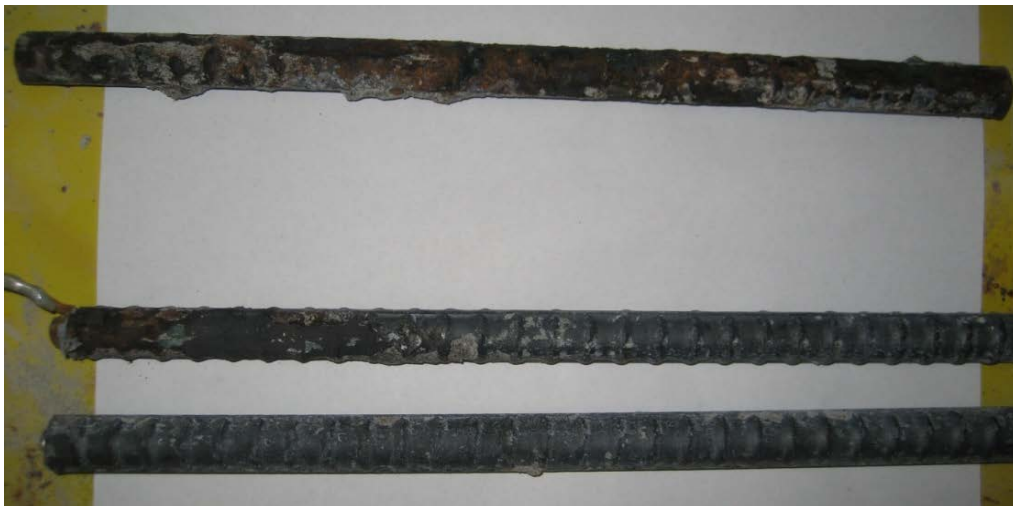
Figure 87b: Bars from cracked beam specimen 1 containing conventional reinforcement after autopsy
