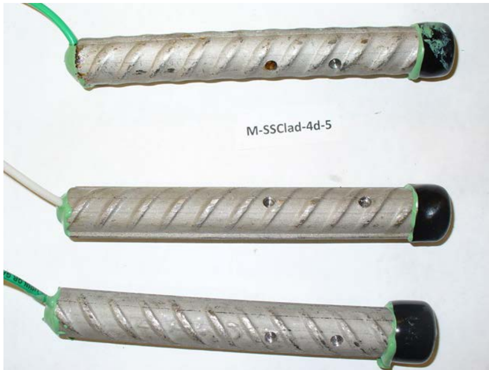
Figure 34: Photograph of specimen SSClad-4h-5 upon completion of the rapid evaluation test, NX-SCR™ stainless steel clad with four holes through the cladding (anode on top, cathode on bottom)
