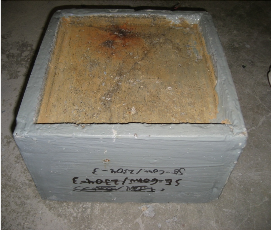
Figure 88a: Staining on Southern Exposure specimen 3 containing mixed Conv./2304 (anode/cathode)
