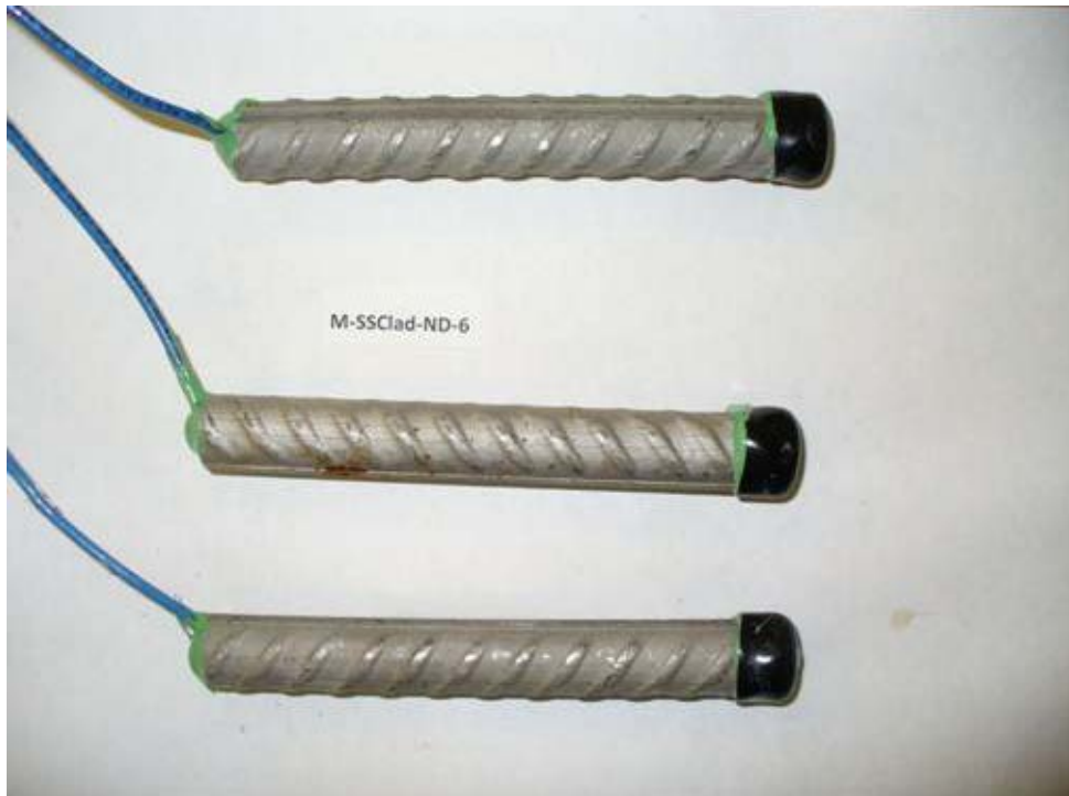
Figure 28a: Photograph of specimen 6 upon completion of the rapid evaluation test, NX-SCR™ stainless steel clad (anode on top, cathode on bottom)
