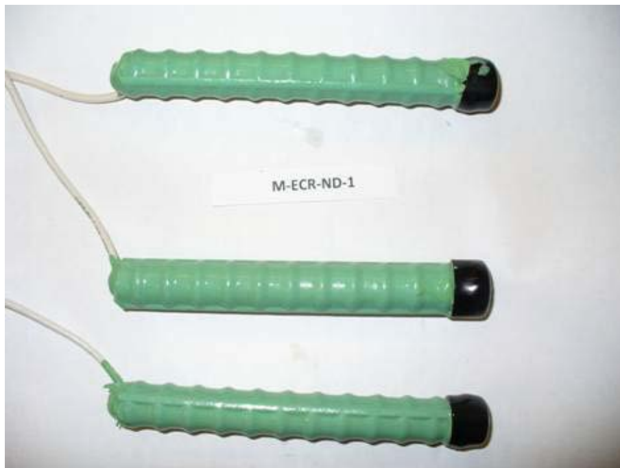
Figure 39: Rapid macrocell specimen upon completion of test, undamaged ECR (anode on top, cathode on bottom)
