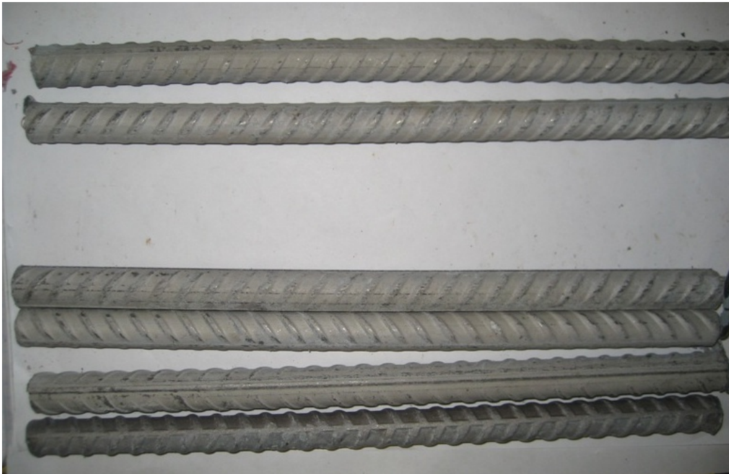
Figure 98a: Bars from Southern Exposure specimen 5 containing undamaged stainless steel clad reinforcement after autopsy
