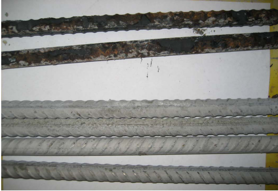
Figure 90: Bars from Southern exposure specimen 1 containing conventional reinforcement as the anode and stainless steel clad reinforcement as the cathode after autopsy
