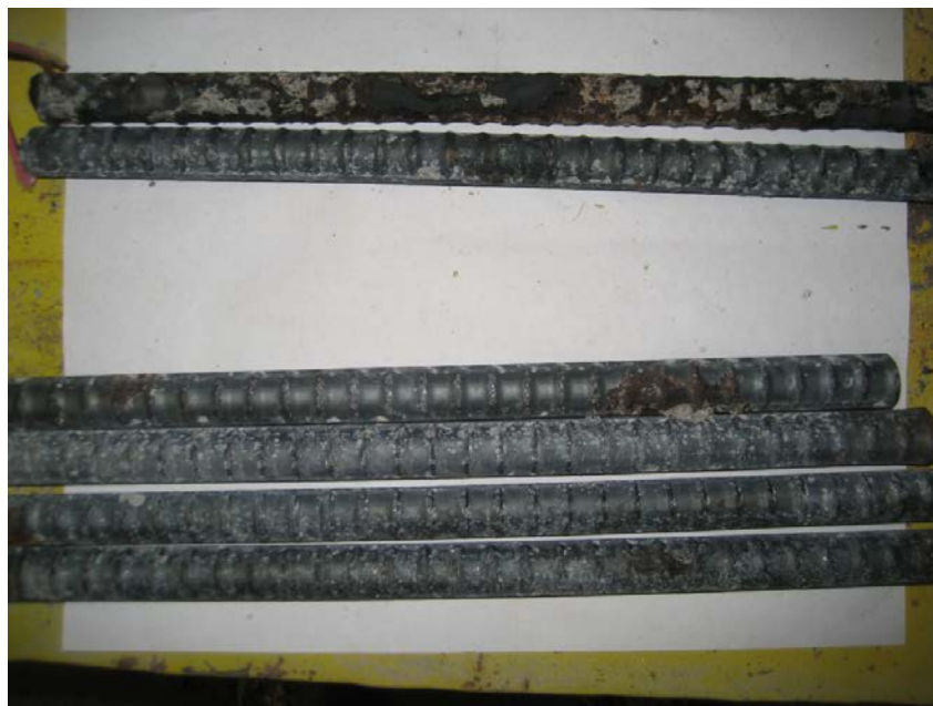
Figure 86b: Bars from Southern Exposure specimen 2 containing conventional reinforcement after autopsy
