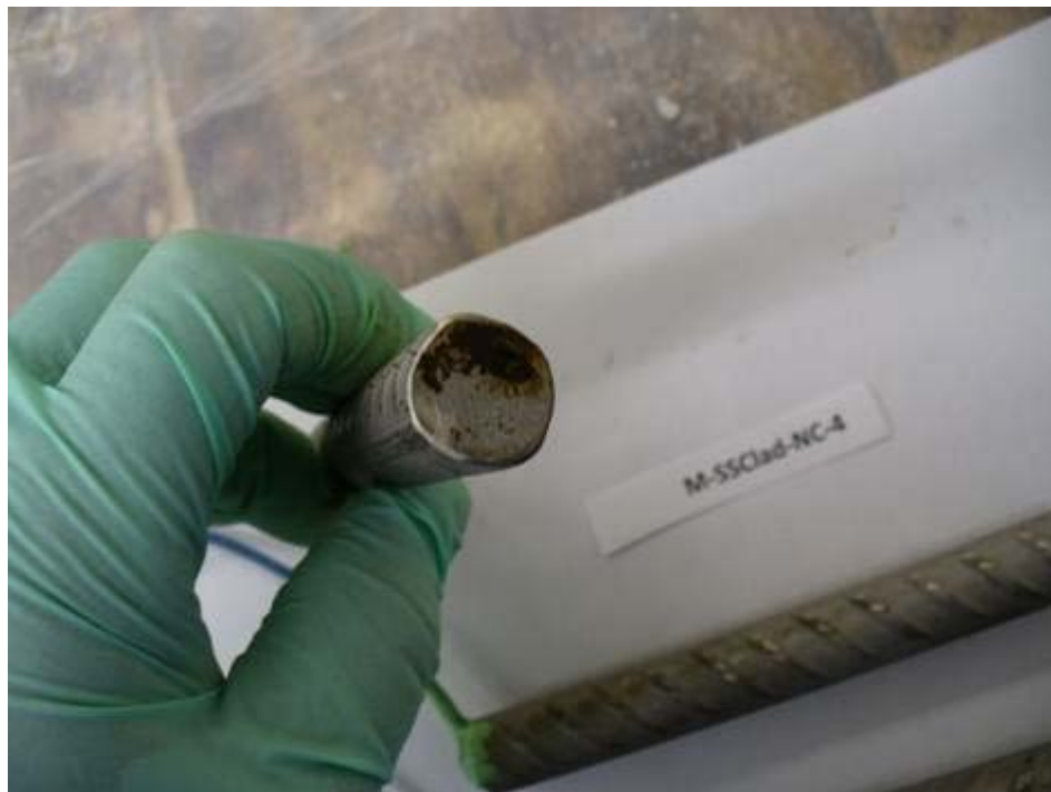
Figure 49: Rapid macrocell specimen upon completion of test, uncapped stainless steel clad reinforcement (close-up of bar end)
