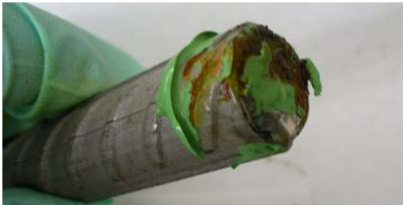
Figure 36: Corrosion under protective cap at end of evaluation, NX-SCR™ stainless steel clad bar, Specimen 2 (close-up)
