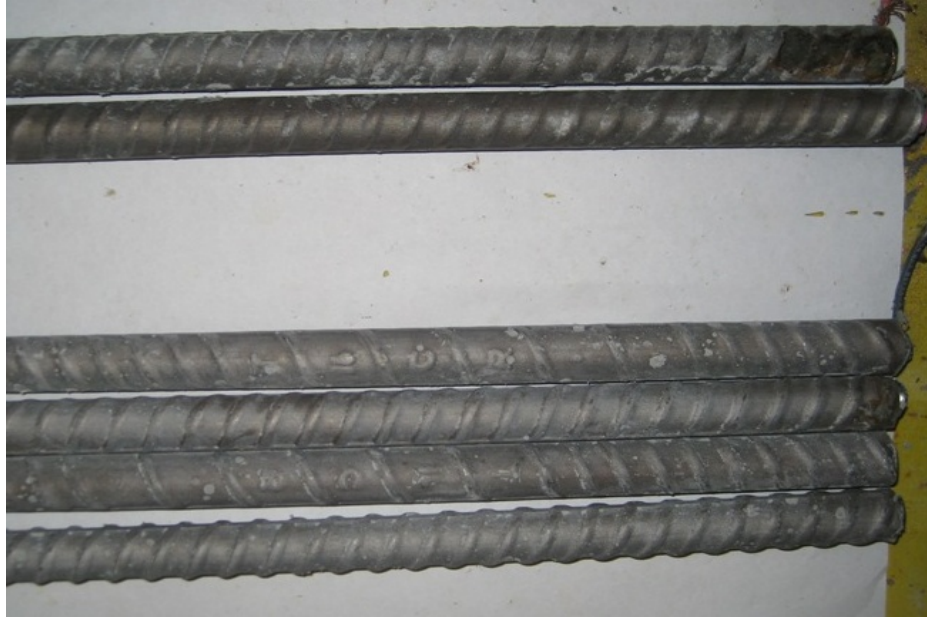
Figure 95: Bars from Southern Exposure specimen 2 containing 2304 stainless steel after autopsy
