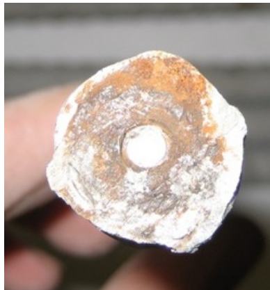
Figure 80b: Corrosion on end of SE-SSClad-b-2 cathode bar
