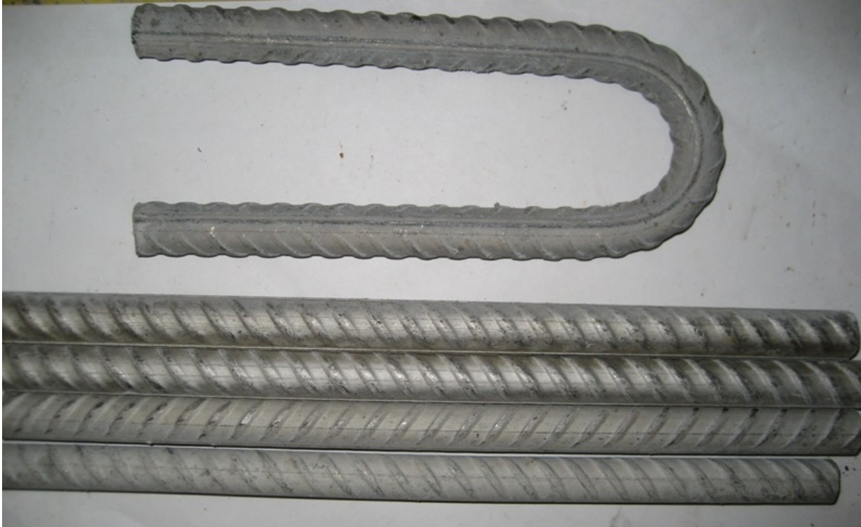
Figure 100: Bars from Southern Exposure specimen 5 containing bent stainless steel clad reinforcement after autopsy
