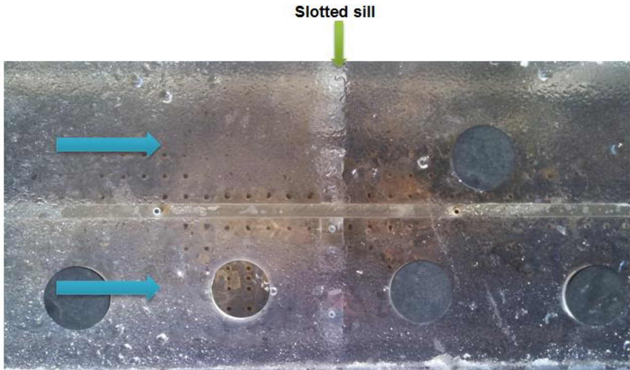
Figure 49. Experiment 29A under pressure flow using a slotted sill (sand)
