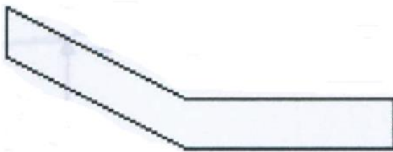
Figure 1c. Elevation view of single Broken-Back culvert
