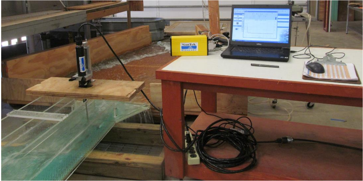
Figure 13. ADV plugged to measure the downstream velocity ( V_{d/s} )
