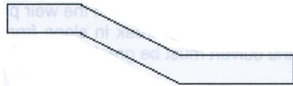
Figure 1d. Elevation view of double Broken-Back culvert
