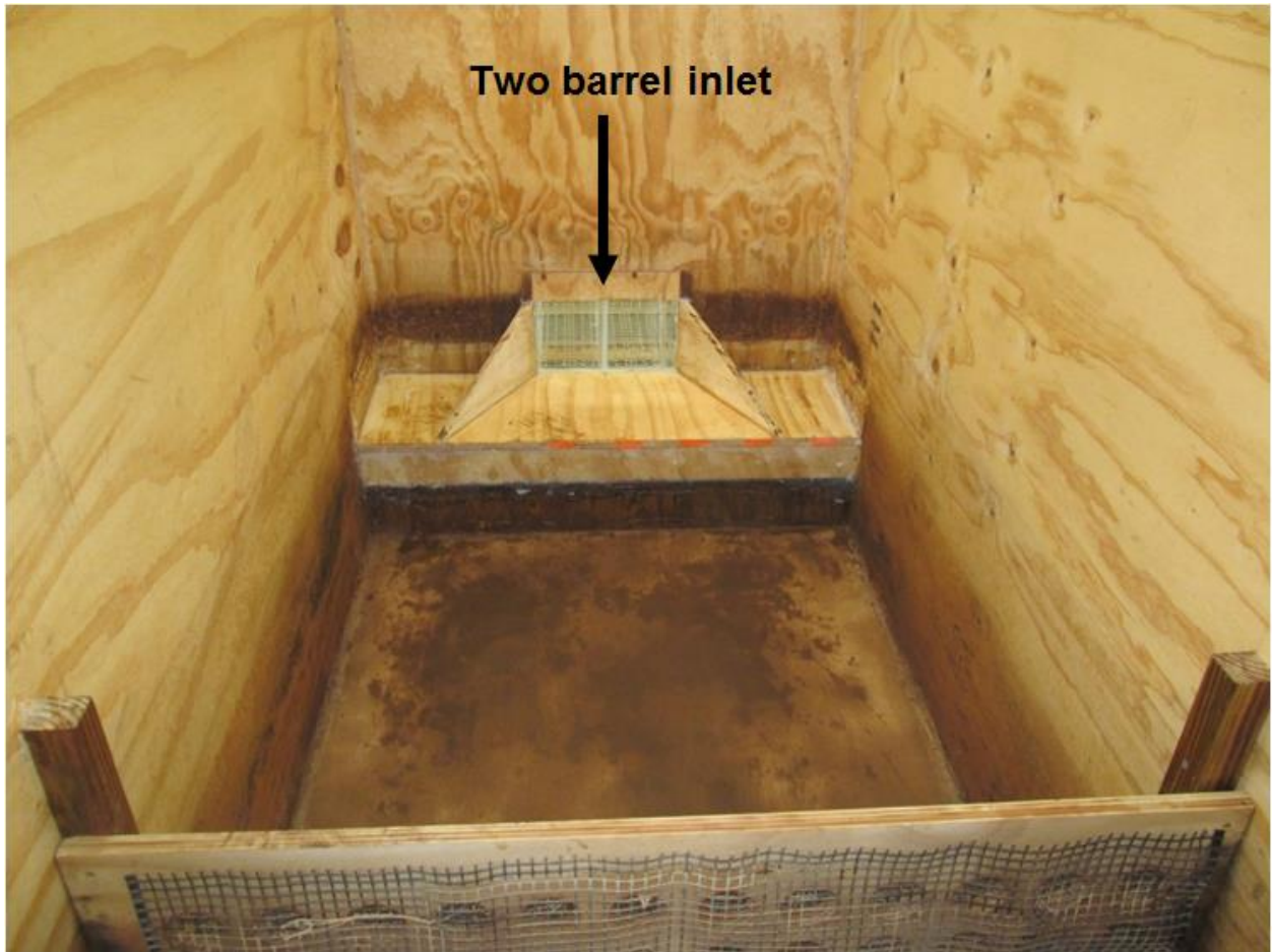
Figure 7. Reservoir and flow straightener
