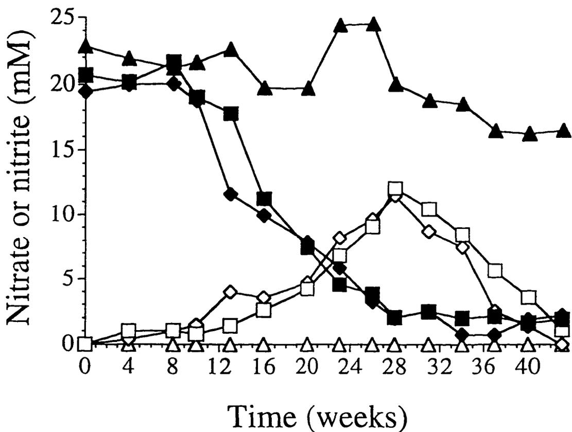
*Figure 6:* Nitrate reduction and nitrite accumulation associated with thiol metabolism in enrichment cultures. Nitrate was reduced (■) and nitrite (□) transiently accumulated in hexanethiol-degrading cultures and cyclohexanethiol-degrading cultures (◆ nitrate; ◇ nitrite), but not in sterile controls (▲ nitrate; △ nitrite).
