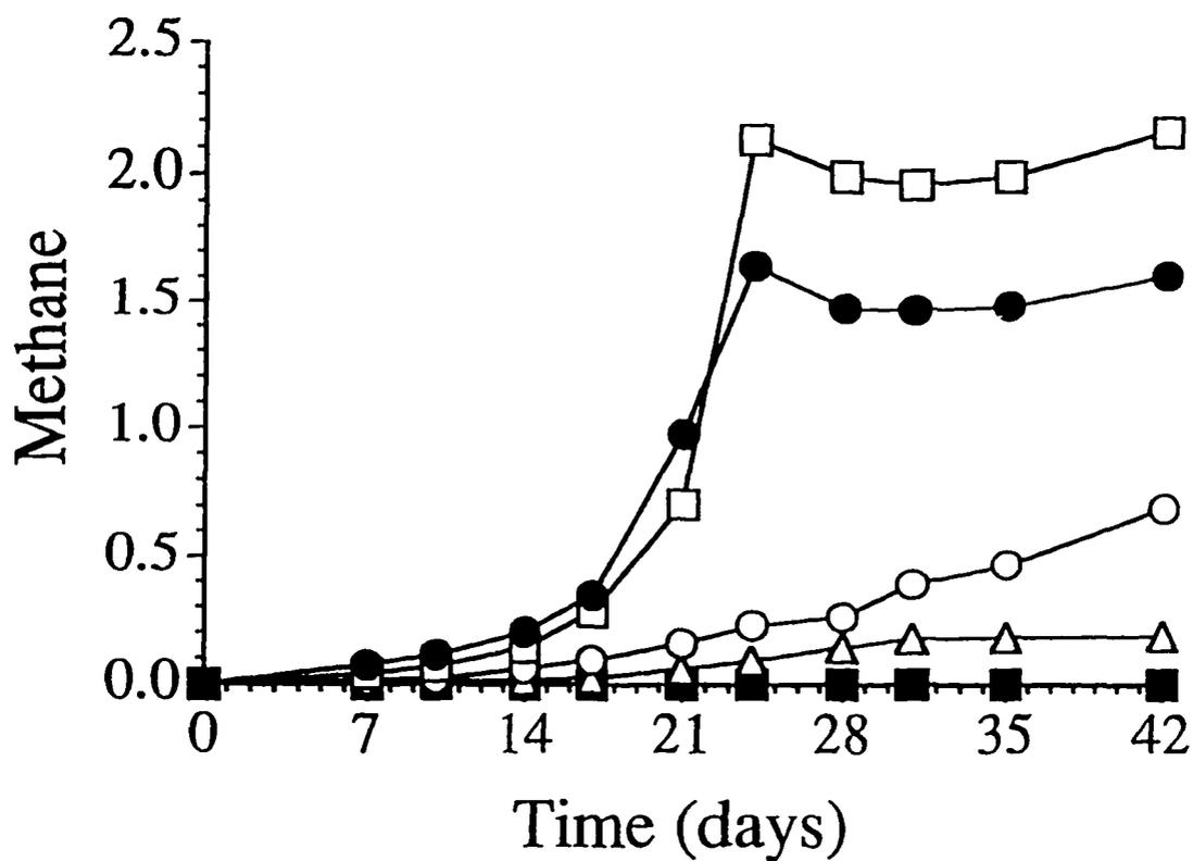
Fig. 5: Effects of aromatic sulfides on methanogenesis in anaerobic cultures established with oily sludge inoculum and lactate as a substrate. Compared to positive controls without sulfides (●), the addition of 1 mmol/L of each compound (□) increased methanogenesis, yet addition of 5 mmol/L (○), or 10 mmol/L (Δ) decreased methanogenesis, and there was no methanogenesis in sterile controls (■).
