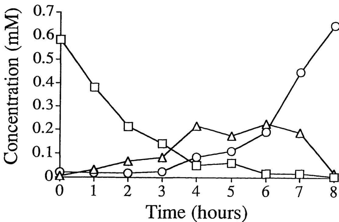
Figure 1: 2,6-Dinitrotoluene transformation in assays with cell-free extracts of *D. tiedjei*. Depletion of 2,6-dinitrotoluene (□) was followed by transient appearance of 2-amino-6-nitrotoluene (Δ) and eventual accumulation of 2,6-diaminotoluene (○).
