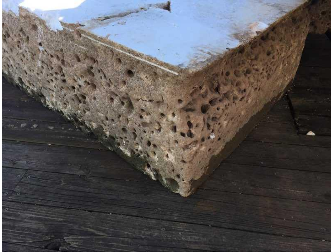
Figure 2: Photograph of a Styrofoam dock float from Lake Texoma, courtesy of Tom Wooten, owner of Buncombe Creek Marina. The holes are Harris mud crab burrows.
