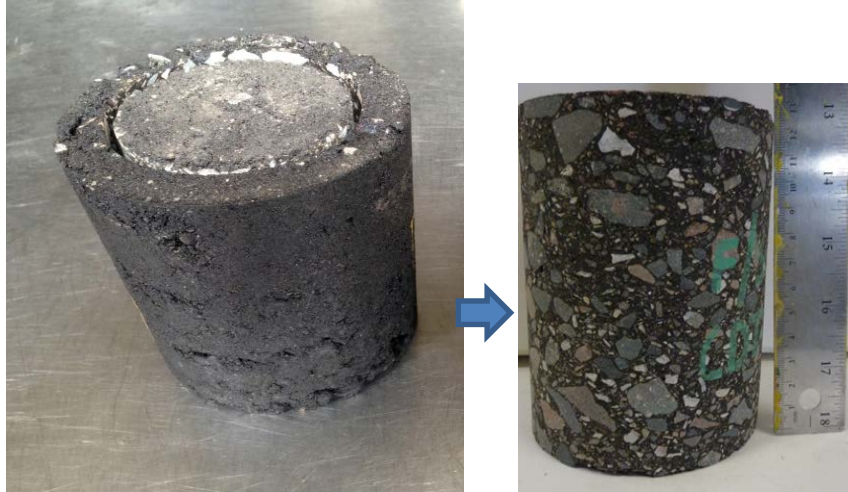
Figure 31. CDT test specimen preparation.
