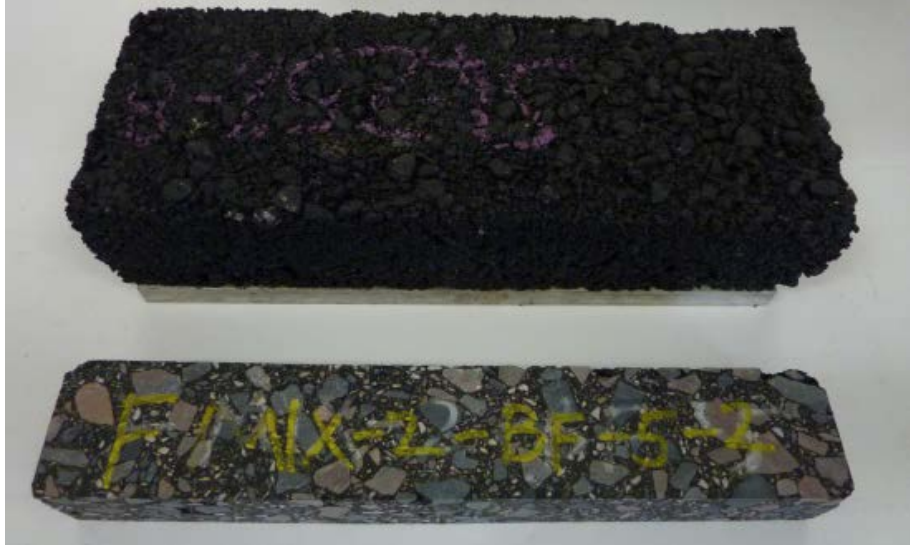
Figure 29. Beam Fatigue test specimen preparation.
