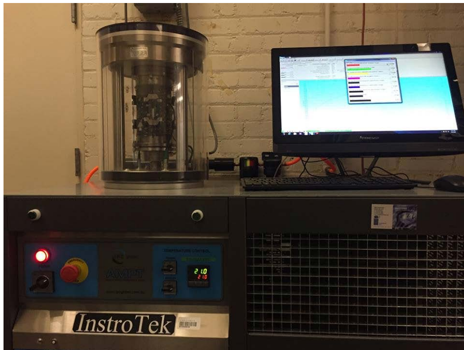
Figure 63: Newly purchased AMPT for conducting fatigue tests.
