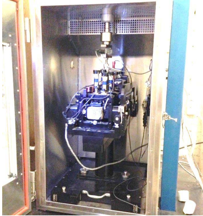
Figure 4: Four-point beam fatigue (BF) test setup.
