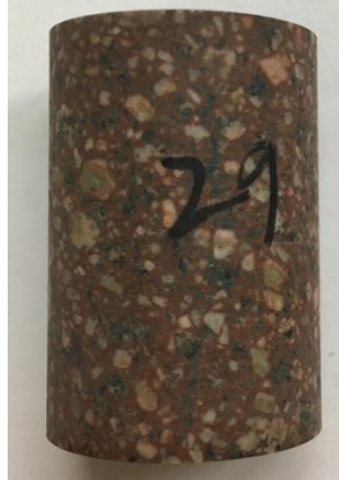
Figure 35. Plug #29 from the Washington Volcanic Group at a depth of 3056.35 ft
