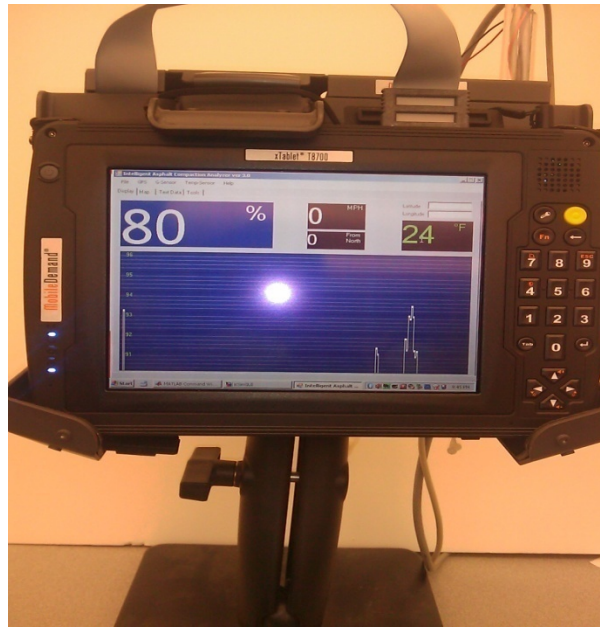
Figure 1. T8700 Rugged Tablet PC with integrated numeric keypad (shown on mounting platform)
