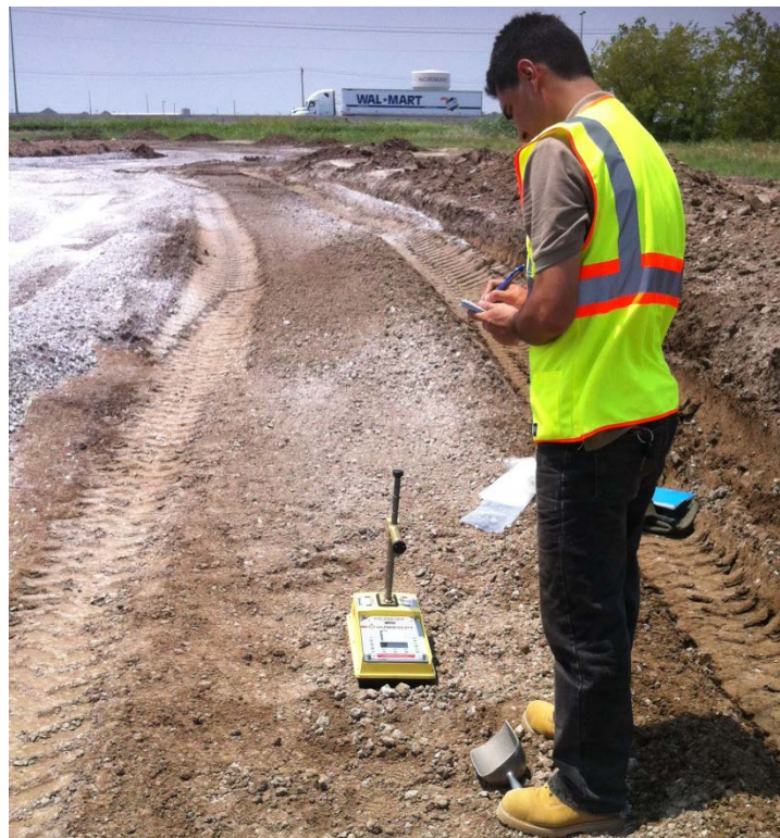
Figure 6.5. Measurement of moisture content and dry density during pre-treatment of existing soil with lime at the I-35 Service Road project.
