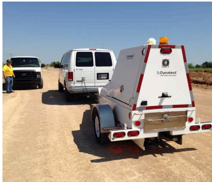
Figure 6.17. FWD test on the compacted subgrade at the I-35 Service Road project.
