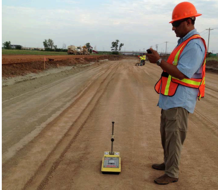
Figure 6.10. NDG measurements on compacted subgrade at the I-35 Service Road project.
