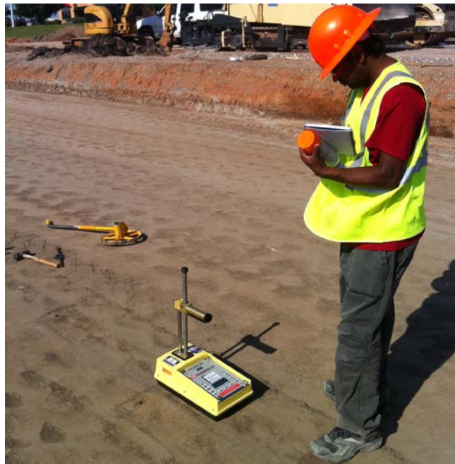
Figure 5.7. Moisture content and dry density measurements with NDG test.
