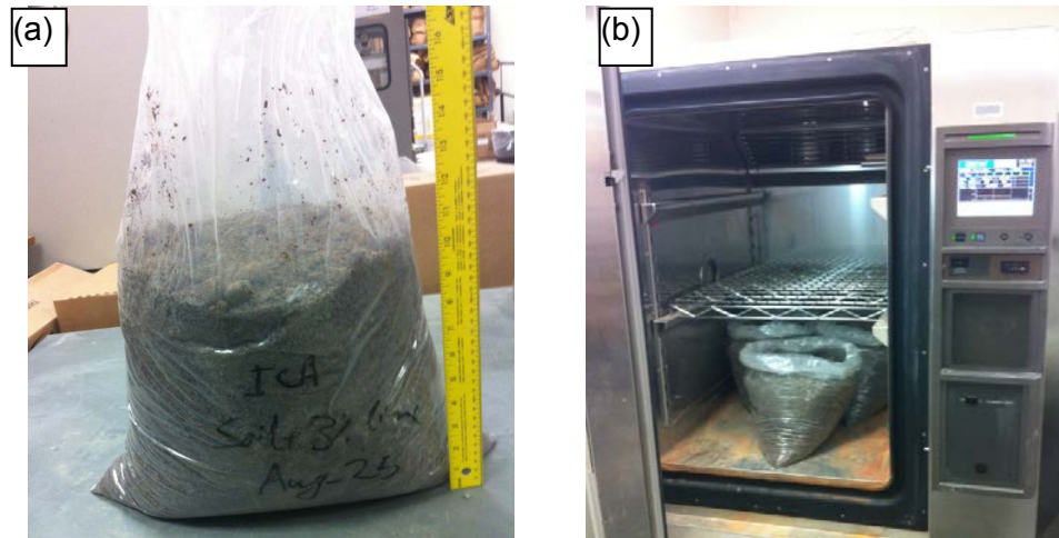
Figure 6.6. Conditioning of soil-lime mix in the laboratory.
