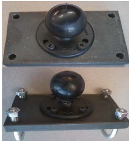
Figure 6. Bracket used to attach the Tablet PC platform to the rail on the roller
