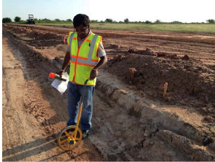
Figure 6.18. Evidence of water run-off on the compacted subgrade before the FWD test.
