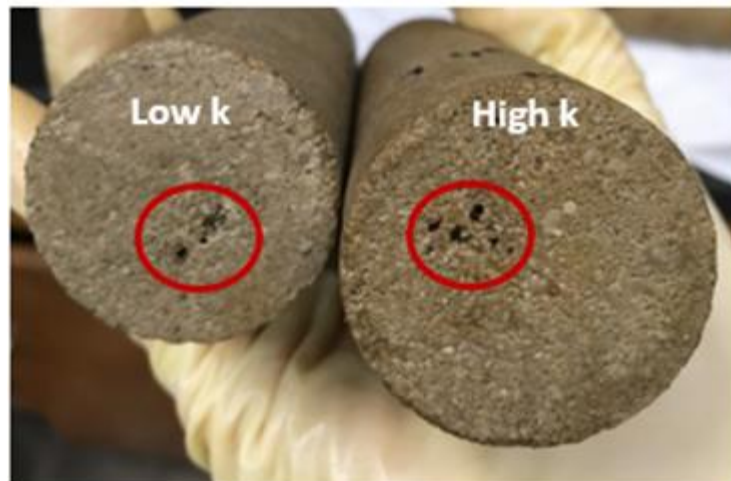
Fig 6-15 Core images for Test P3 with 1.25 vol% Si + 9% MgCl 2 + 15% HCl at 90° C
