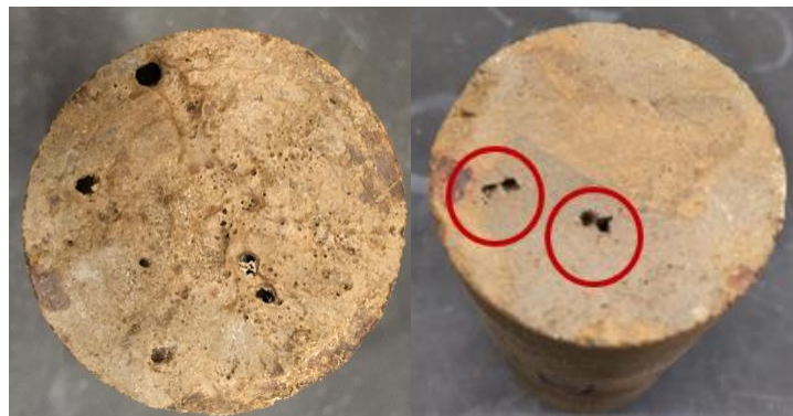
Fig 6-11 Core inlet(left) and outlet(right) images for Test S7 with 1.25 vol% Si + 9% MgCl 2 + 15% HCl
