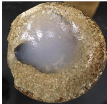
Fig 5-12 Gelation in the core
