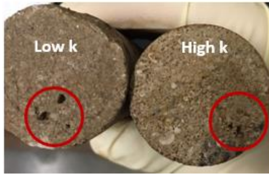
Fig 6-9 Core images for Test S3 and S4 with 1.25 vol% Si + 9% MgCl 2 + 15% HCl
