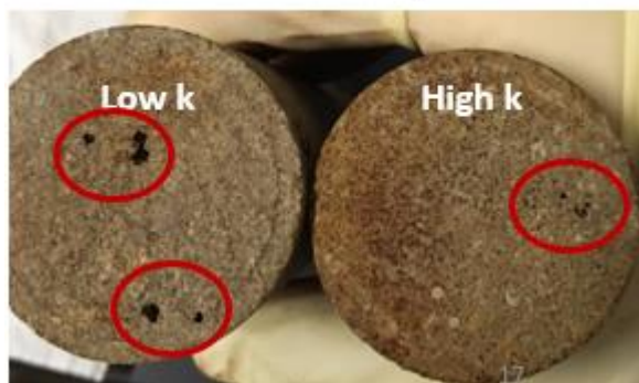
Fig 6-10 Core images for Test S5 and S6 with 1.25 vol% Si + 9% MgCl 2 + 15% HCl
