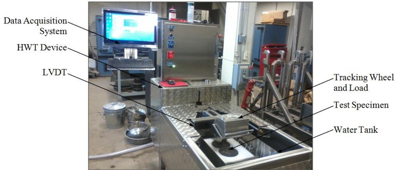
Figure 13: Hamburg Wheel Tracking (HWT) Testing Device
