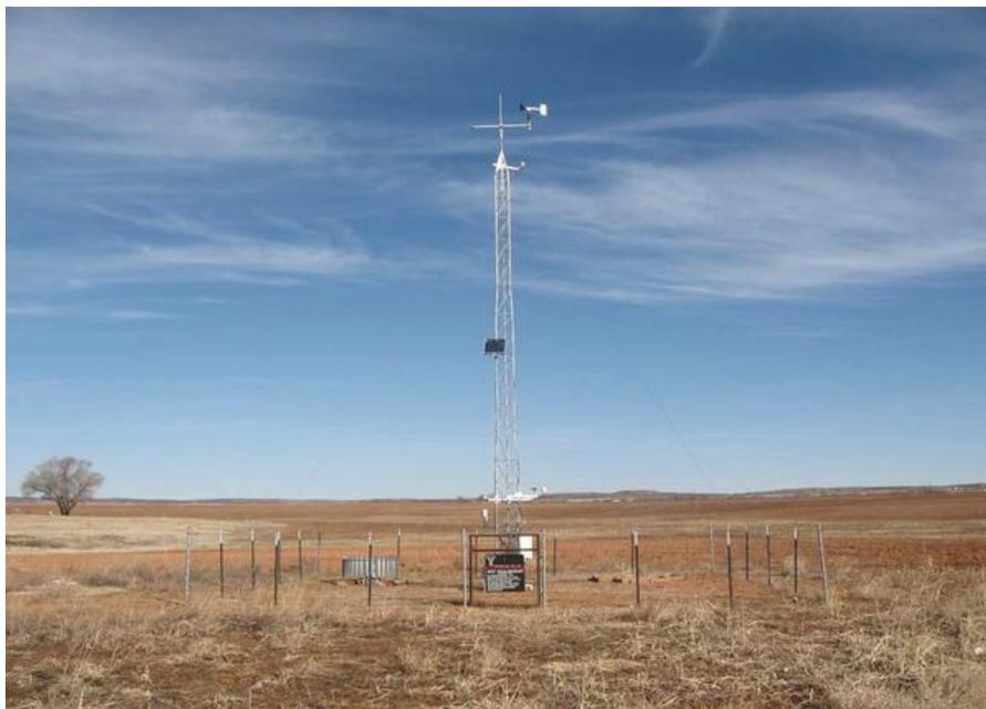
**Figure 1 A Standard Mesonet Station (from Mesonet website)**
