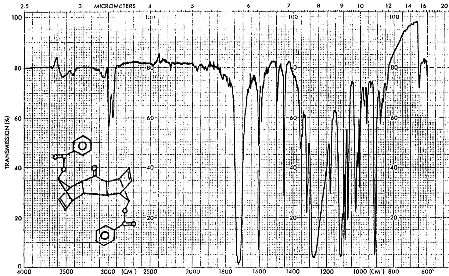
Figure IV-18. IR Spectrum of SNTNS Benzoyloxy Dimer Ketone XXXII (CHCl<sub>3</sub>).
