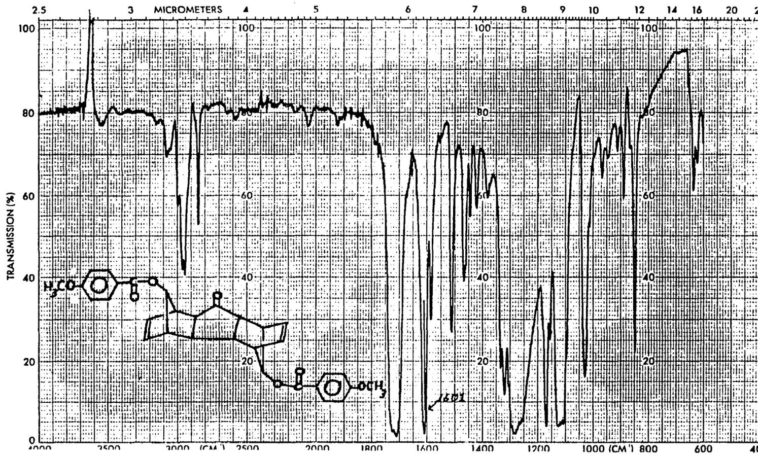
Figure IV-49. IR Spectrum of AXTA *p*-Anisoyloxy Dimer Ketone XVIII (CHCl<sub>3</sub>/TMS).
