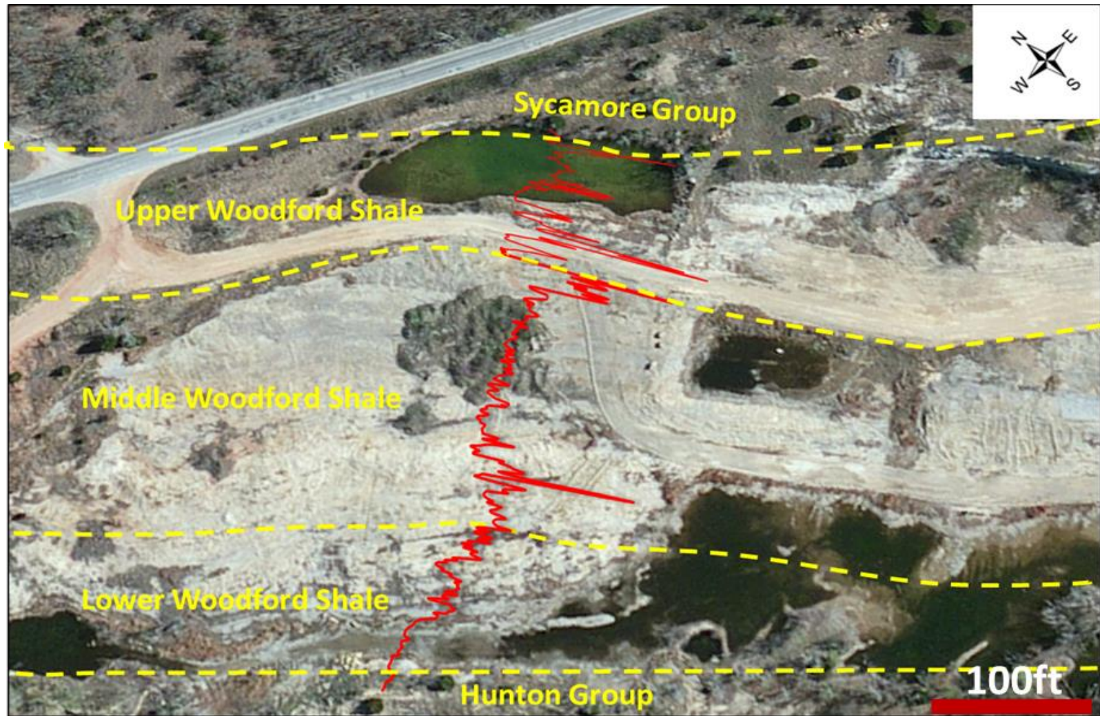
Figure 25. Woodford Shale outcrop at the McAlister Cemetery Quarry, with GR superimposed, marking the boundaries of the informal members of the Woodford Shale.
