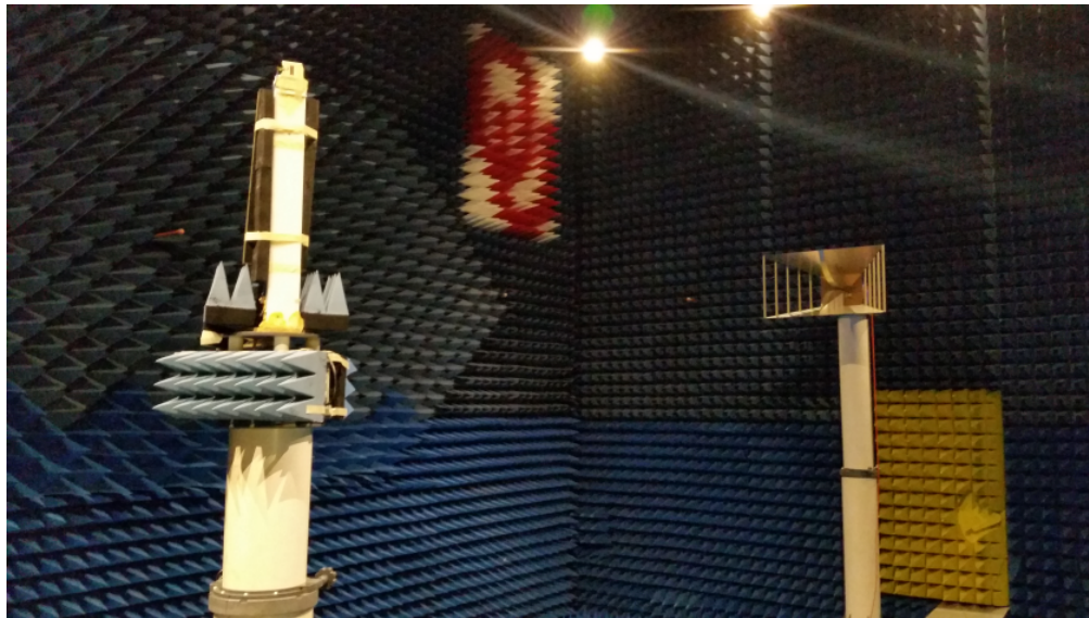
Figure 4.24: Filtenna mounted on antenna positioner in the anechoic chamber
