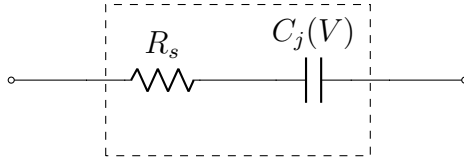
Figure 3.3: Series RC varactor model used in HFSS
