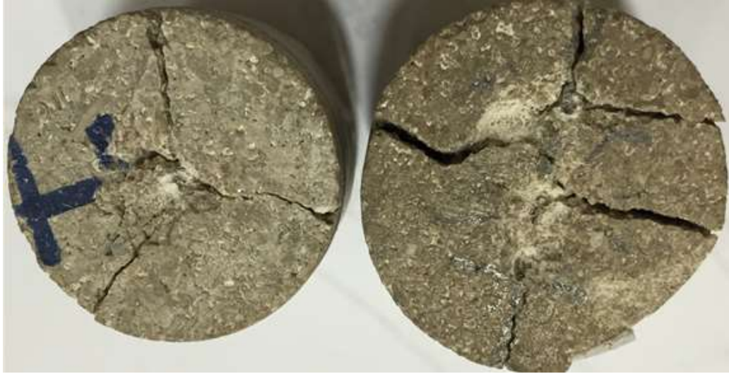
Figure 2.14 Indented semi-circular cylinders of Limestone, note the fractures are more tortuous than Grey Berea Sandstone, and the near crater chipping is significant
