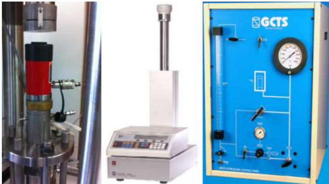
Figure 4.3 Hydraulic cylinder and Teledyne ISCO pump for applying axial load and GCTS pressure booster (HPC-070) for applying confining pressure
