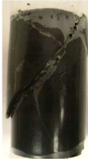
Figure 4.35 Macroscopic fractures induced by creep failure, Haynesville 07-11
