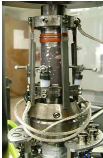
Figure 5.13 Sample (fractured tuff) assemble ready for multistage triaxial joint shear test
