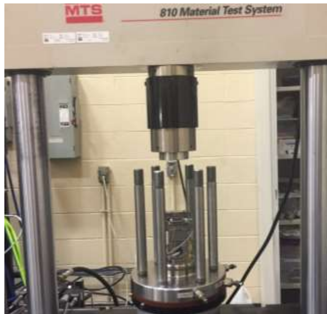
Figure 3.5 MTS 810 frame and GCTS triaxial cell with internal S-shaped load cell and Brazilian specimen assembly
