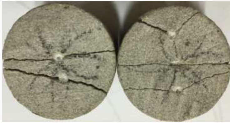
Figure 2.11 Indented semi-circular cylinder of Grey Berea Sandstone, note the fractures are more planner than that of Limestone
