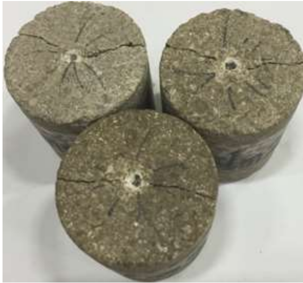
Figure 2.8 Indented Indiana Limestone cylinders, note the chipped area around the crater
