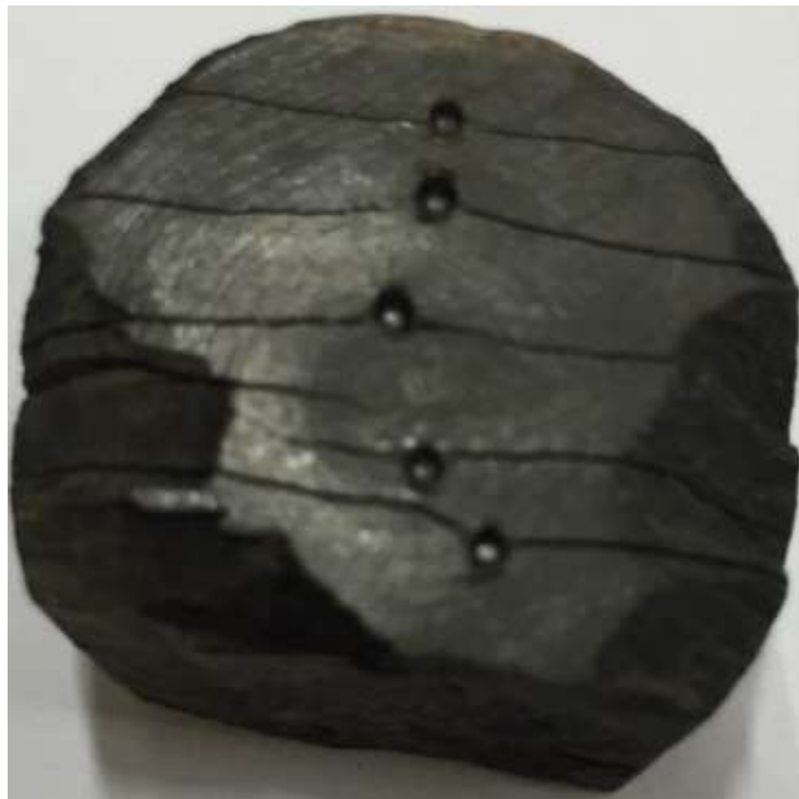
Figure 2.16 Indented Marcellus shale disc, note the fractures are very planar and parallel with the bedding plane
