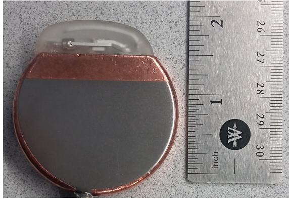
Figure 5.15: Fabricated implantable device with the straight vertical antenna. A coaxial cable for the antenna measurement is inserted to the can at the bottom.
