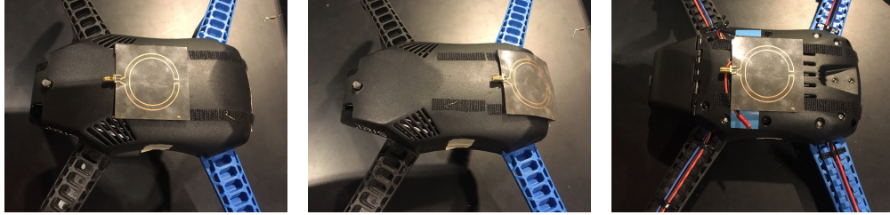
Figure 4.16: Conformally mounted 20MHz bandwidth CFDA variation in the top (left), rear (middle), and bottom (right) positions as mentioned
