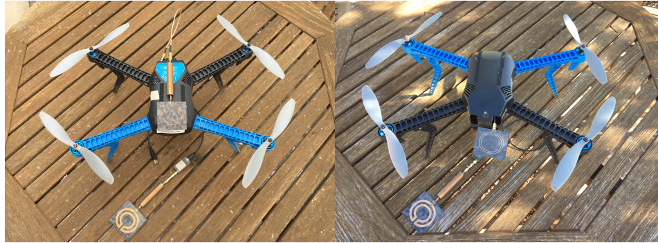
Figure 5.5: Example antenna configurations for base station telemetry module and for IRIS aircraft with both conformal (left) and non-conformal (right) positioning on the aircraft
