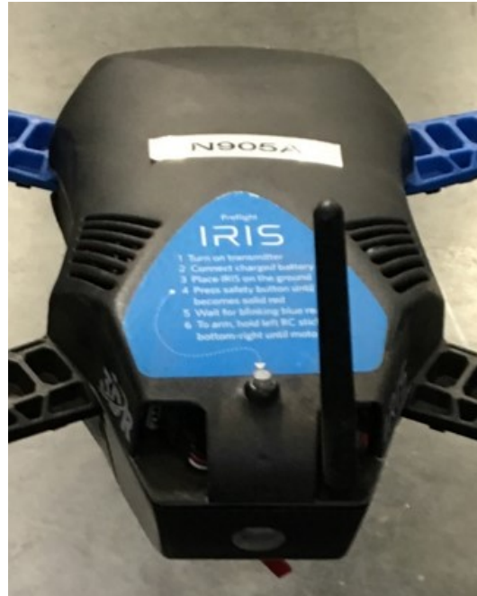
Figure 1.1: Antenna configuration of the included coiled monopole rubber duck antenna on the IRIS craft used as an antenna test platform
