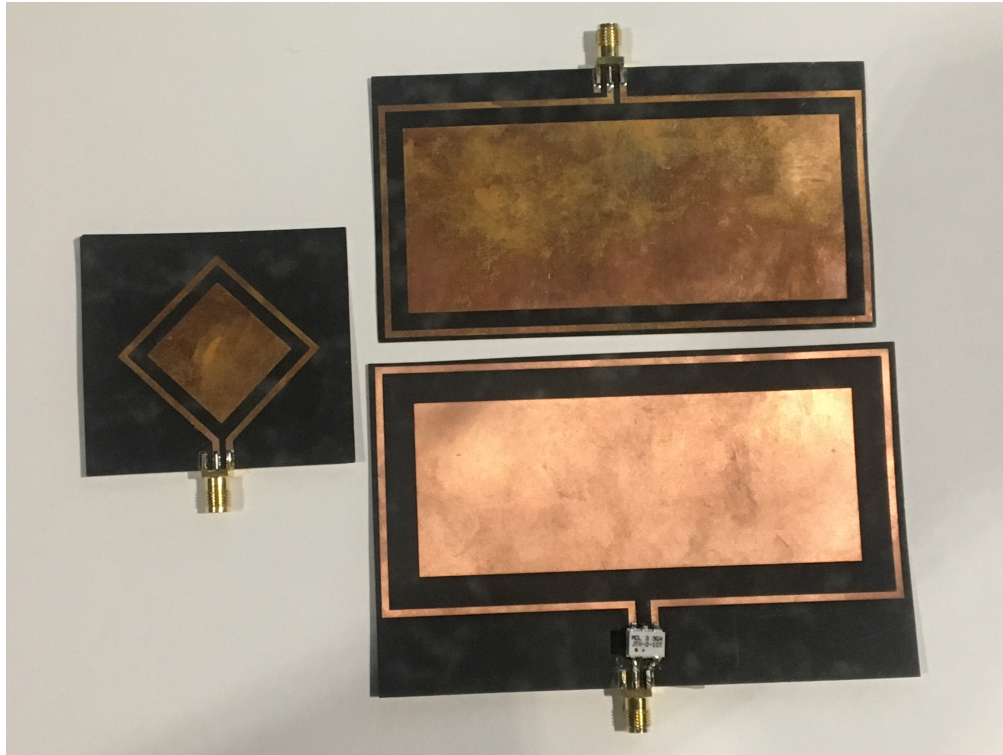
Figure 3.3: Fabricated Loop antennas: 2.4 GHz 50 \Omega diamond loop (left), 915 MHz 50 \Omega rectangular loop (top), and 915 MHz 100 \Omega rectangular loop with 2:1 chip balun (bottom)
