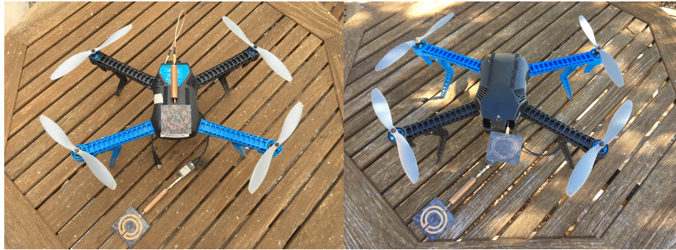
Figure 5.2: Quadrotor test configuration for antennas in both conformal (left) and non-conformal (right) configurations on the IRIS aircraft
