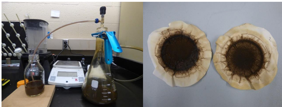
Figure 16: Asphaltene content measurement setup. The filter paper is placed on top of the conical flask.
