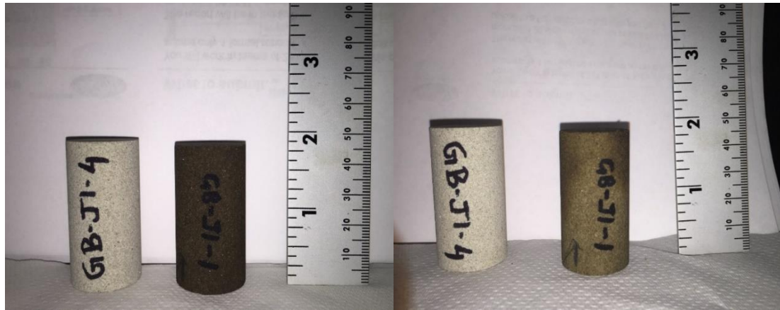
Figure 28: Cores after crude injection (left) and after heptane flush (right). The darker tones of the cores indicate the presence of crude residue, even after heptane flush.
