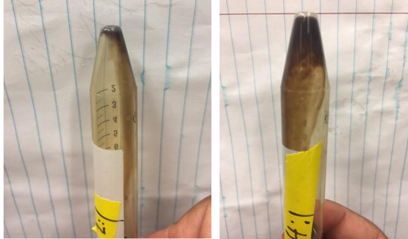
Figure 26: Asphaltene precipitation after bottle tests. More precipitation is noted in case of crude mixed with heptane in 1:4 ratio
