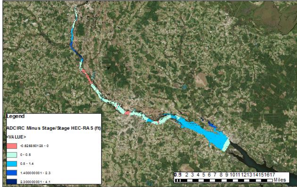
Figure 7-16 ADCIRC inundation depth minus HEC-RAS Stage/Stage Inundation Depth. Pink indicates HEC-RAS results above ADCIRC results. Darkening shades of blue indicate ADCIRC results above HEC-RAS results.
