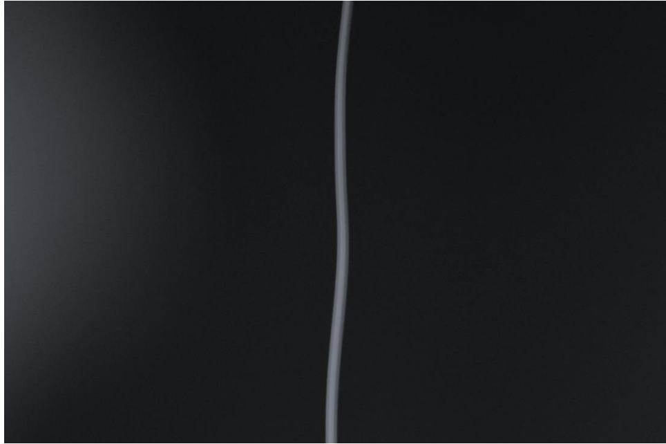
Fig. V.5. Online image of a melt blown fiber taken with a Nikon 3200D camera. The camera had a 1/4000 second shutter speed and a f-stop of 6.3 (large aperture).
