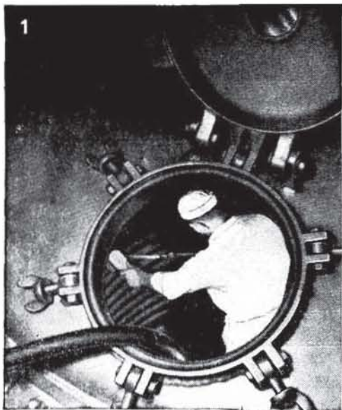
(1) One of many 3000-gallon converters in which Dextri-Maltose is processed. Interior being thoroughly cleansed by hand prior to steam sterilization.
