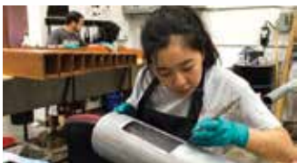
Mayu Allen ('14), a graduate of the AOI's organ technology program, restoring a tuba pipe.
