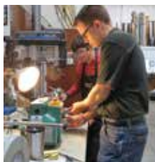
John Riester works with Nathan Rau to machine new brass weights for reed tongues.
