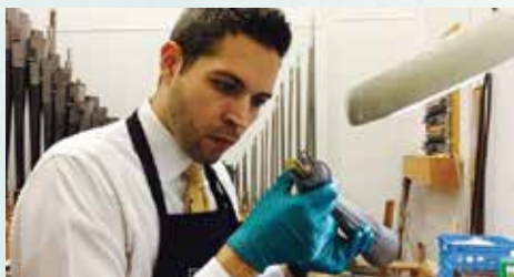
Adam Pajan inspecting the tongue and shallot of a pipe from the WKY tuba rank.
