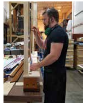
Paul Watkins builds racking to support one of the reed ranks in the WKY Kilgen.
