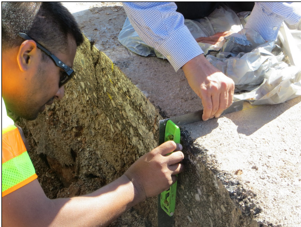
Figure 7.11: Depth Measurements of Different Layers
