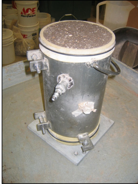
Figure 4.12 Compacted Resilient Modulus Specimen of Aggregate Base
