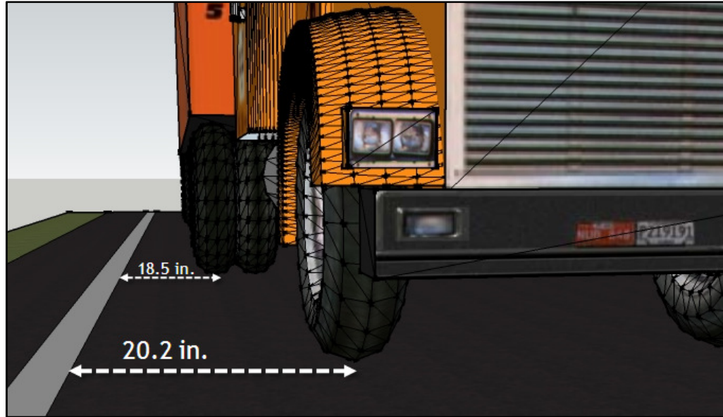
Figure 4.5: Distances Used in Calculating Wheel Wander
