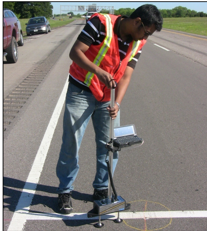
Figure 3.9: Rut Measurements with Face Dipstick® (Hossain et al., 2010)
