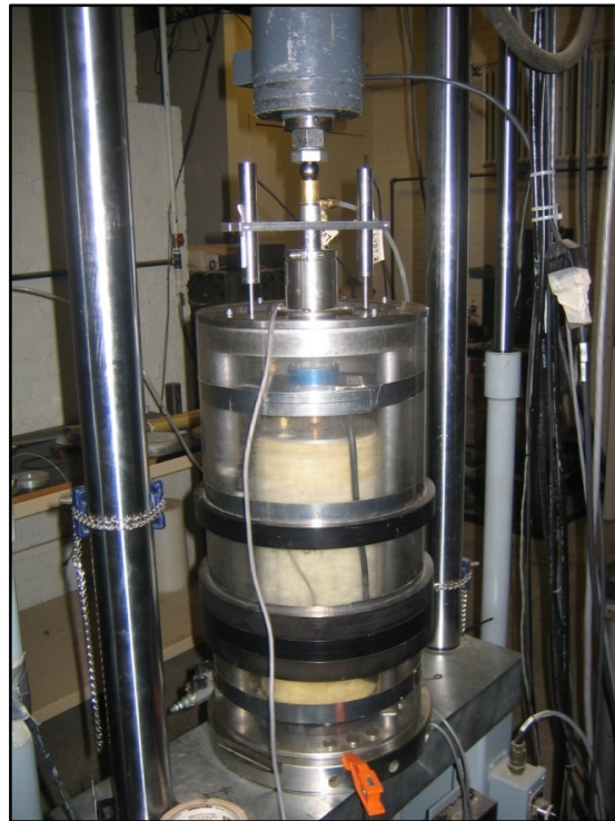
Figure 4.13: Setup for Resilient Modulus Testing on Aggregate Base Specimen
