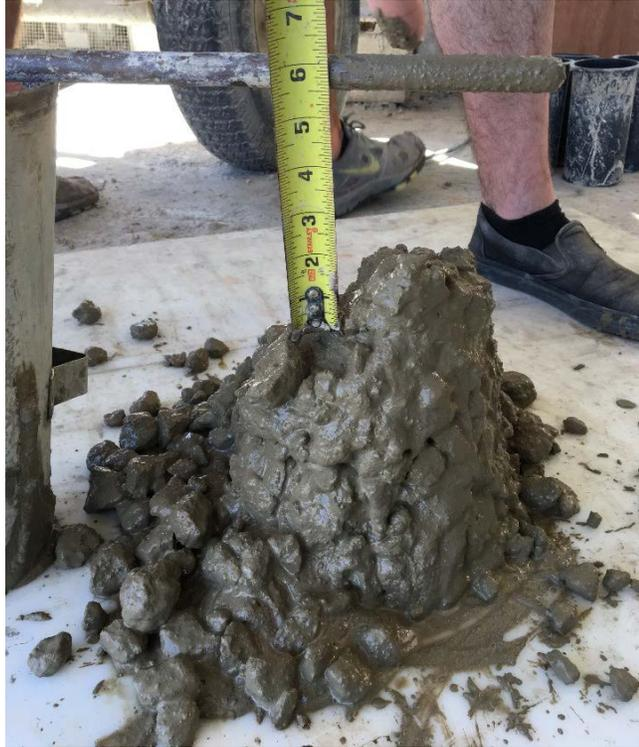
***Figure 4.8 1-50 Slump Reading***
