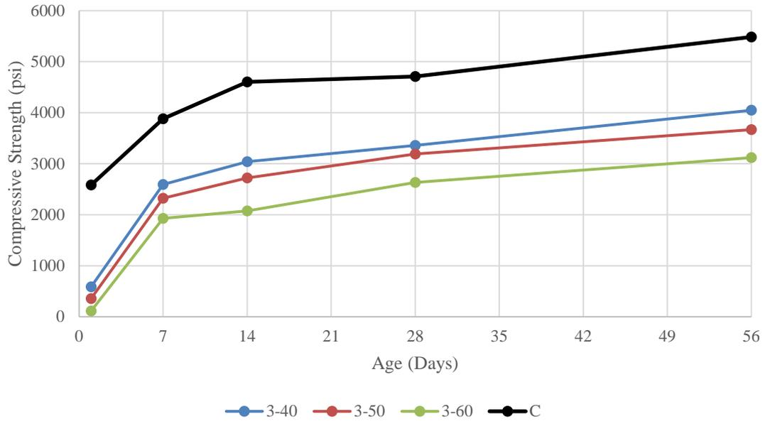
**Figure 4.23 Series No. 3 & C Control Compressive Strength vs. Time**
