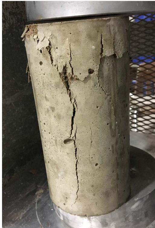
**Figure 4.20 3-60 28-Day Specimen Post-Loading**
