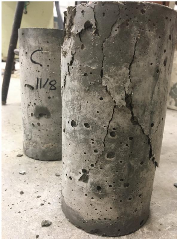
***Figure 4.6 Control 1-Day Specimen Post-Loading***
