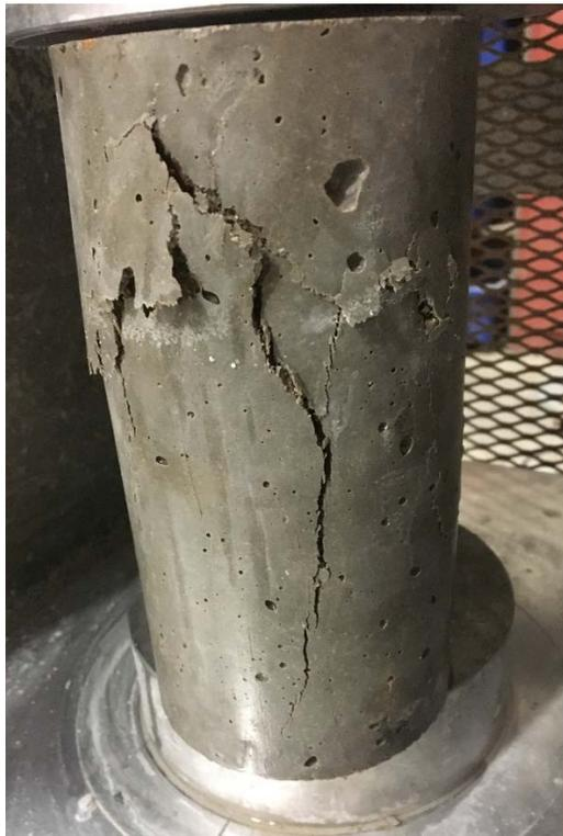
**Figure 4.12 1-50 28-Day Specimen Post-Loading**
