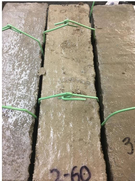
*Figure 6.5 Condition of 2-60 After 36 Cycles*
