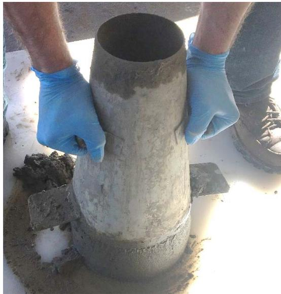
*Figure 4.2 Control Slump Reading*
