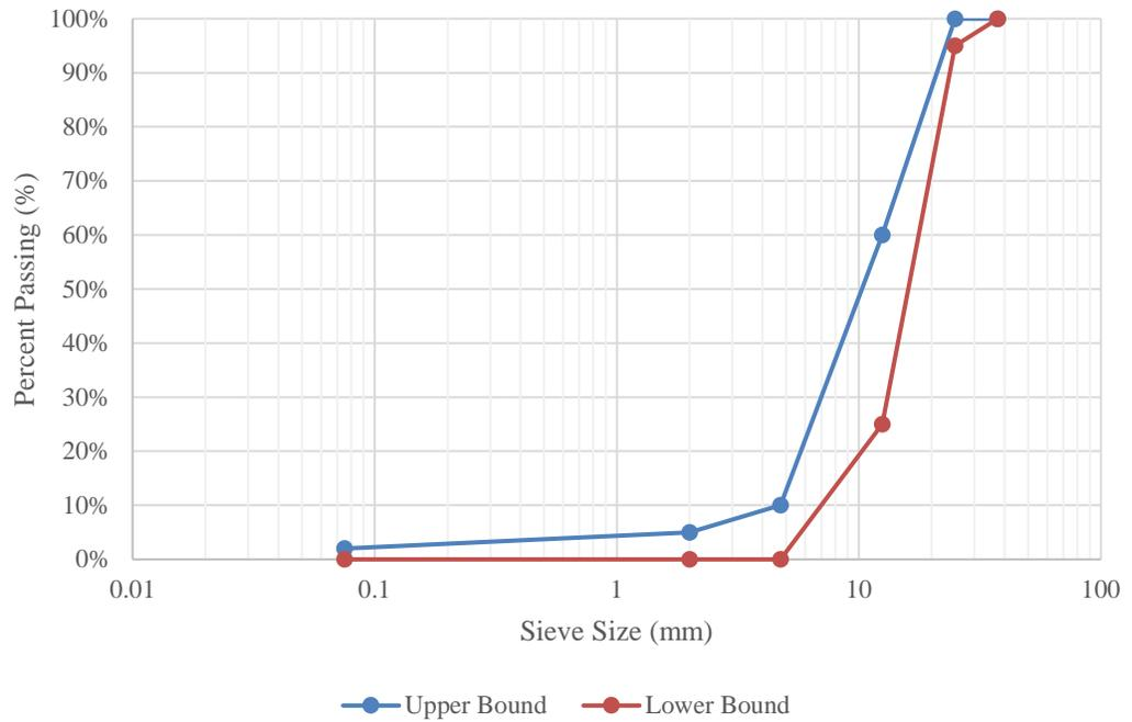
**Figure 3.1 Acceptable ODOT Coarse Aggregate Range**
