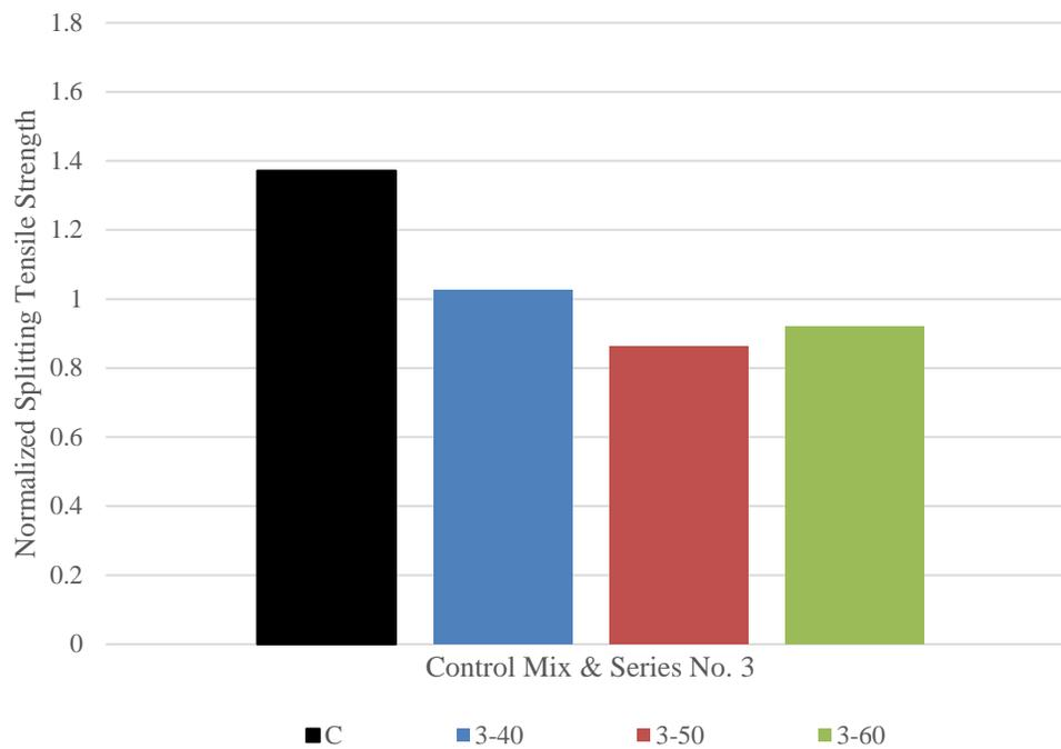
**Figure 4.32 Normalized Splitting Tensile Strength for Series No. 3 & Control**
