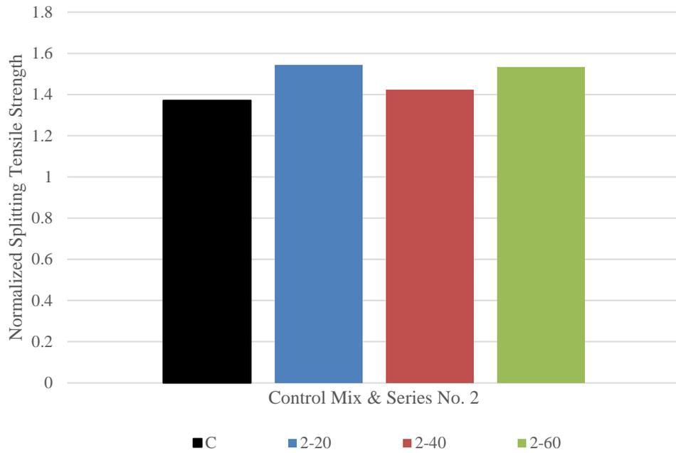
**Figure 4.31 Normalized Splitting Tensile Strength for Series No. 2 & Control**
