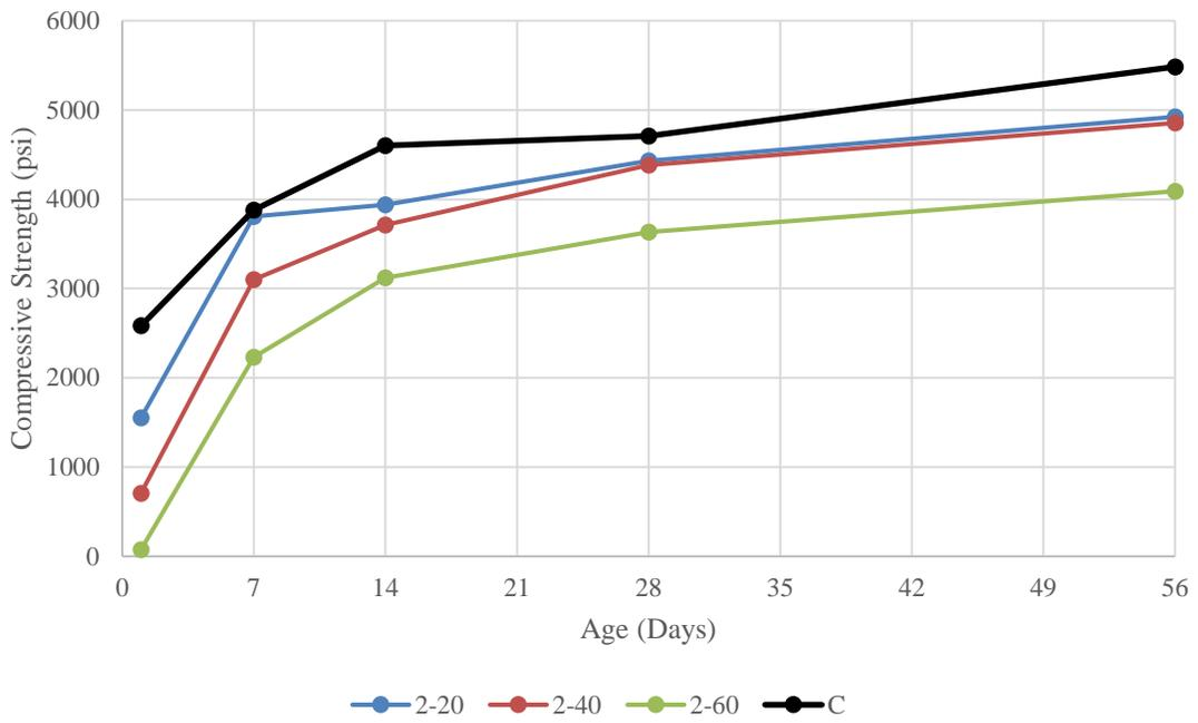
**Figure 4.22 Series No. 2 & Control Compressive Strength vs. Time**
