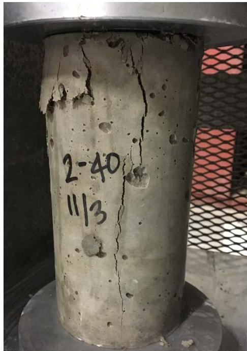
**Figure 4.18 2-40 28-Day Specimen Post-Loading**
