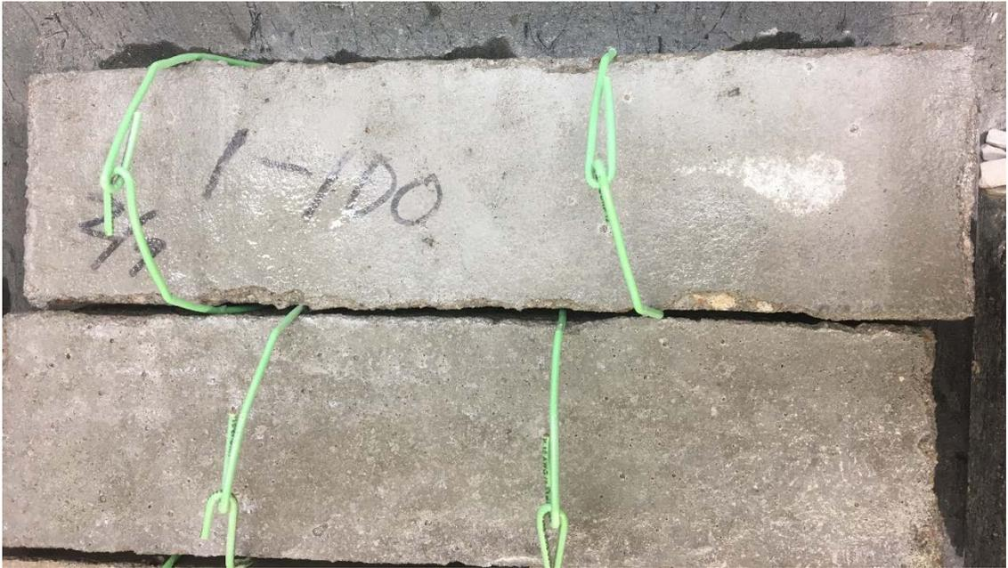
*Figure 6.6 Condition of 1-100 After 36 Cycles*
