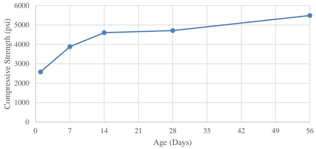
***Figure 4.5 Compressive Strength vs. Time Plot for Control Mix***
