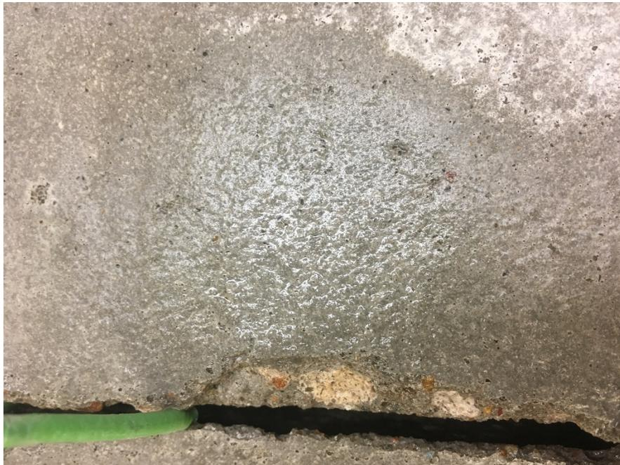
*Figure 6.7 Close-Up of 1-100 After 36 Cycles*
