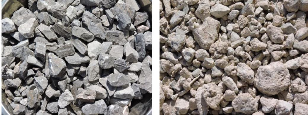
***Figure 2.3 Up-Close Comparison of Virgin Coarse Aggregate (left) and RCA (right)***
