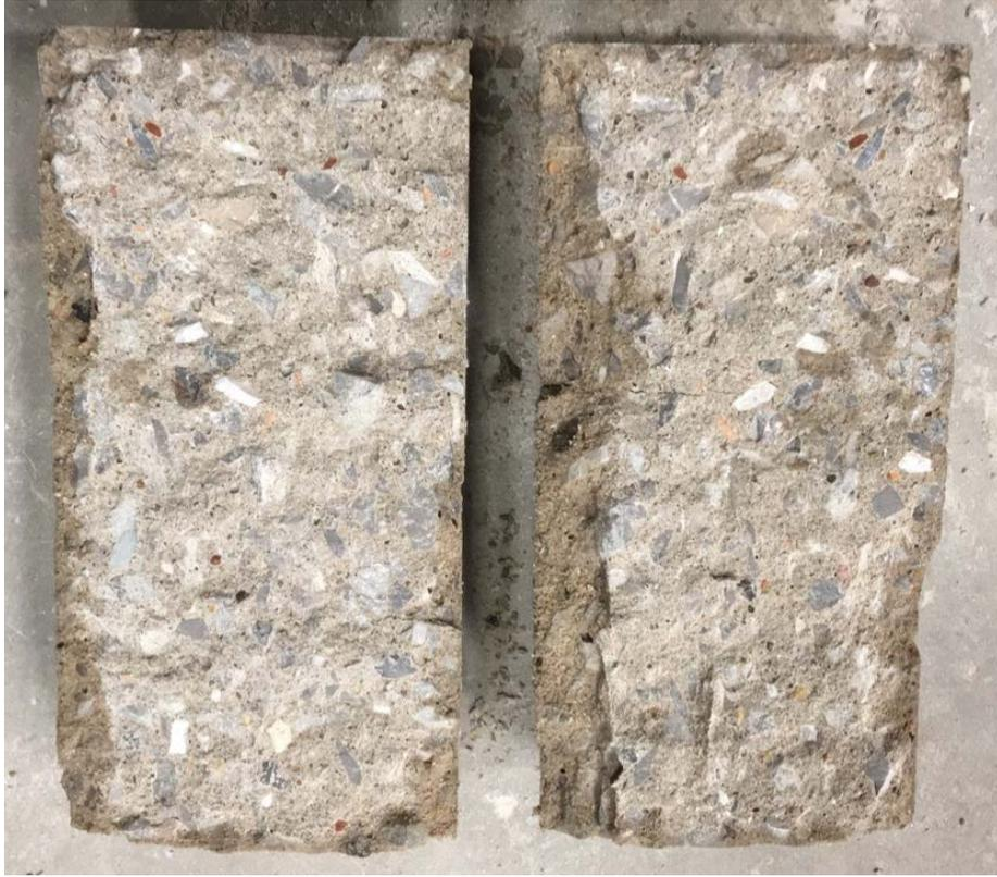
*Figure 4.16 2-40 Split Cylinder Fracture Surface*
