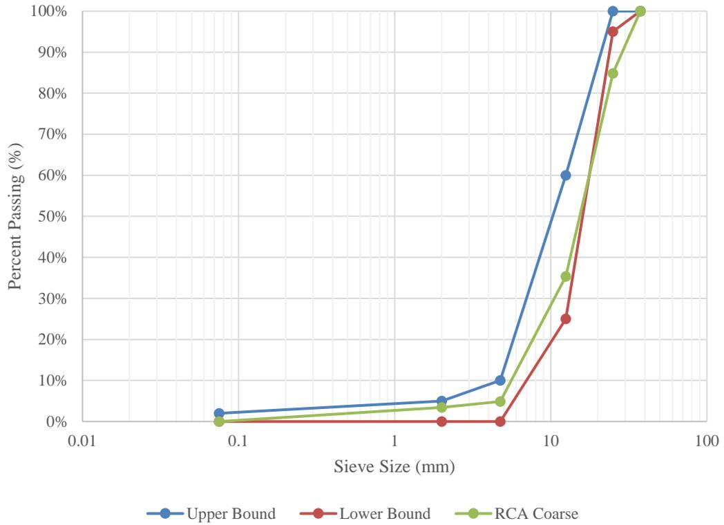
**Figure 3.5 Gradation Curve for RCA Coarse**
