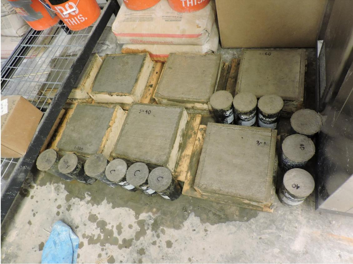
*Figure 6.15 Ponding Specimens Prior to Demolding at Age 14 Days*
