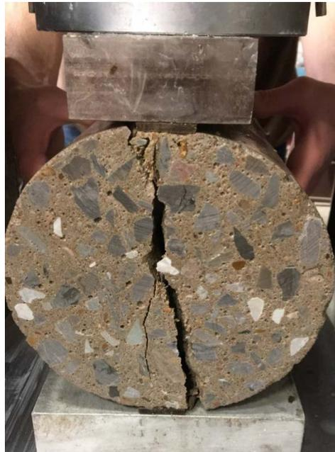
**Figure 4.15 2-40 Split Cylinder Test Post-Loading**
