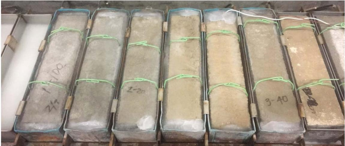
***Figure 6.3 Freeze-Thaw Specimens After 36 Cycles***
