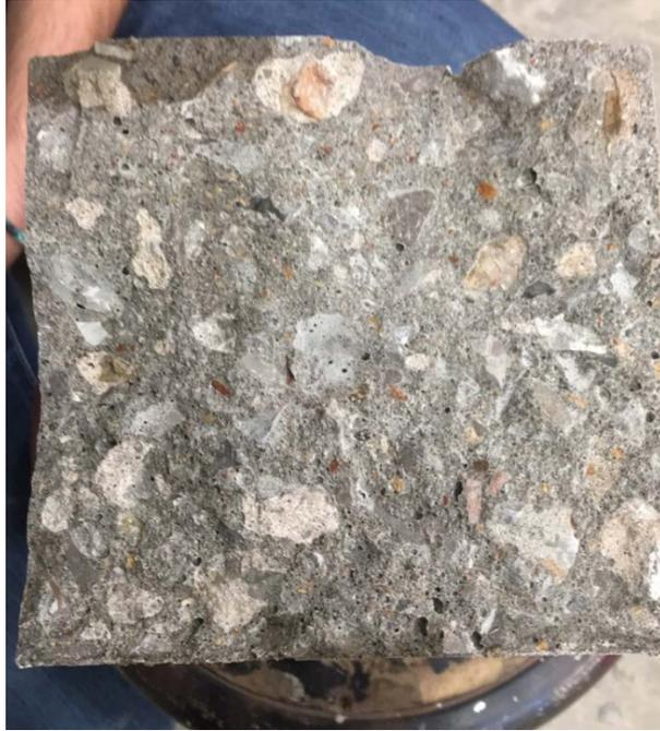
*Figure 4.9 1-50 MOR Fracture Surface*
