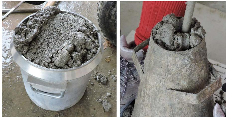
*Figure 5.2 Mix 4-15 Close-Up in Air Pot and Slump Cone*
