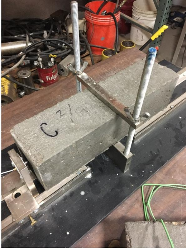
*Figure 6.1 Control Specimen in MOE Apparatus at 0 Cycles*
