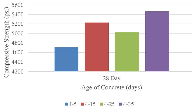
**Figure 5.6 Comparison of 28-Day Compressive Strength for Series No. 4**
