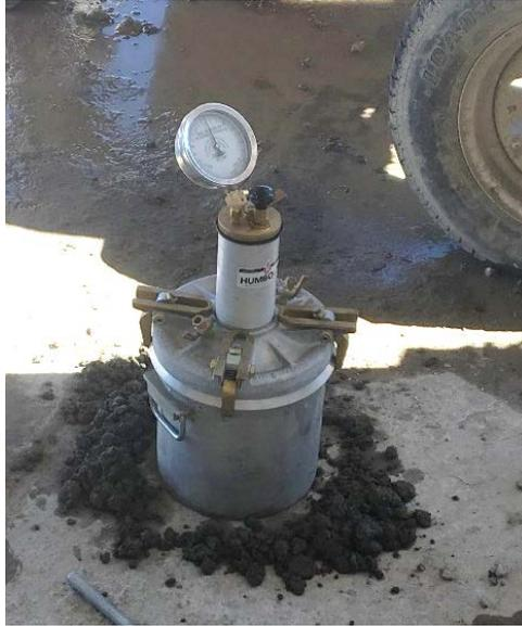
*Figure 4.1 Air Content Reading*
