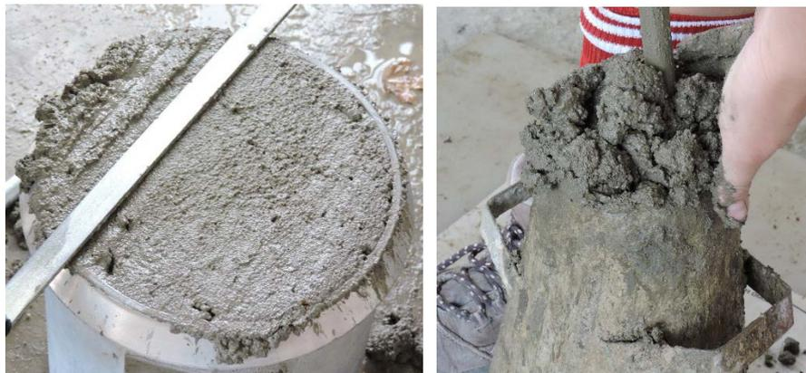
*Figure 5.3 Mix 4-25 Close-Up in Air Pot and Slump Cone*
