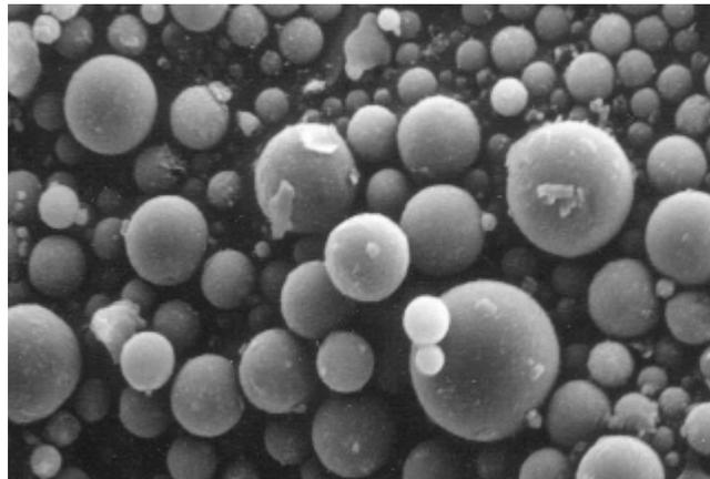
**Figure 2.4 Fly Ash Particles at 2000x Magnification (FHWA, 2001)**
