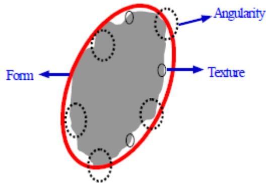
***Figure 3.7 Aggregate Shape Properties (FHWA, 2006)***
