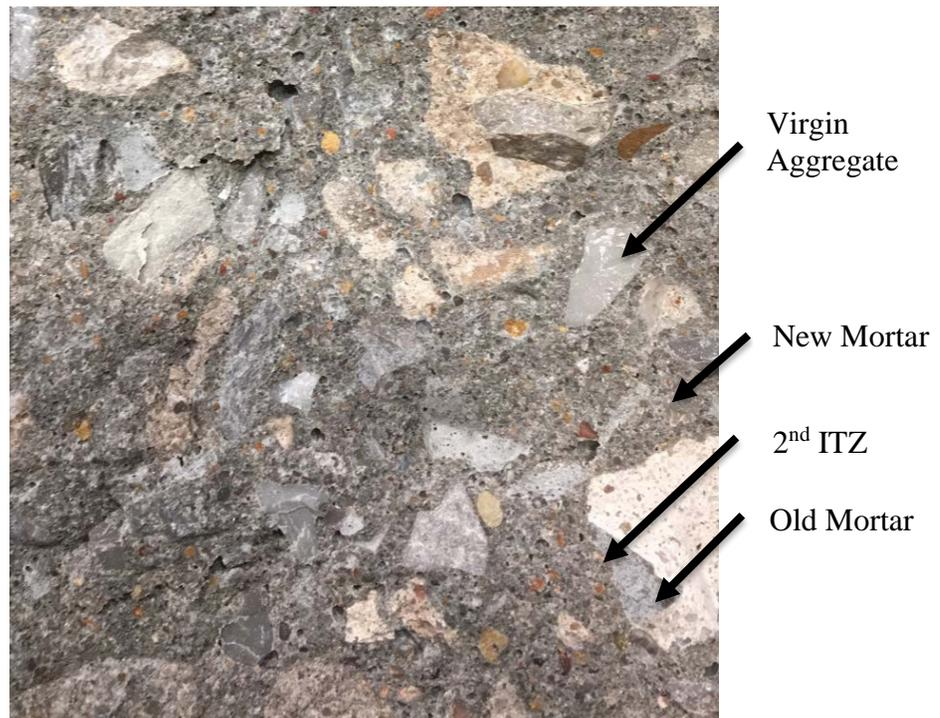
***Figure 2.2 Microstructure of RCA Concrete***
