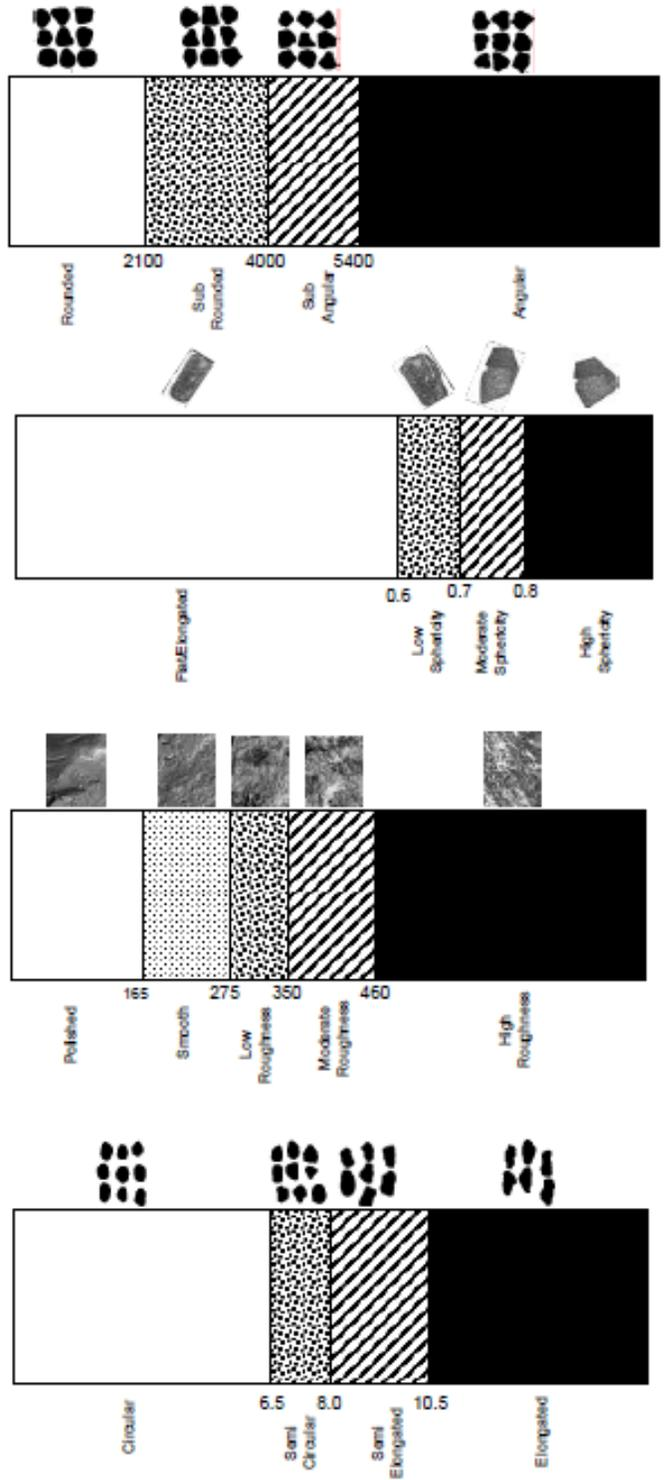
Figure 3.9 Aggregate Shape Classification Chart (FHWA, 2006)
