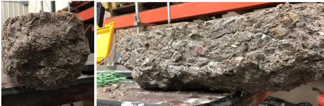
*Figure 6.9 End and Side View of Control After 300 Cycles*
