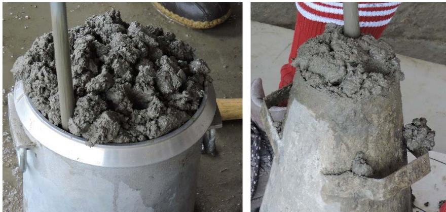
**Figure 5.4 Mix 4-35 Close-Up in Air Pot and Slump Cone**
