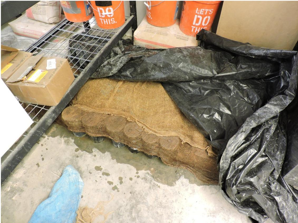
***Figure 6.14 Ponding Specimens - Moist Curing***
