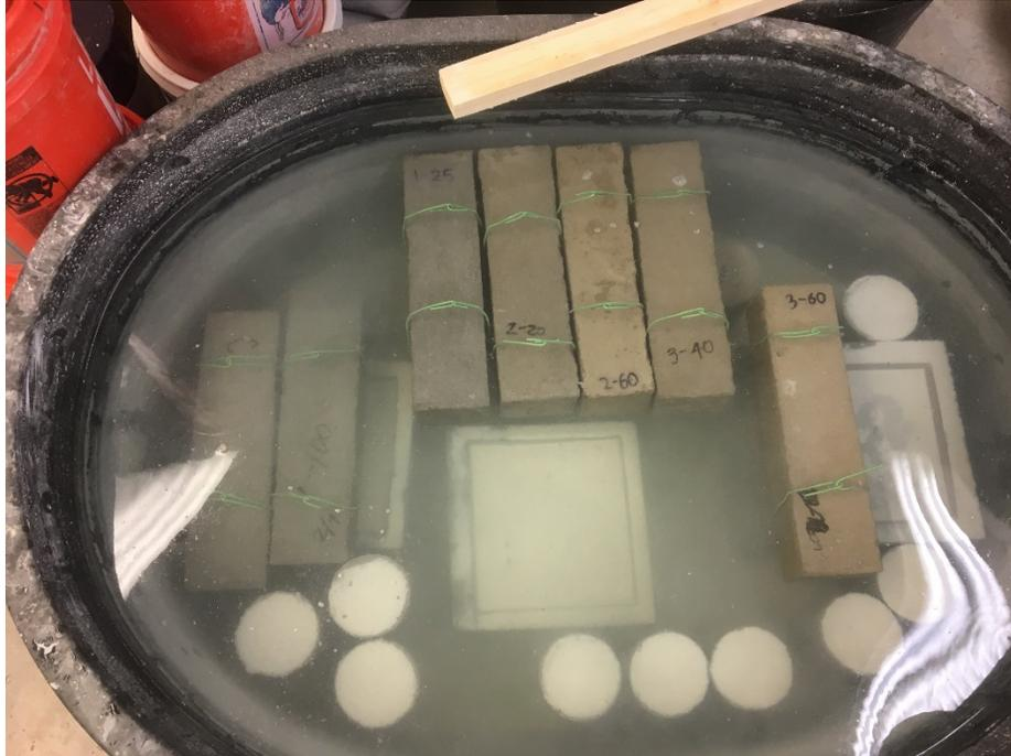
*Figure 6.4 24-Hour Soaking after 36 Cycles*
