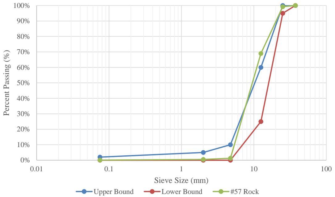
**Figure 3.3 #57 Rock Gradation with ODOT Boundaries**
