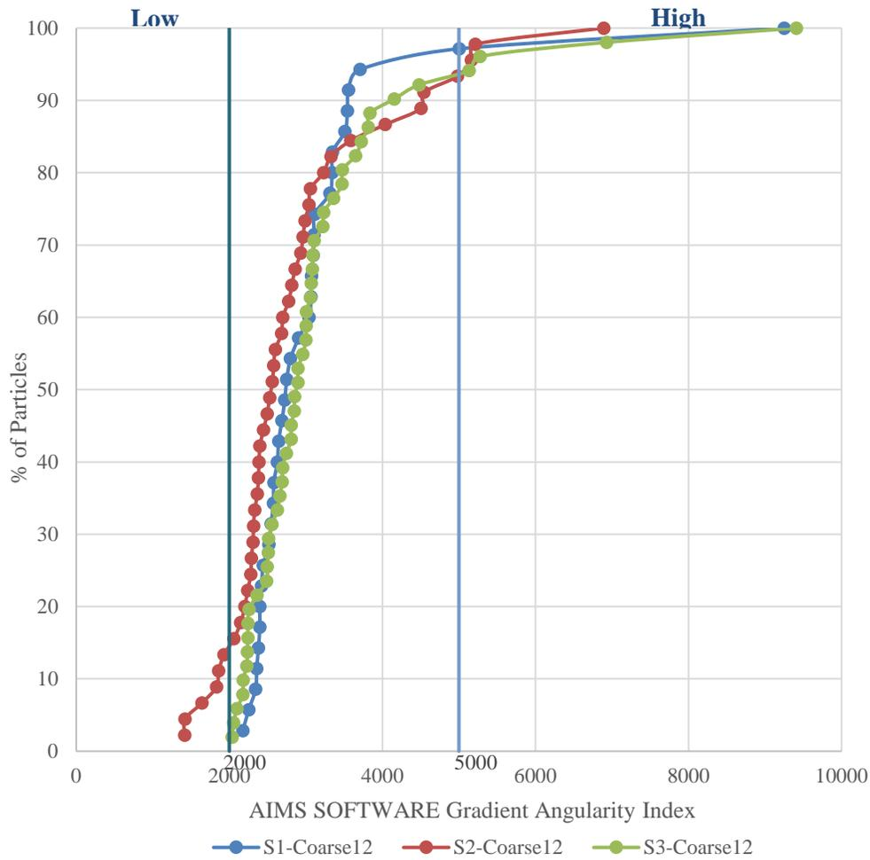
**Figure 3.12 AIMS RCA Gradient Angularity Analysis**
