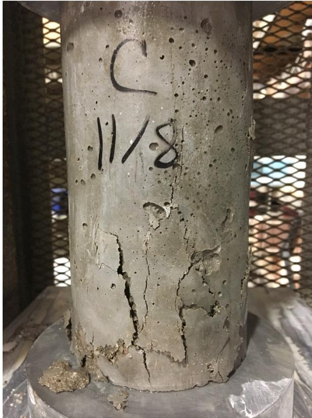
*Figure 4.7 Control 28-Day Specimen Post-Loading*
