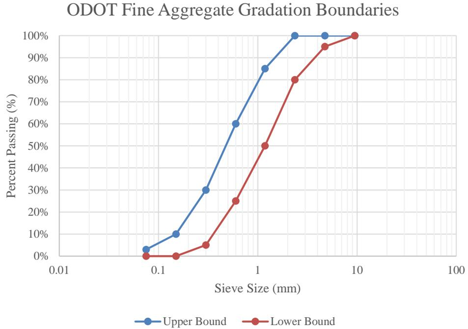
**Figure 3.2 Acceptable ODOT Fine Aggregate Range**
