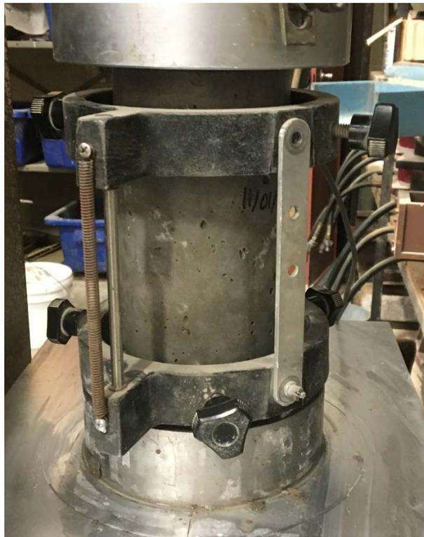
*Figure 4.10 MOE Test Apparatus*
