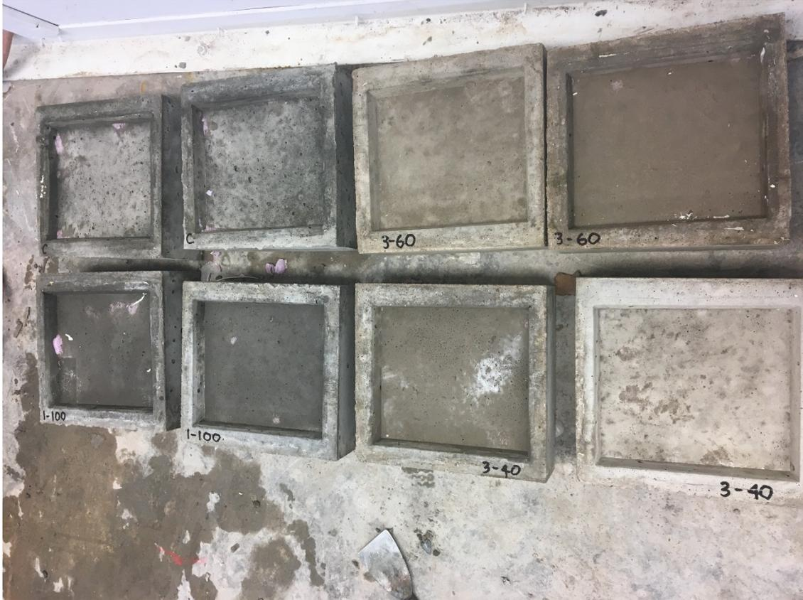
*Figure 6.16 Ponding Specimens - Air Curing*
