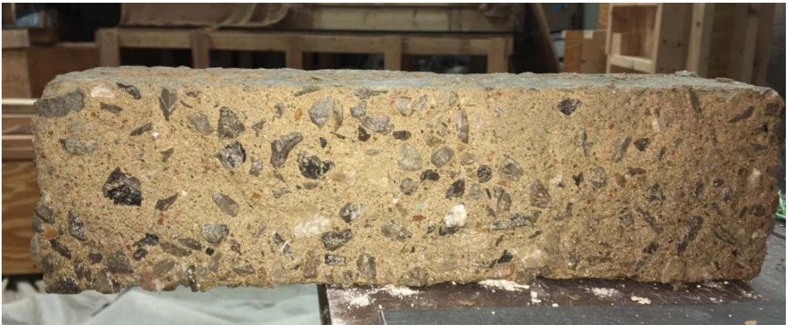
*Figure 6.11 Side View of 2-60 After 300 Cycles*
