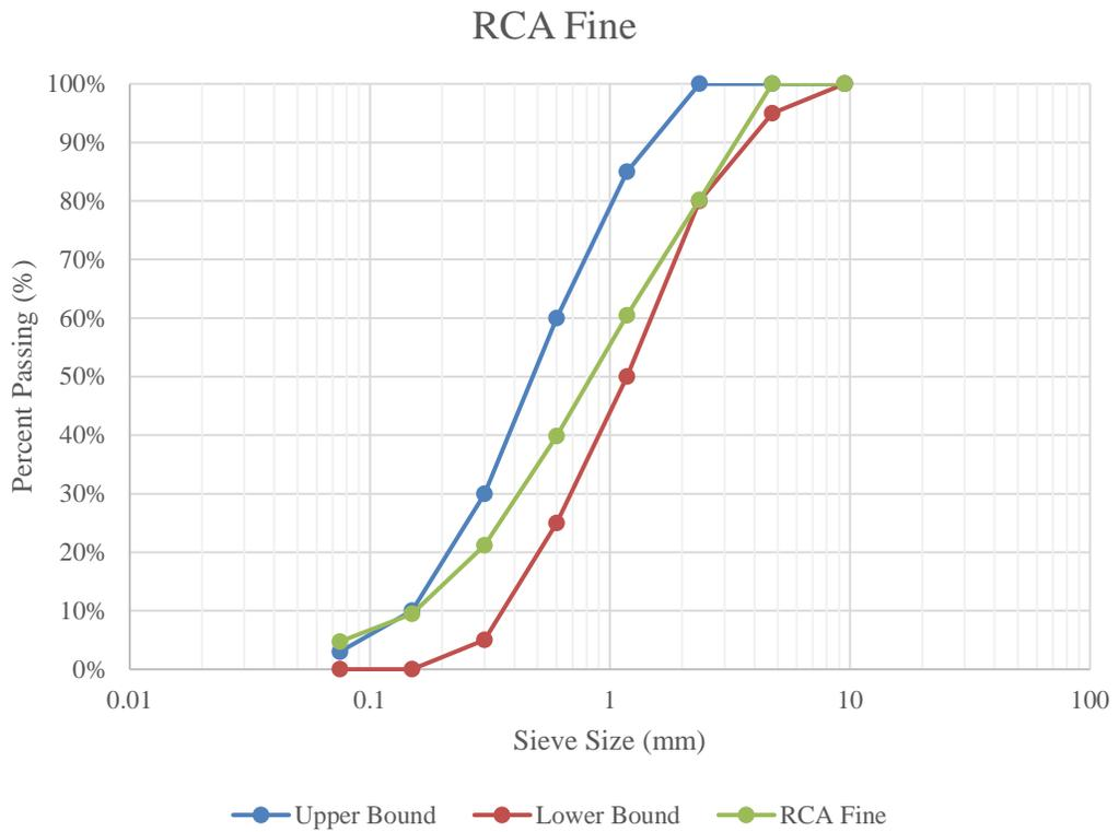
**Figure 3.6 Gradation Chart for RCA Fines**
