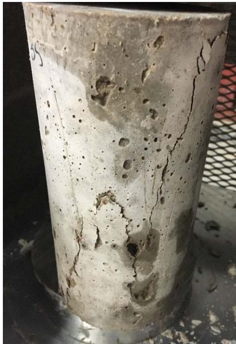
**Figure 5.5 4-35 At 28-Day Strength Post-Loading**
