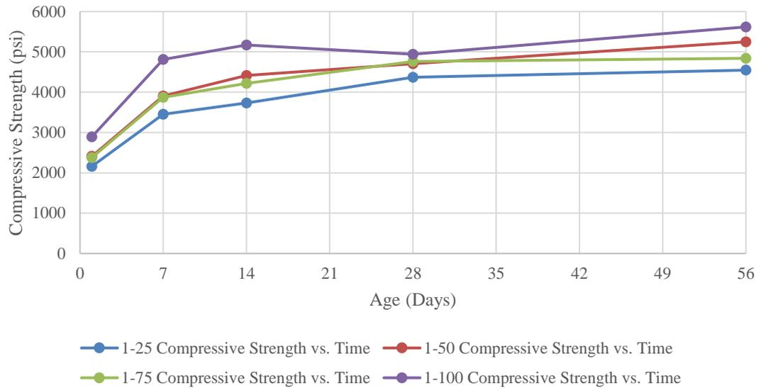
**Figure 4.11 Compressive Strength vs. Time Plot for Series No. 1**
