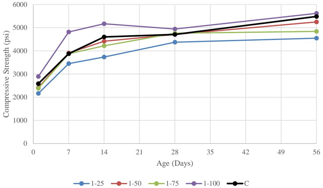
**Figure 4.21 Series No. 1 & Control Compressive Strength vs. Time**
