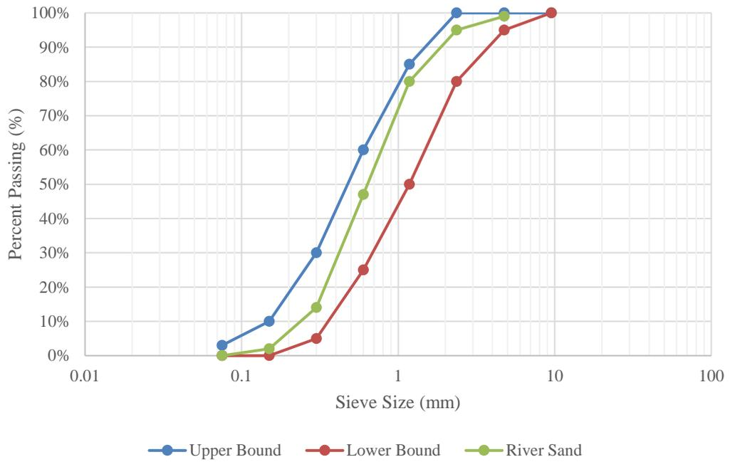
**Figure 3.4 River Sand Gradation with ODOT Boundaries**
