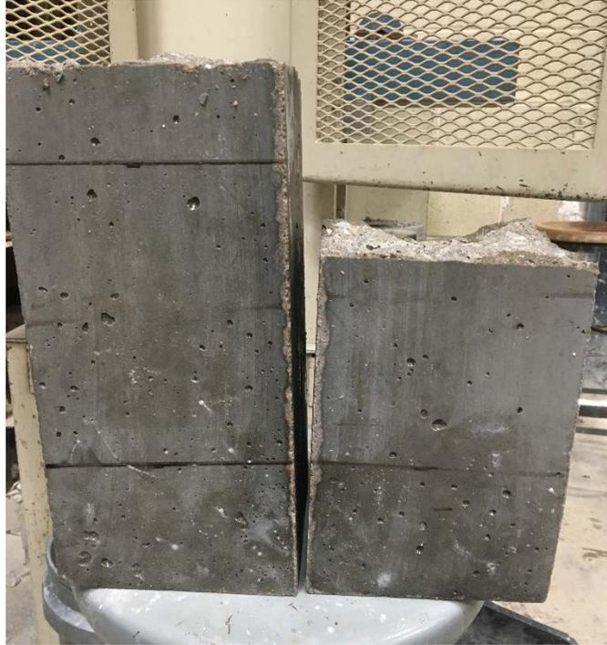
*Figure 4.4 Control MOR Beam After Loading*
