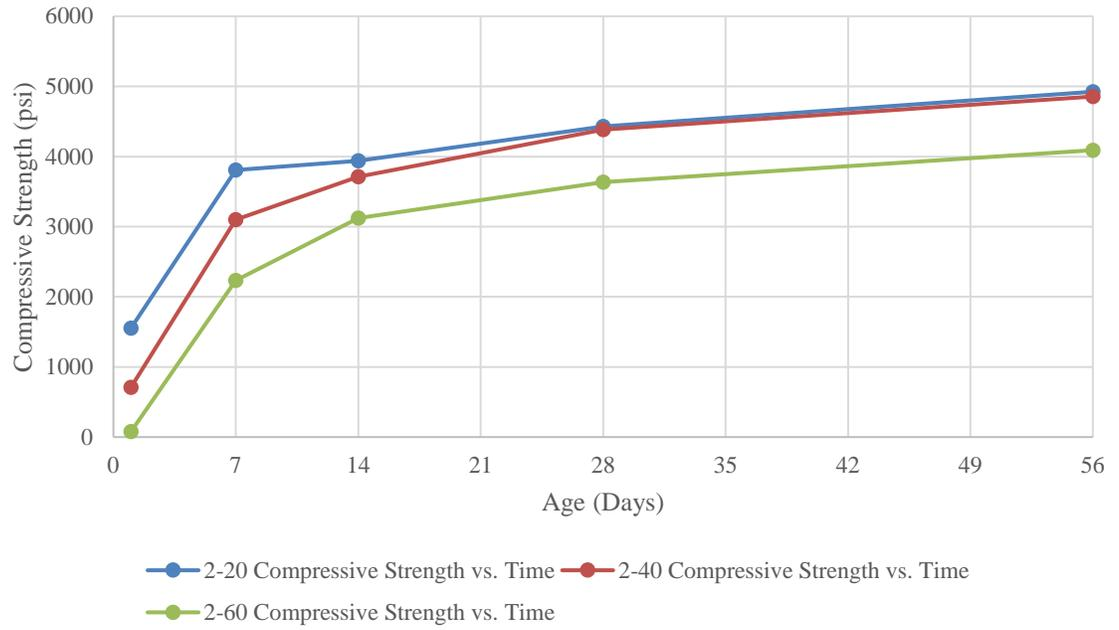
**Figure 4.17 Compressive Strength vs. Time Plot for Series No. 2**
