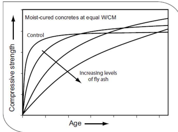
**Figure 2.5 Compressive Strength of Fly Ash Concrete vs. Age (Thomas, 1987)**
