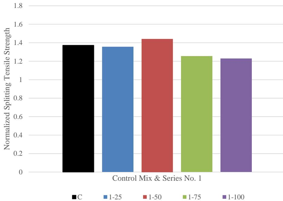
**Figure 4.30 Normalized Splitting Tensile Strength for Series No. 1 & Control**
