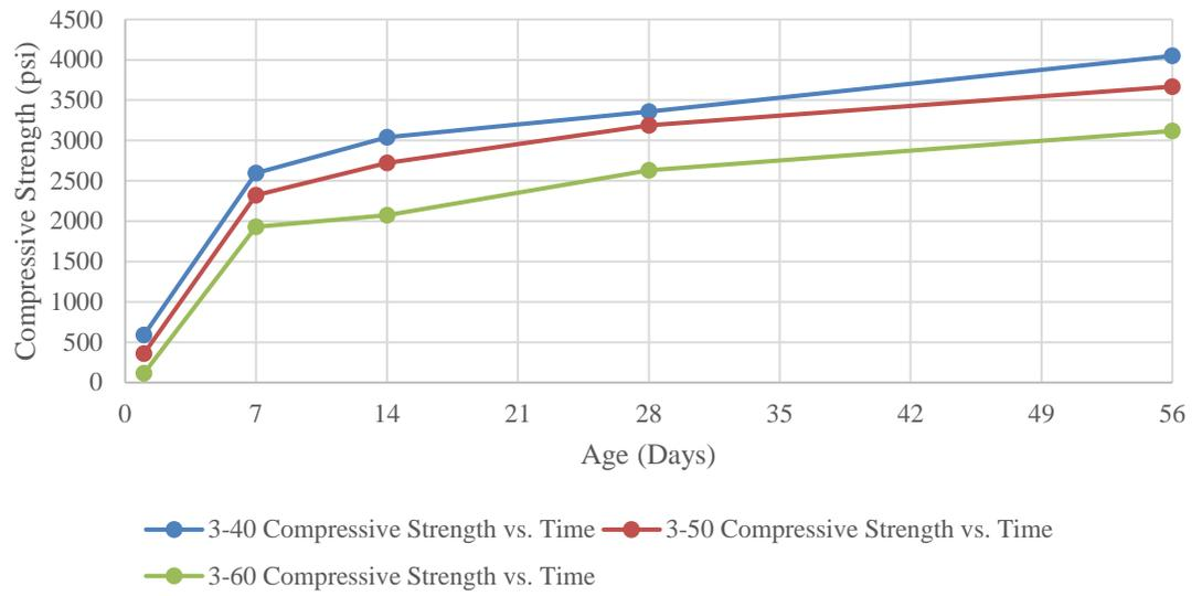
**Figure 4.19 Compressive Strength vs. Time Plot for Series No. 3**
