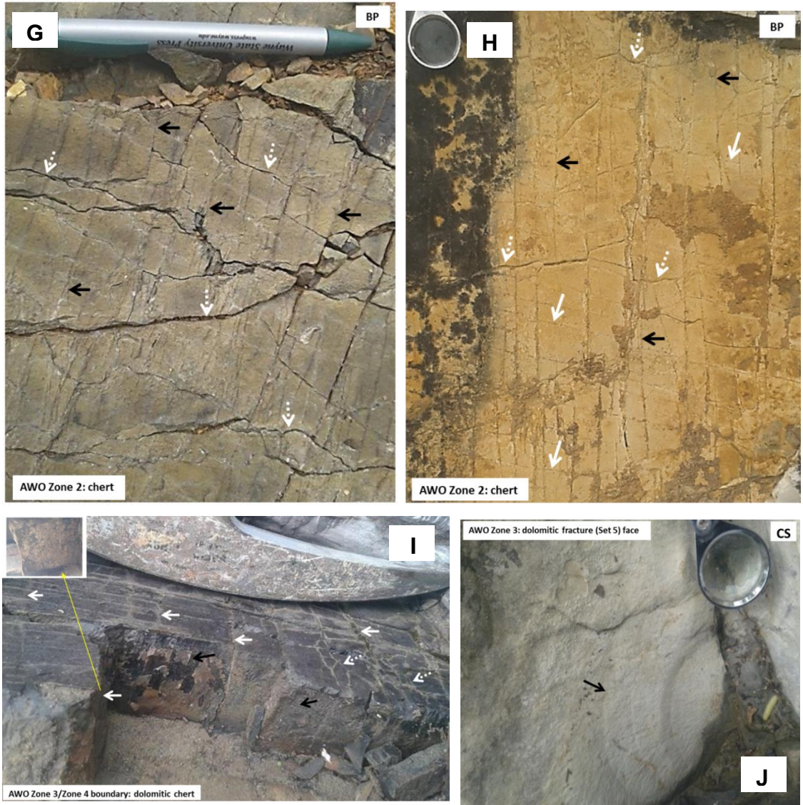
Figure 3.5: Fracture (joint) sets in the US-77D and AWO. Fractures are identified on the outcrop with arrows drawn sub-perpendicular to their traces. Some fractures are indicated by both arrows and lines drawn directly above the fractures for easier identification. A) US-77D wall ( 34^{\circ}26'38.6''\text{N} , 97^{\circ}07'40.6''\text{W} ) from the lower Woodford Shale showing the different fracture sets. Set 4 fractures are not shown in this photograph due to their small sizes. B) Carbonaceous, argillaceous mudstones (more ductile) with Set 2 fractures that are generally absent in the brittle beds. Notice that Set 4 fractures are non-systematic and shorter compared to the other sets. C) Set 2 fractures with substantial right-lateral displacement and gouge. Opening bends are circled. D) Remnant cake of a ductile mudstone bed on a chert bed. Note that Set 2 fractures present on the mudstone are oriented about 35-40 degrees counterclockwise (as seen in the photograph of the overturned beds) to the Set 5 fractures in the chert beds. E) Massive ductile mudstone beds dominated by Set 2 and Set 4 fractures. F) Dolomitic beds showing crosscutting between Set 1 and Set 5 fractures. G) Heavily quartz cemented Set 5 fractures and non-systematic Set 4 fractures. H) Narrow, systematic,
