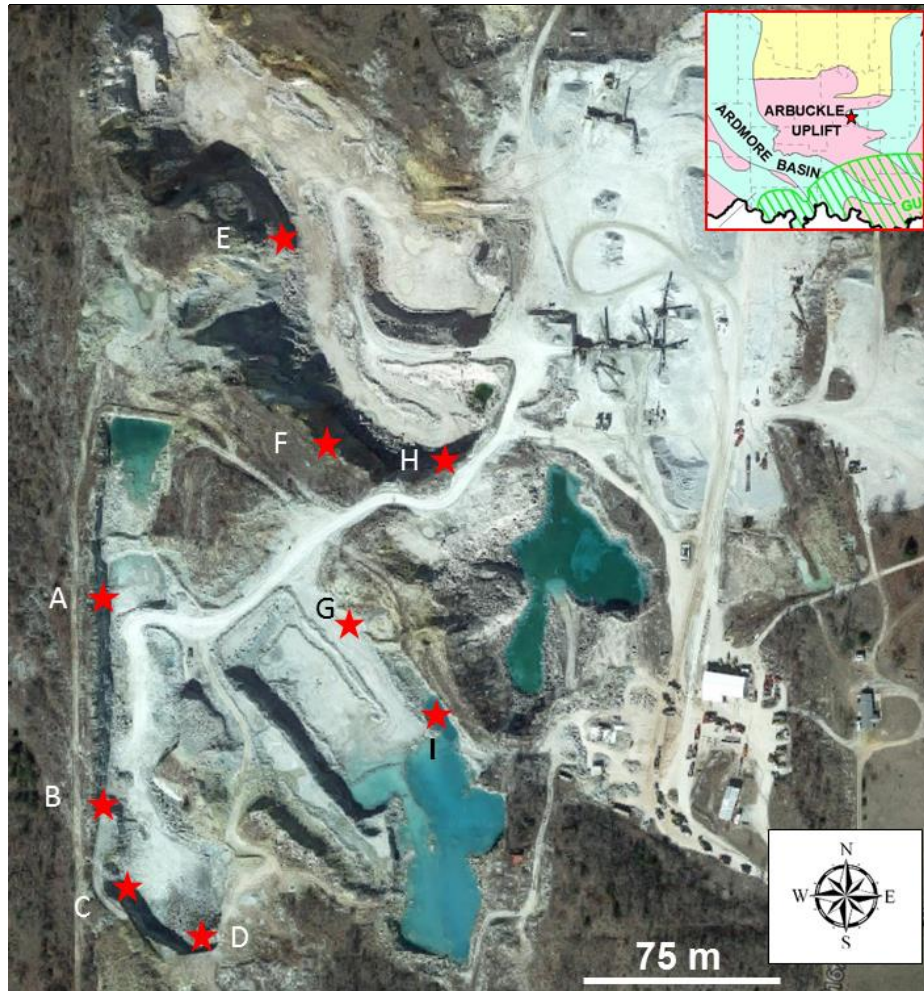
Figure 1.5: Plan view of the Jennings Quarry (34°35'39.3"N, 96°39'01.2"W). The beds dip 5-15 degrees towards the NE direction at the measured spots. The west and south sides have well-exposed faces for fracture length and height measurements. In addition, locations such as Spot G and Spot I (dry during measurement) have quarry floor fracture exposures for aperture measurements.
