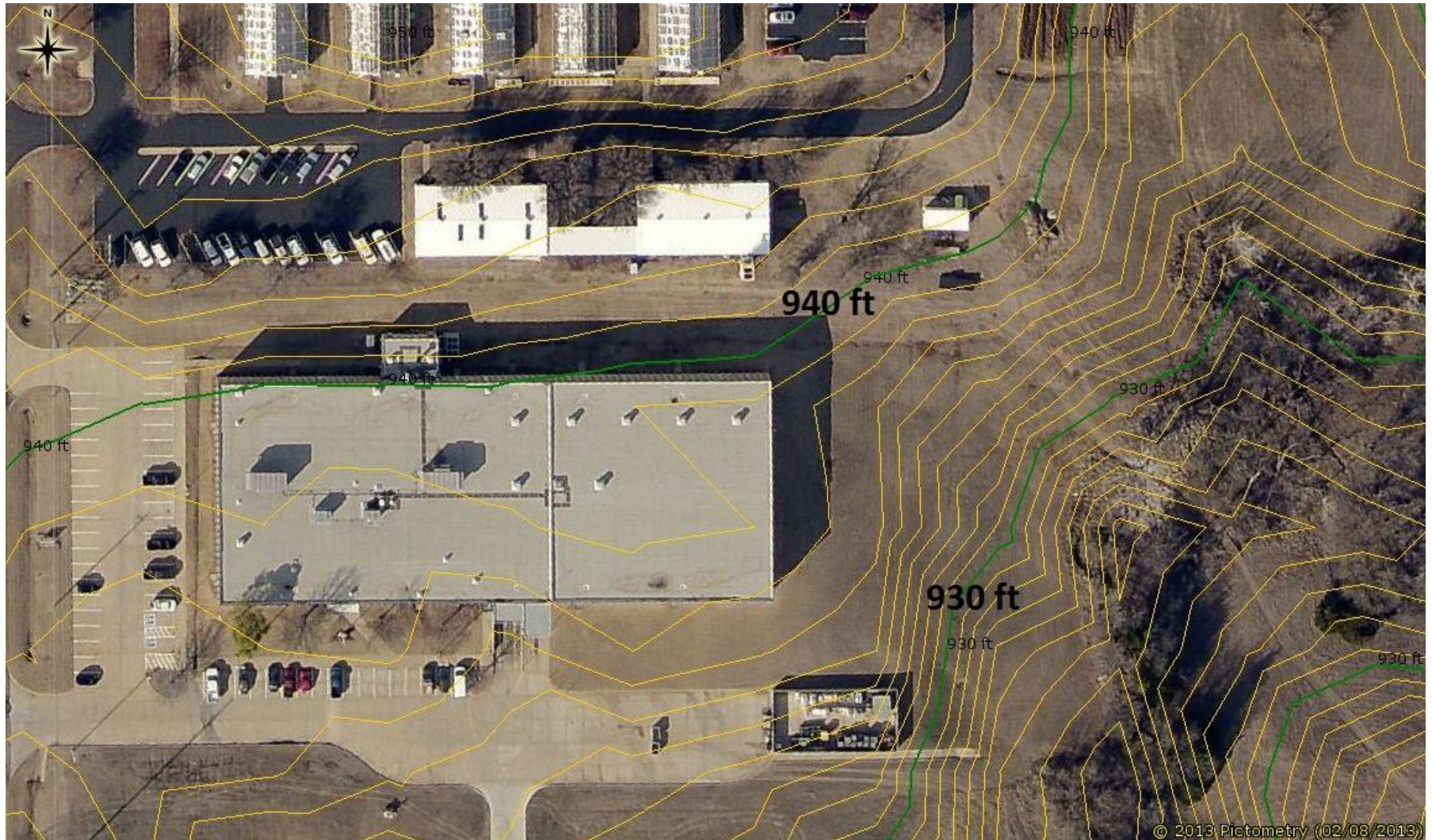
Figure D-1. Topographic Map of USDA-ARS. The Environmental and Warehouse Buildings are seen in white and the runoff will be transported down gradient of these buildings.
