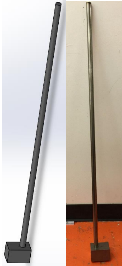
Figure 102: Solidworks model for hammer (left) and final machined hammer (right)
