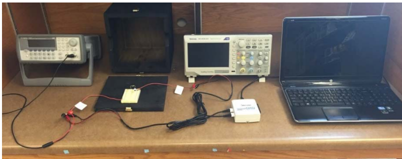
Figure 16: Electrical System - RC circuit
