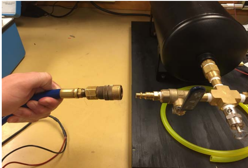
Figure 72: Charging the Tank with Air
