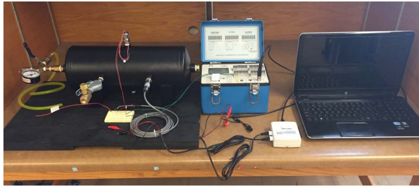
Figure 18: Fluid/Thermal System - Blowdown Tank
