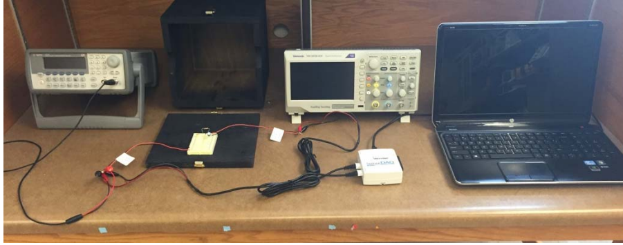
Figure 1: Electrical System-RC Circuit
