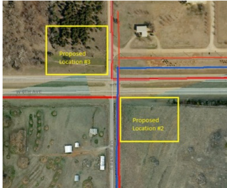
Figure 4.1-3: Alternatives #2 and #3 for our pump location site. Alternative #2 was chosen as our official site, and alternative #3 was rejected due to poor existing grading on the site.
