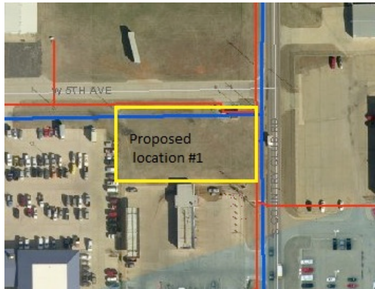
Figure 4.1-2: Alternative #1 for our pump location site. This alternative was rejected because it was deemed too cluttered with existing buildings and utilities.
