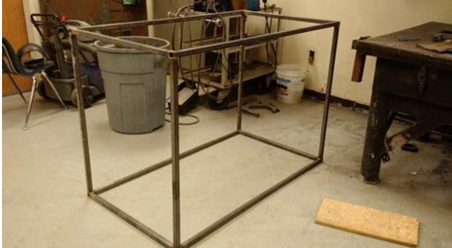
Figure 1 – Fabricated half-scale model of skid frame.
