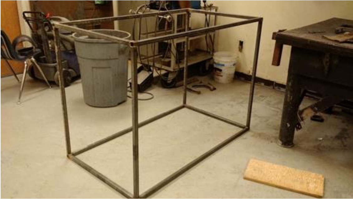
Figure 6 – Image shows actual fabricated skid model located at DML. Straight welds and dimensions match that of models shown in the previous figure.
