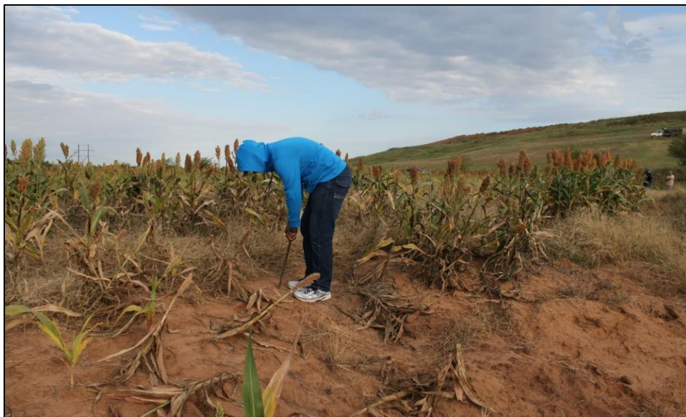
Figure 6: Sampling the cover topsoil
