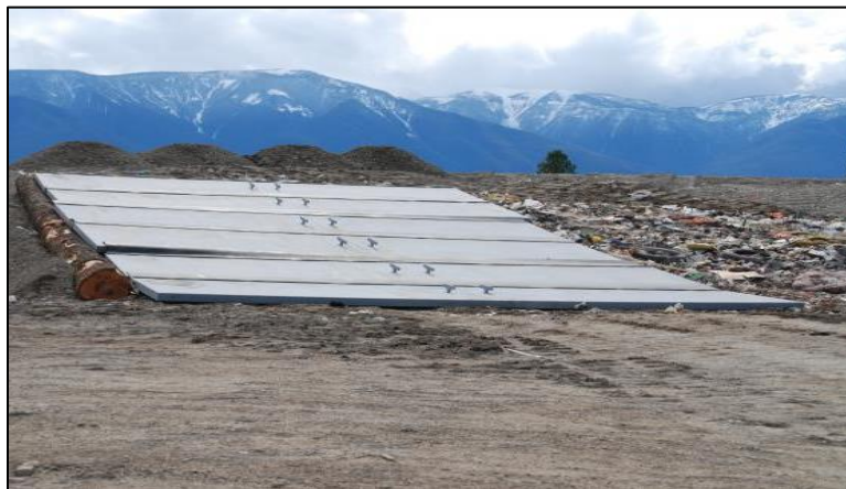
Figure 12: Landfill steel plates (Solid Waste Association of North America, 2015)
